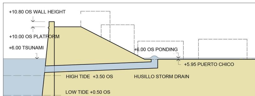
**Figure 8.** Schematic profile of Puerto Chico square and flooding of this neighbourhood through the storm drain.
