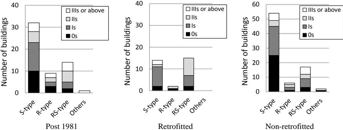
Figure 5.2. Damage rank of the column base
