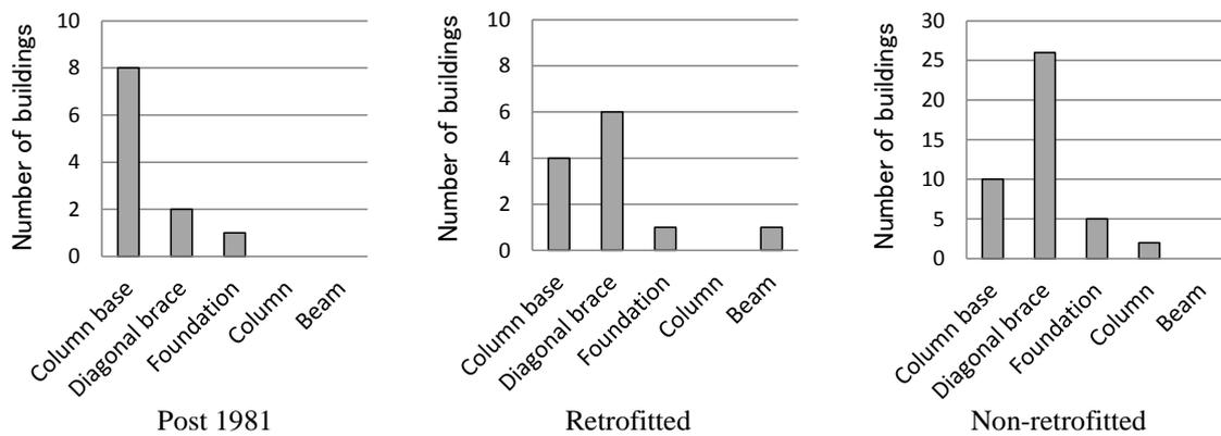
**Figure 3.5.** Structural components whose damage rank was IVs or Vs of buildings with “major damage”
