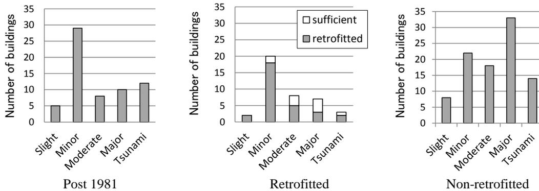
**Figure 3.4.** Damage rank of the buildings
