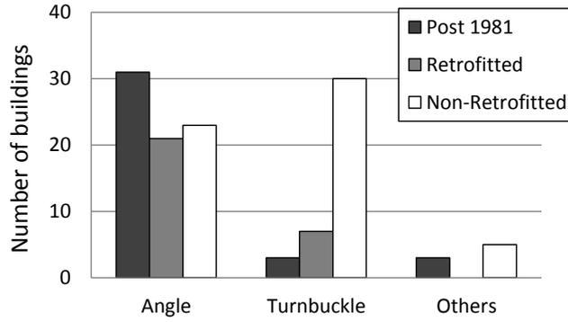
**Figure 4.1.** Section shapes used in the diagonal braces
