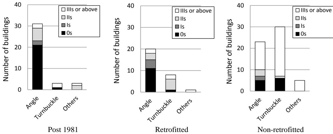
**Figure 4.2.** Damage rank of the diagonal braces
