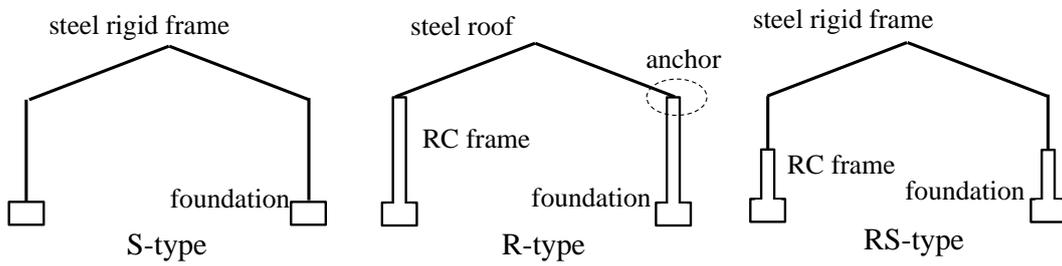
**Figure 3.2.** Structural frame in the Y-direction
