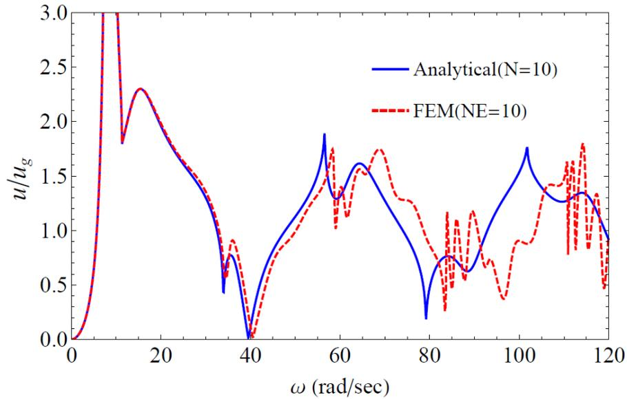
**Figure 4.** FEM vs. Analytical displacement of the beam crest
