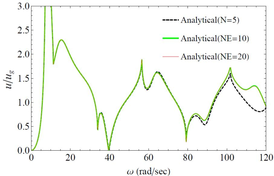
**Figure 3.** Analytical FRF of the beam crest for different number of series terms considered
