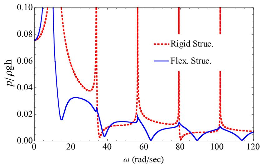
**Figure 7.** FRF of pressure at base level for rigid and flexible cases of Structure
