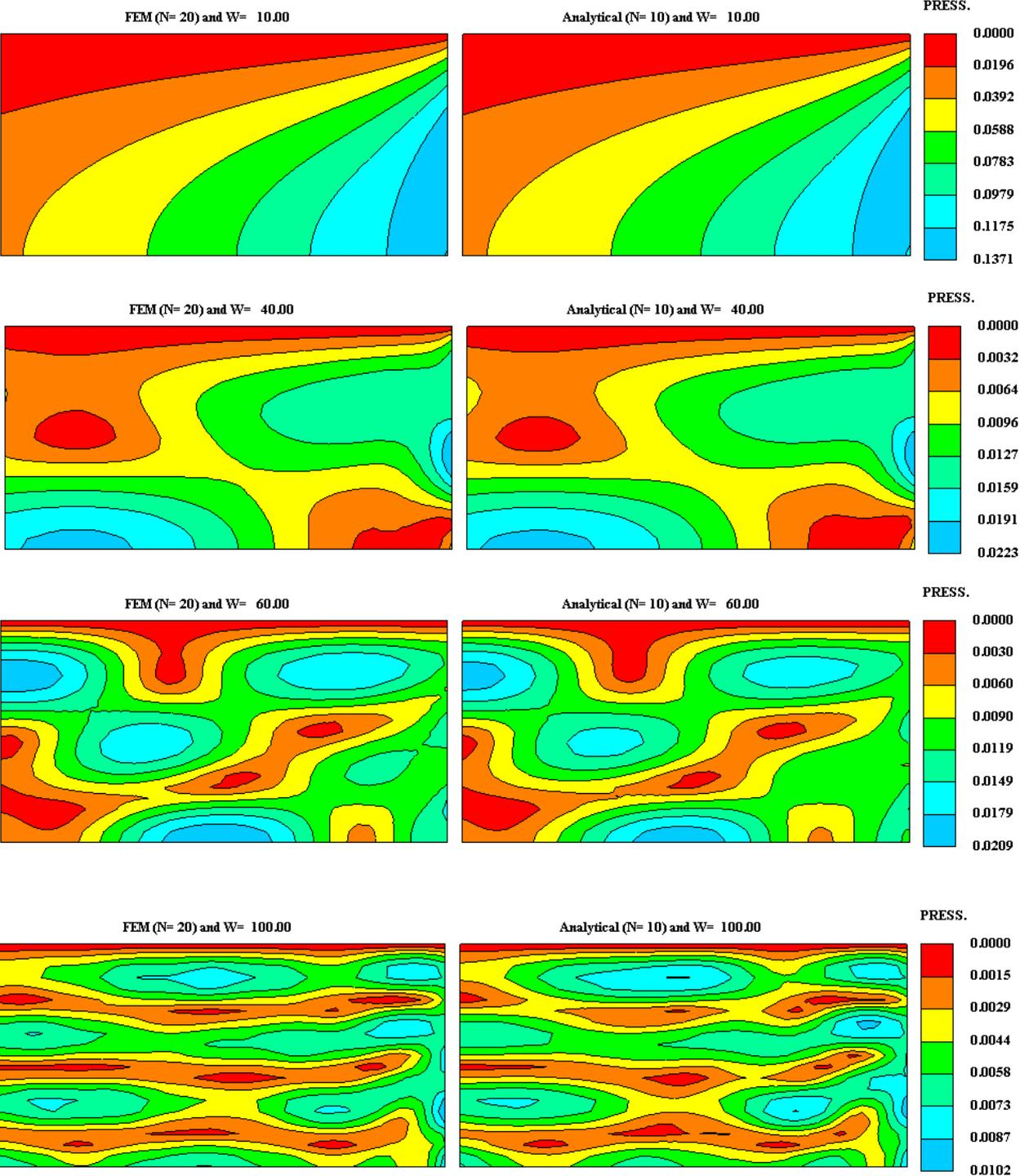
Figure 10. Pressure distribution of FEM vs. Analytical results for various  $\omega$
