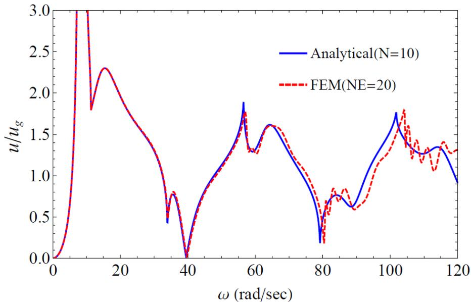
**Figure 5.** FEM vs. Analytical displacement of the beam crest
