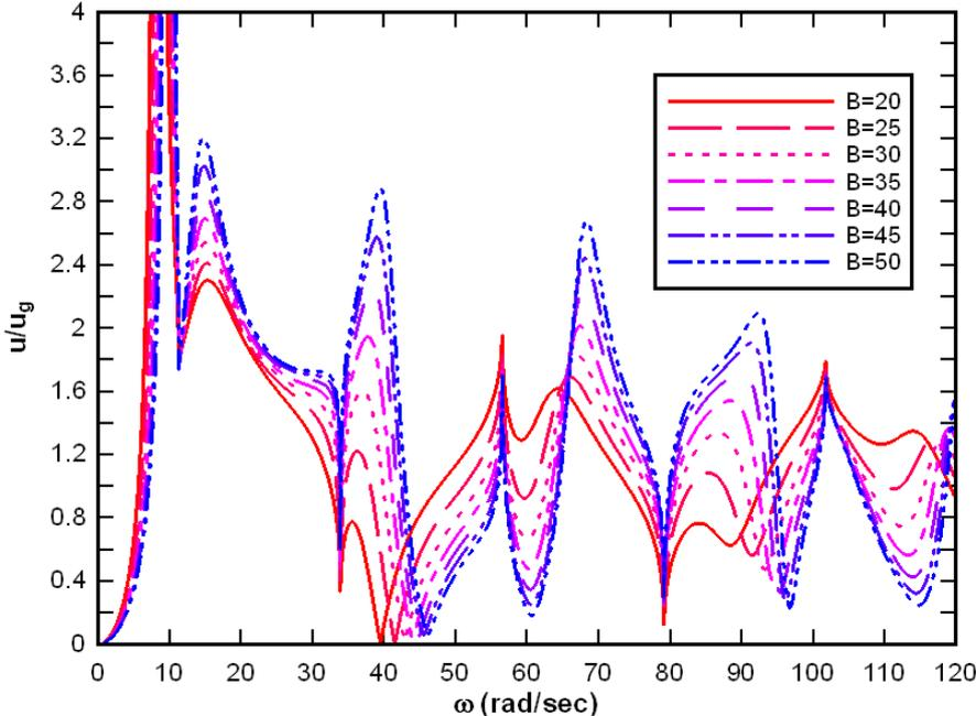
**Figure 9.** FRF of displacements at beam crest for various widths of beam
