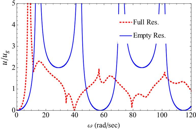
**Figure 8.** FRF of beam crest for full vs. empty reservoir cases
