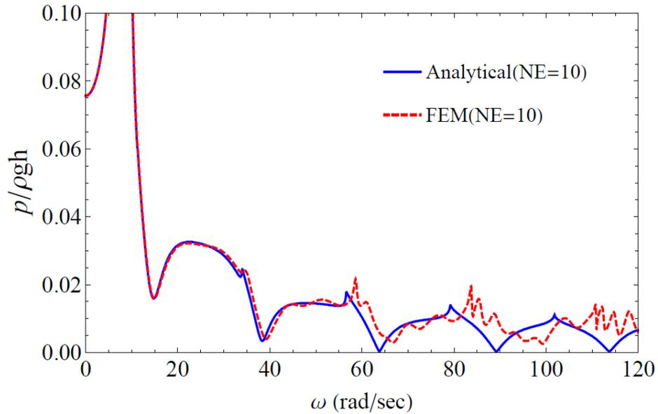
**Figure 6.** Pressure frequency response function at base level
