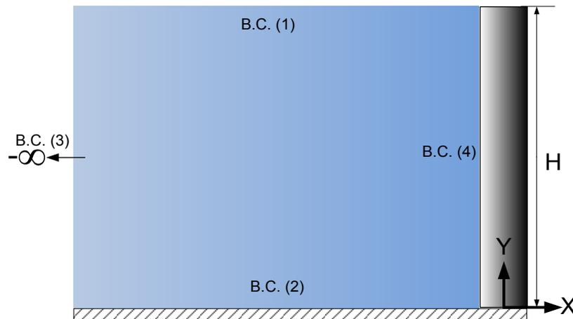
**Figure 1.** Fluid-structure system and fluid boundary conditions
