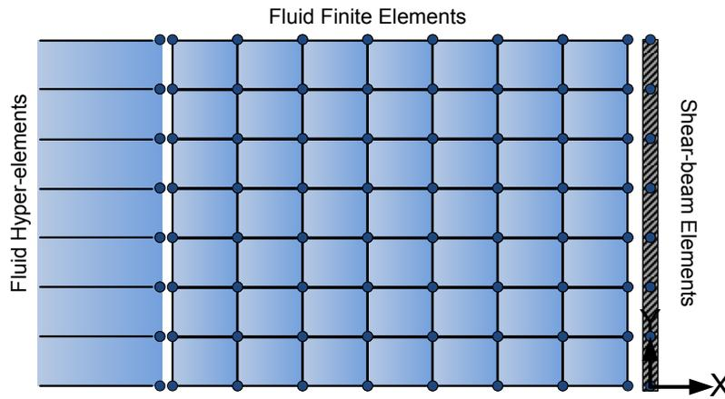
**Figure 2.** A schematic finite element mesh for the beam and reservoir
