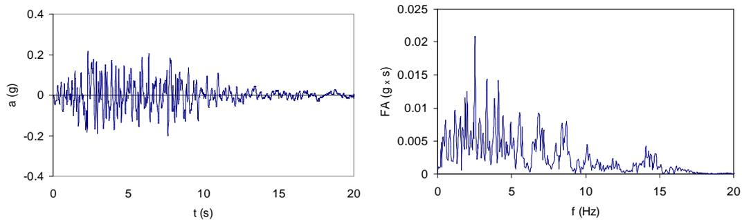
**Figure 7.** Time history and Fourier amplitude of the horizontal input accelerogram (NTC)
