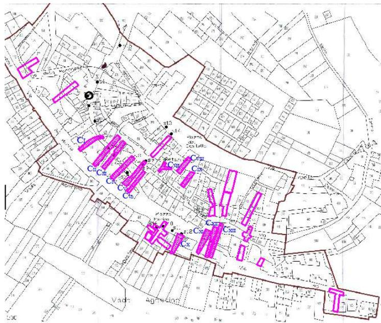
**Figure 5.** Plan location of the main cavities detected in the centre of Castelnuovo
