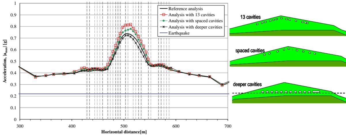
**Figure 10.** Peak acceleration along the free surface of the hill: effect of horizontal spacing among cavities and of cavity depth below the hill surface
