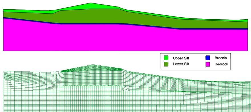
**Figure 6.** Model geometry with material identification (top); finite element mesh (bottom)
