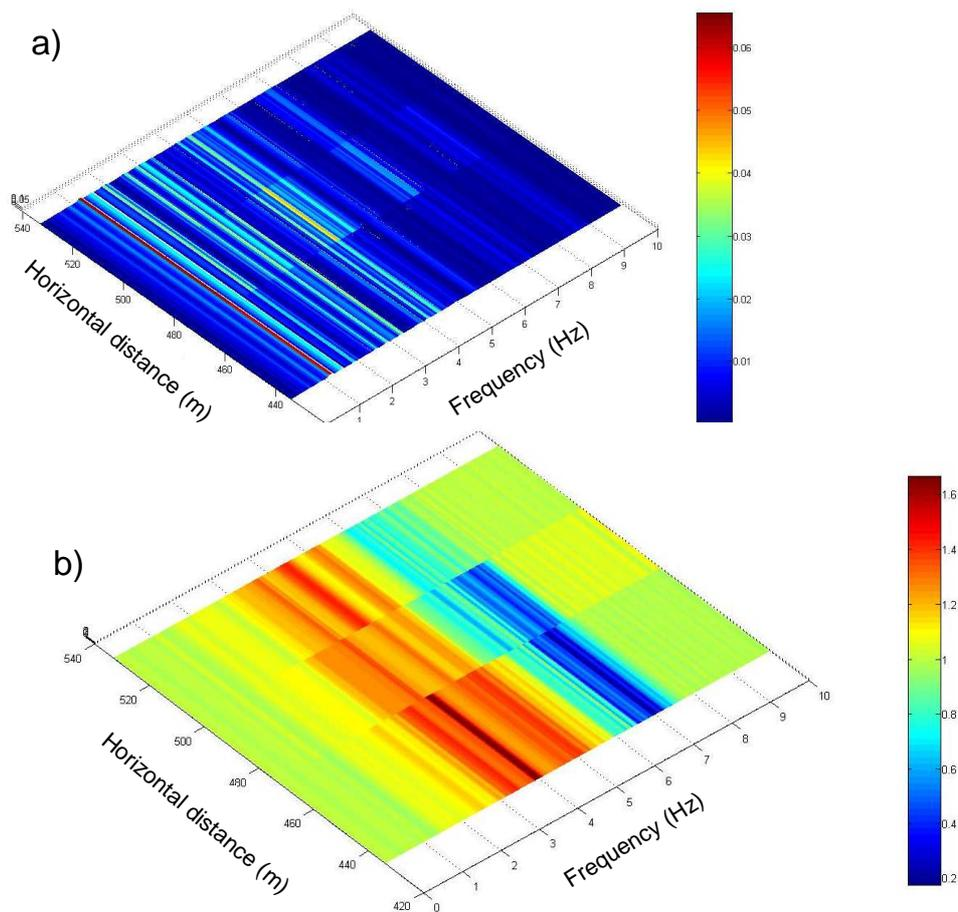
**Figure 12.** In (a) acceleration Fourier amplitude along the top of the hill for the reference analysis (no cavities); in (b) transfer function between the surface accelerations computed from the analysis with 13 cavities and from the reference analysis (no cavities)
