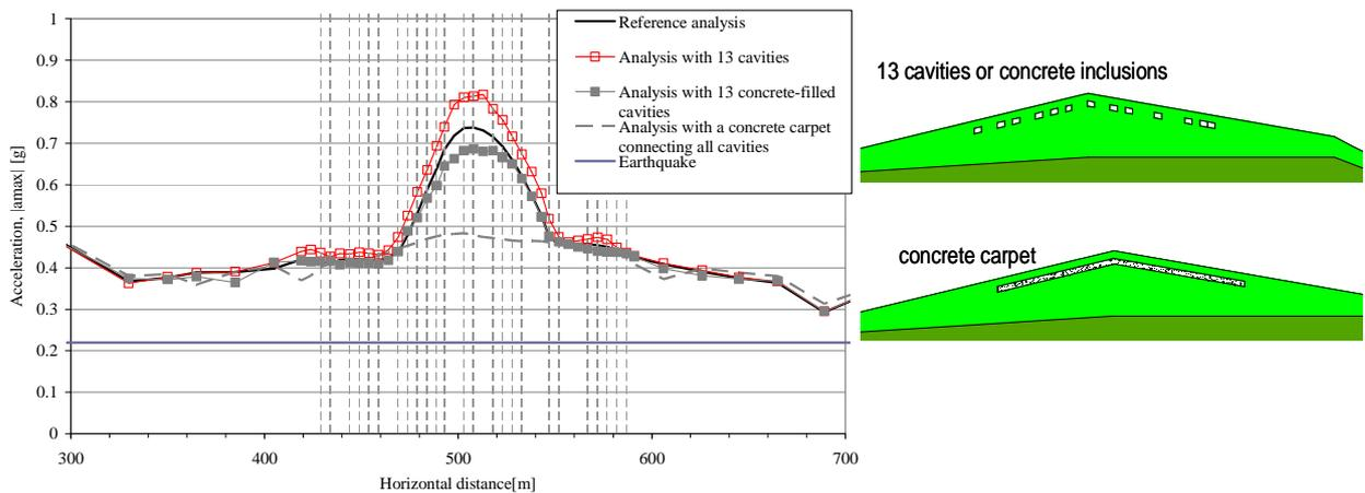
**Figure 11.** Peak acceleration along the free surface of the hill: effect of cavities, concrete inclusions and of a continuous concrete carpet
