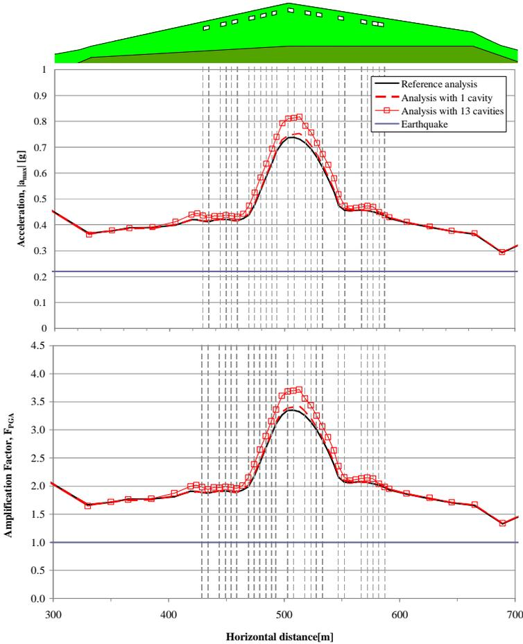
**Figure 9.** Peak acceleration (top) and PGA amplification factor (bottom) along the free surface of the hill
