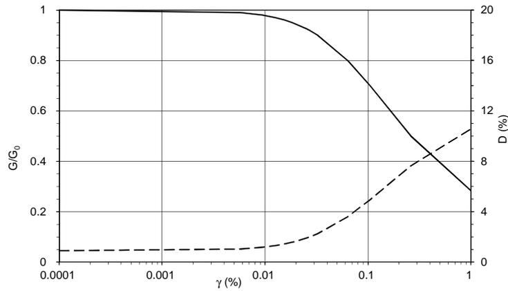
**Figure 4.** Experimental nonlinear behaviour of the white silt (L) present in the subsoil of Castelnuovo
