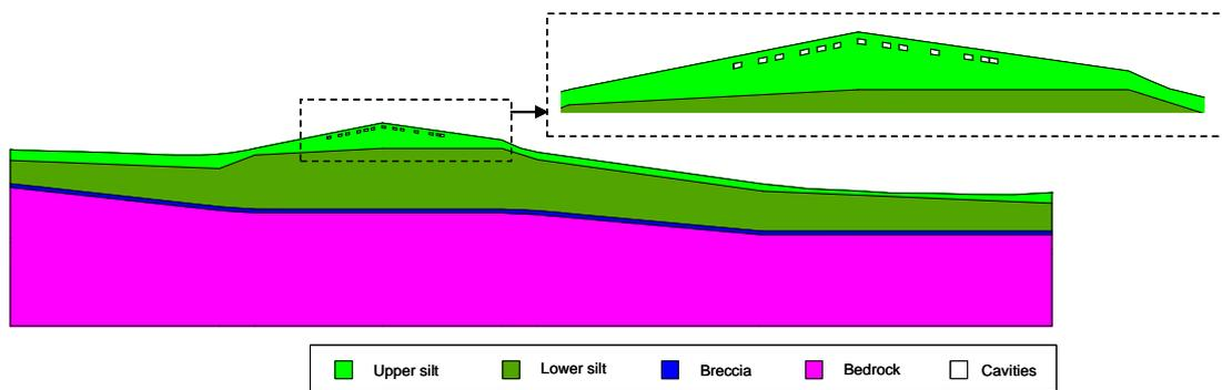
**Figure 8.** Location of cavities in the numerical model with a zoom at the top of the hill
