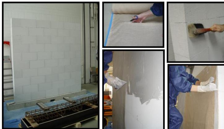
**Figure 10.** Reinforcement of masonry wall with jute fibre mats
