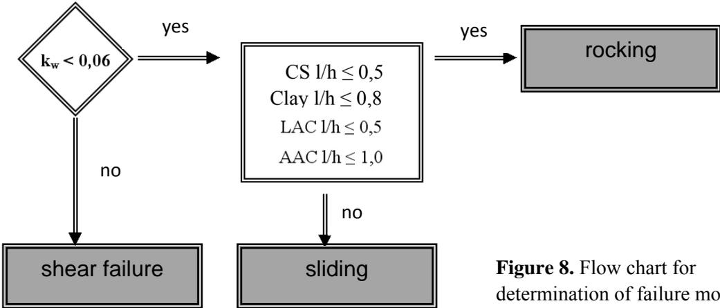
Figure 8. Flow chart for determination of failure mode
