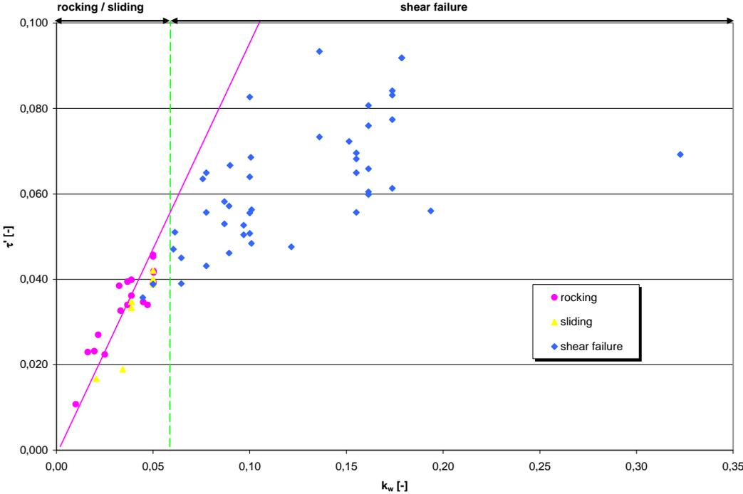
Figure 7. Nondimensional representation of lateral force capacity versus wall coefficient
