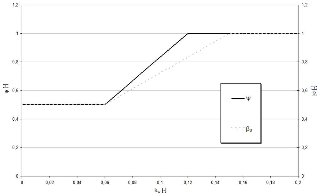
**Figure 5.** Dependency of fixture degree  $\psi$  and coefficient of clamping efficiency  $\beta_0$  from wall coefficient  $k_w$
