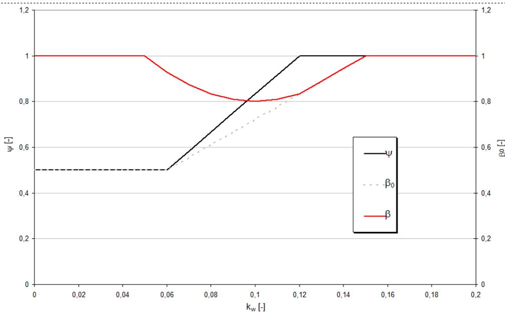
**Figure 6.** Correction factor  $\beta$  versus wall coefficient  $k_w$
