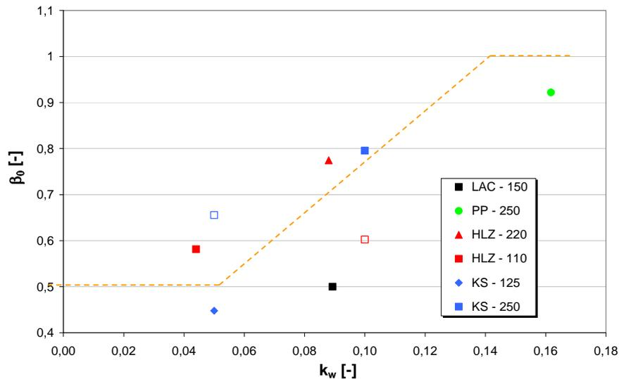
**Figure 4.** Influence of wall coefficient  $k_w$  on the coefficient of clamping efficiency  $\beta_0$
