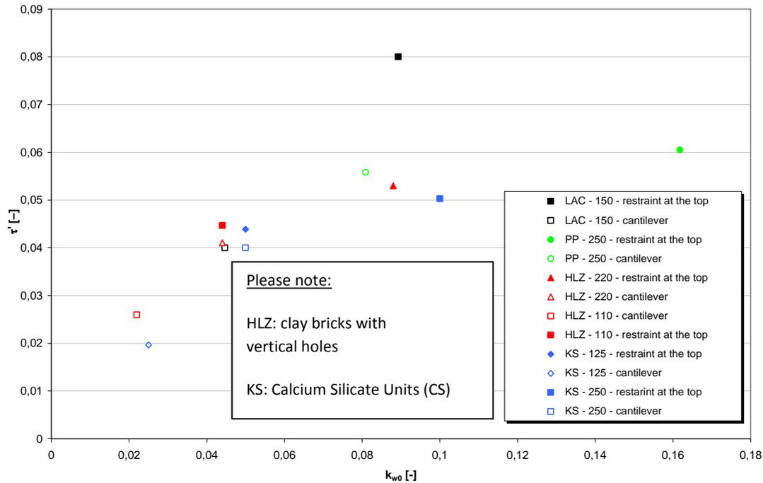
**Figure 3.** Influence of moment fixture (clamping) on the non-dimensional shear capacity
