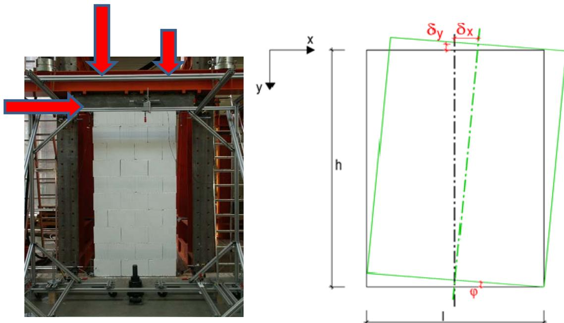
**Figure 1.** Rotational movement of a wall by an angle  $\varphi$
