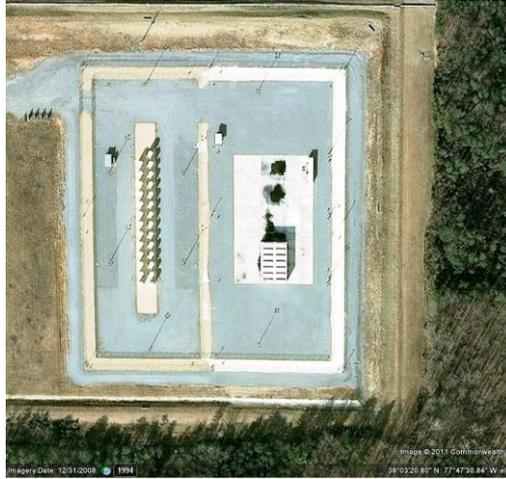
**Figure 2.** Dry casks placed vertically in robust above-ground concrete at North Anna nuclear power plant site [10]
