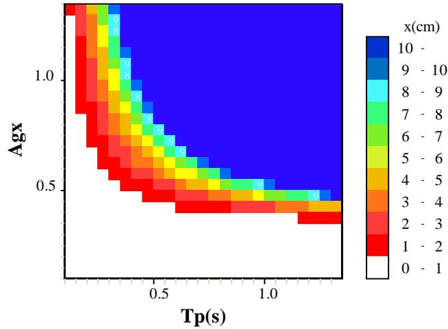
**Figure 4.** Predicted displacement in cm (color scale indicated) as a function of predominant period of shaking,  $T_p$ , and peak acceleration,  $A_{gxg}$ , for a  $\mu$  value of 0.3. Red swath indicates values that predict maximum displacement values of 1-2 cm, the target displacement to estimate  $A_{gxeqg}$  with a 90% probability of nonexceedance.
