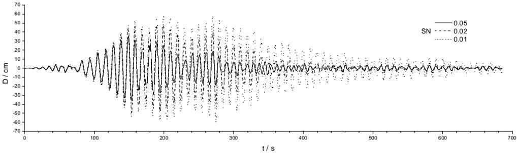
**Figure 7** Structural response displacement time histories(SN)
