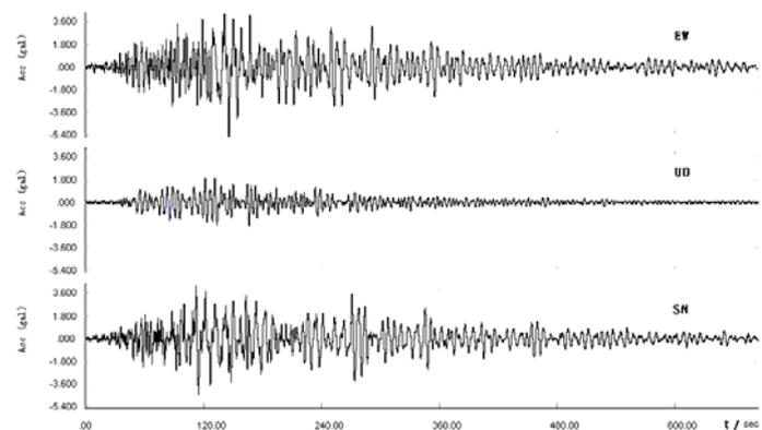
Figure 2 Main earthquake ground motion records of A050 station in Jiangsu province
