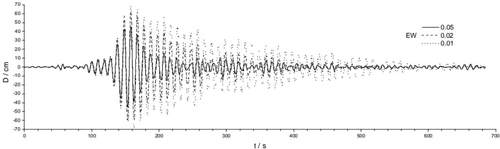
**Figure 8** Structural response displacement time histories(EW)
