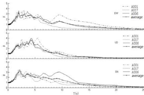
**Figure 3** Acceleration response spectra of bedrock site
