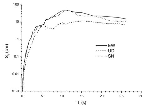
**Figure 6** Displacement response spectra of ground motion records (A050, damping ratio: 0.05)
