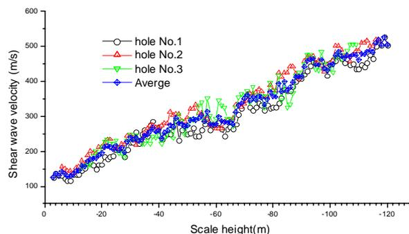
**Figure 5** Shear wave velocities of soil layers
