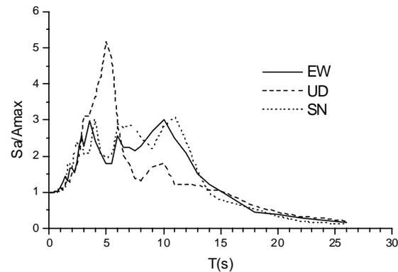
**Figure 4** Acceleration response spectra of ground motion records (A050 station, damping ratio: 0.05)
