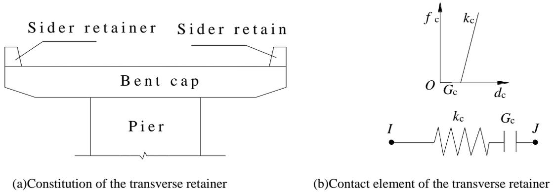
**Figure 3.** The transverse restrainer
