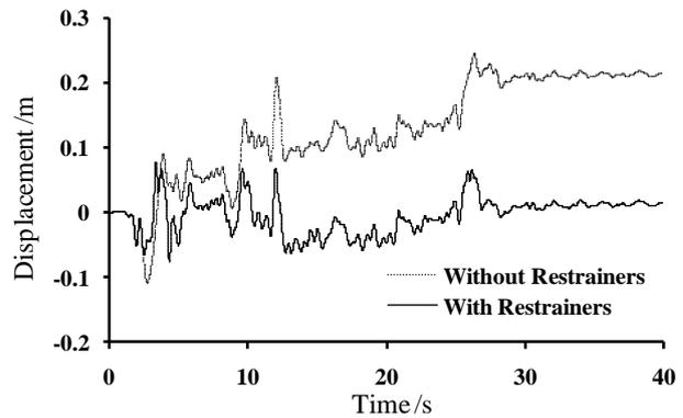
**Figure 5.** Time-history of the transverse relative displacement of pier-girder at Pier 2 under El Centro wave (PGA is 0.2g)
