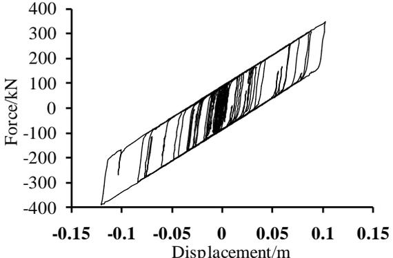
**Figure 11.** Hysteretic curve of LRB at Pier 1 under transverse-vertical El Centro wave (PGA is 0.4g)
