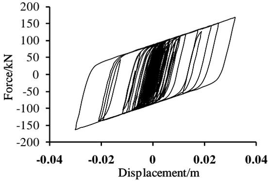
**Figure 10.** Hysteretic curve of LRB at Pier 1 under longitudinal-vertical El Centro wave (PGA is 0.4g)
