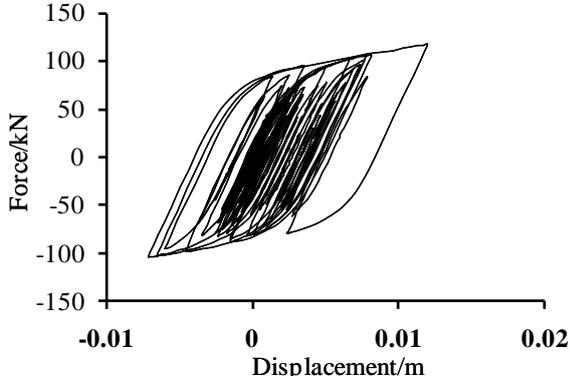
**Figure 8.** Hysteretic curve of LRB at Pier 1 under longitudinal-vertical El Centro wave (PGA is 0.2g)
