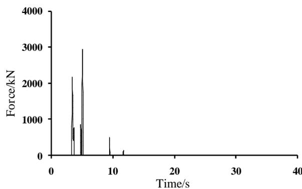
**Figure 6.** The time-history of the tension of the left restrainer at Pier 2 under the longitudinal-vertical El Centro wave (PGA is 0.2g)
