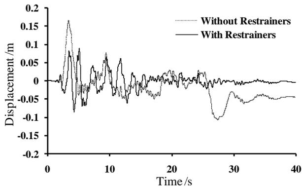
**Figure 4.** Time-history of the longitudinal relative displacement of pier-girder at Pier 2 under El Centro wave (PGA is 0.2g)
