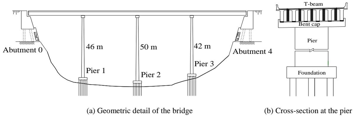
**Figure 1.** Skeleton diagram of HPCB
