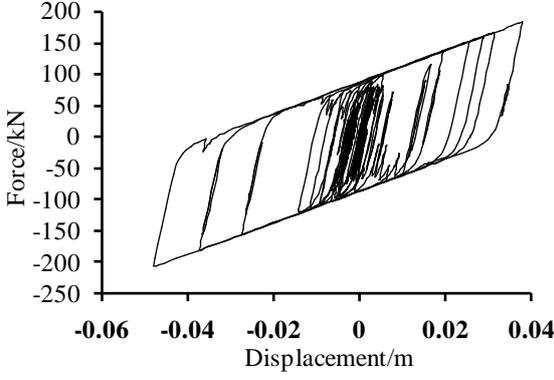
**Figure 9.** Hysteretic curve of LRB at Pier 1 under transverse-vertical El Centro wave (PGA is 0.2g)
