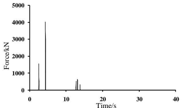
**Figure 7.** The time-history of pressure of the left restrainer at Pier 2 under the transverse-vertical El Centro wave (PGA 0.2g)
