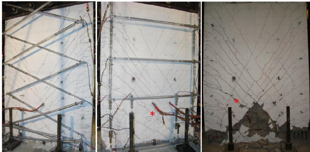
**Figure 7.** Crack patterns in specimen RW-A15-P10-S51 at drift ratios of 0.5%, 1.5%, and at failure
