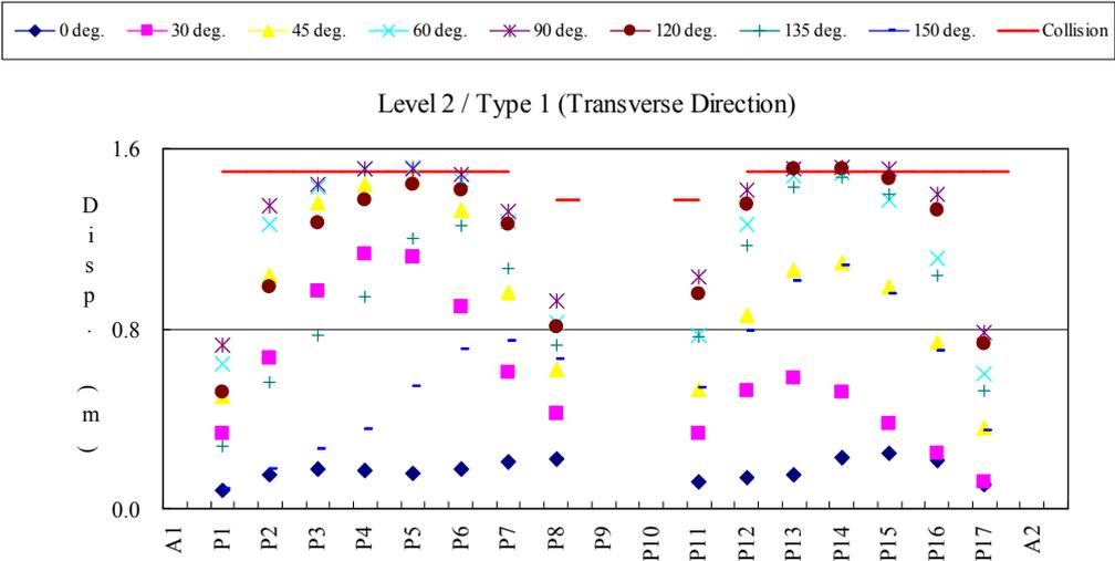
Figure 5.5 Displacement of slide bearings
