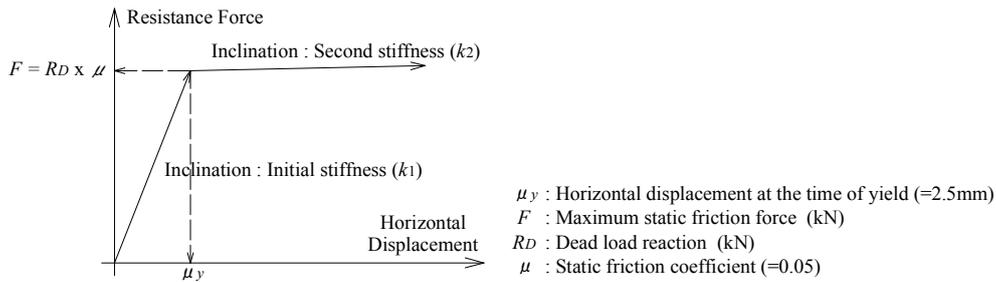
**Figure 5.2** Modeling for slide bearing
