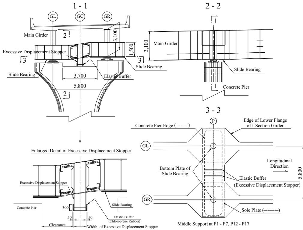
**Figure 3.2** Middle support of 2-I section girder and slide bearings
