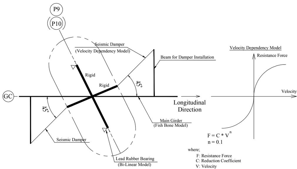
**Figure 5.3** Modeling for seismic damper
