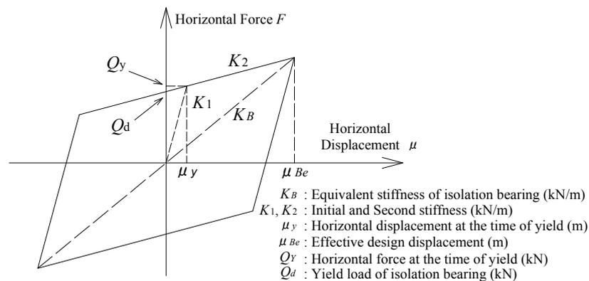
**Figure 5.1** Modeling for elastomeric bearing
