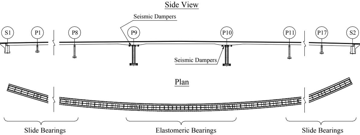
Figure 3.1 Device arrangement
