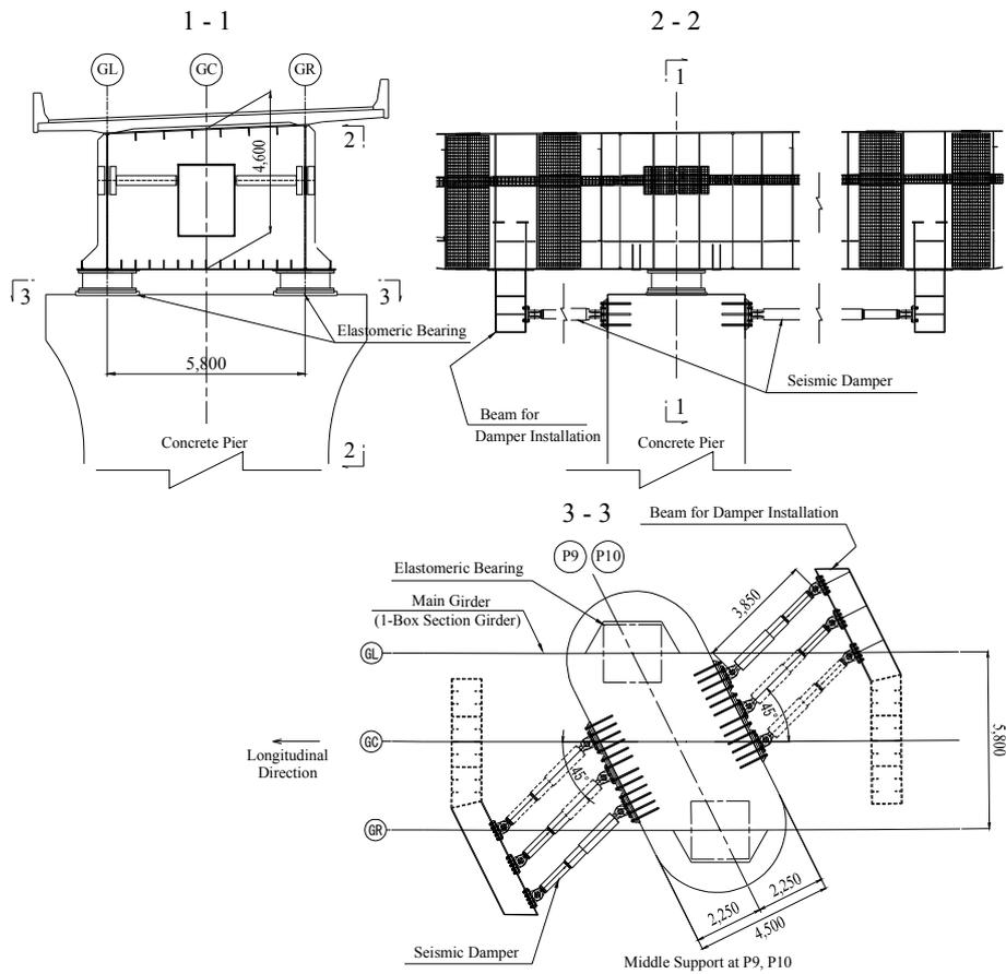
**Figure 3.3** Middle support of 1-box section girder installed the lead rubber bearings and seismic dampers
