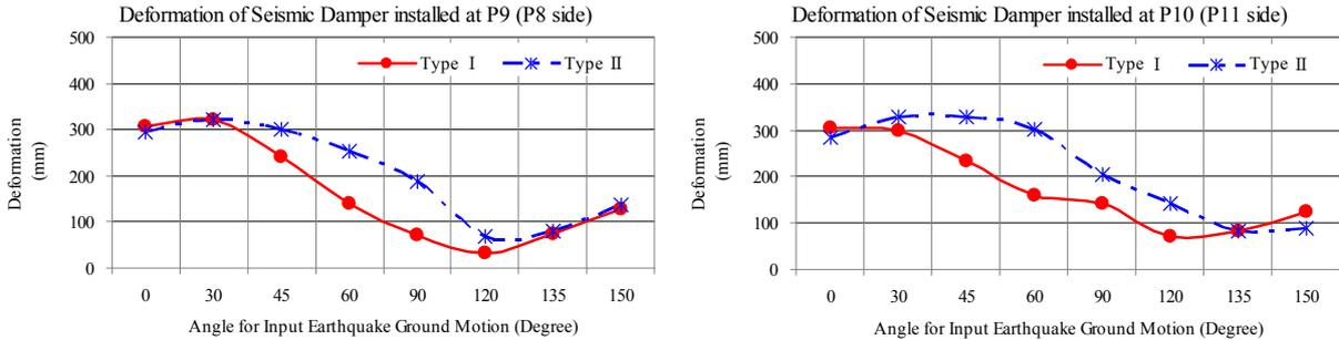
Figure 5.6 Deformation of seismic damper at Pier 9 and Pier 10
