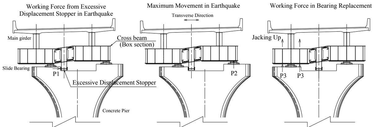
**Figure 6.2** Design force for cross beams with excessive displacement stopper
