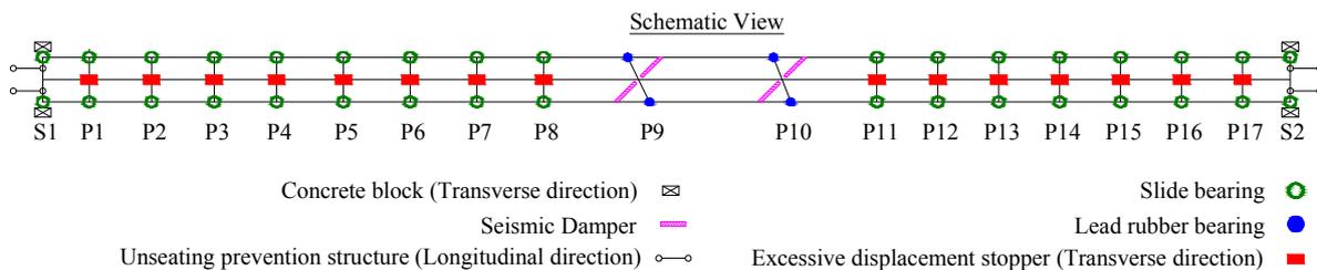
**Figure 4.1** Arrangement of unseating prevention system for Imagiregawa Bridge
