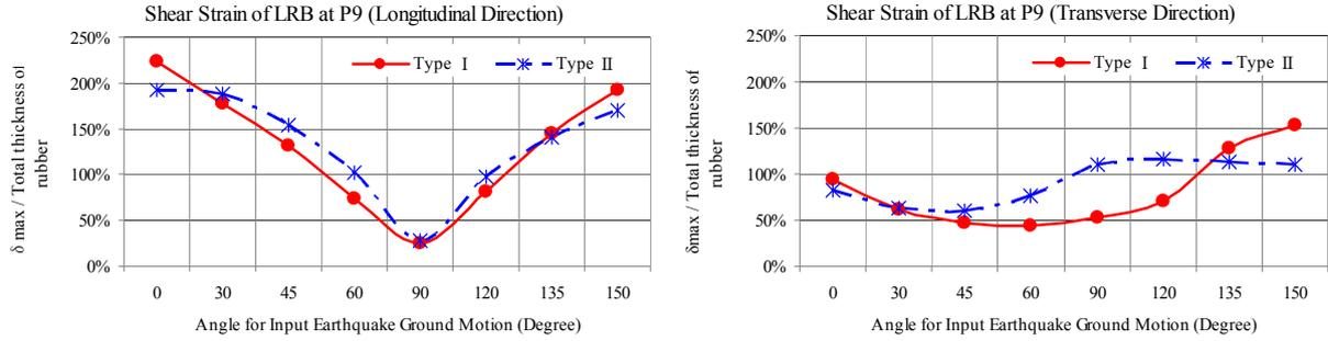
Figure 5.7 Shear strain of lead rubber bearing at Pier 9
