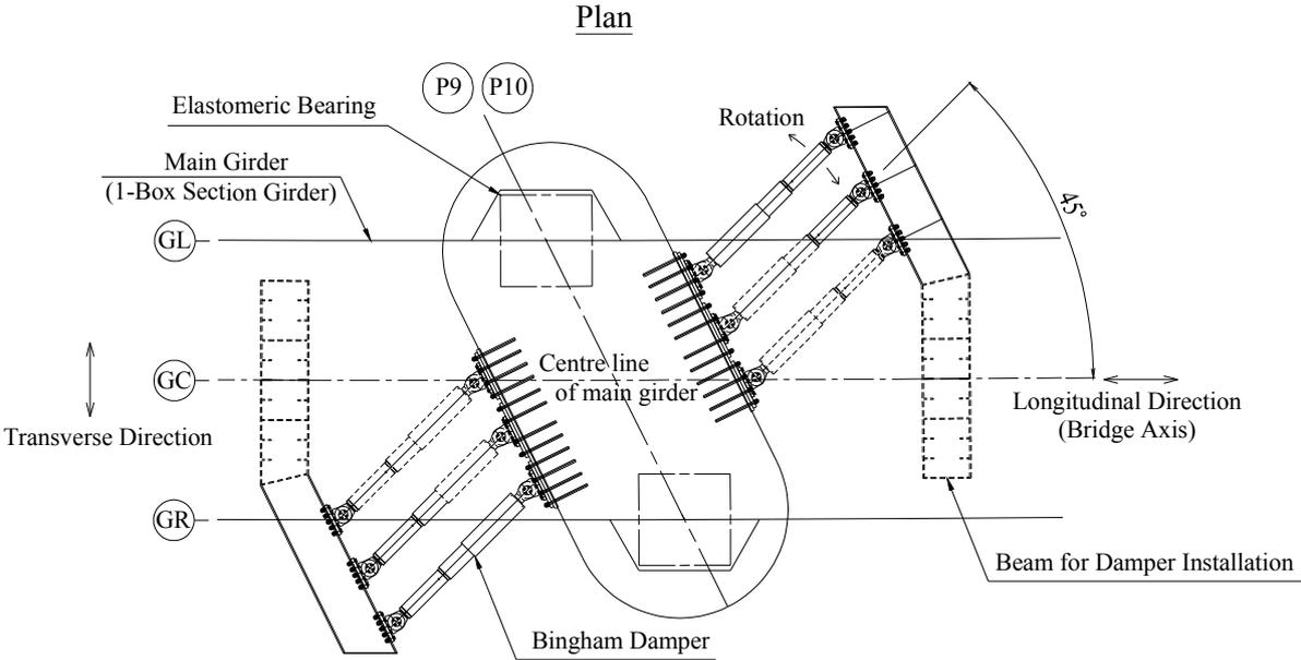
Figure 2.1 Installation angle of seismic damper
