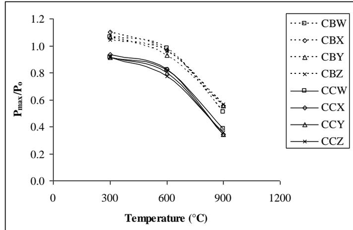
Figure 5. Variation of load ratio  $P_{\max}/P_0$  with temperature of pre-damaged confined column
