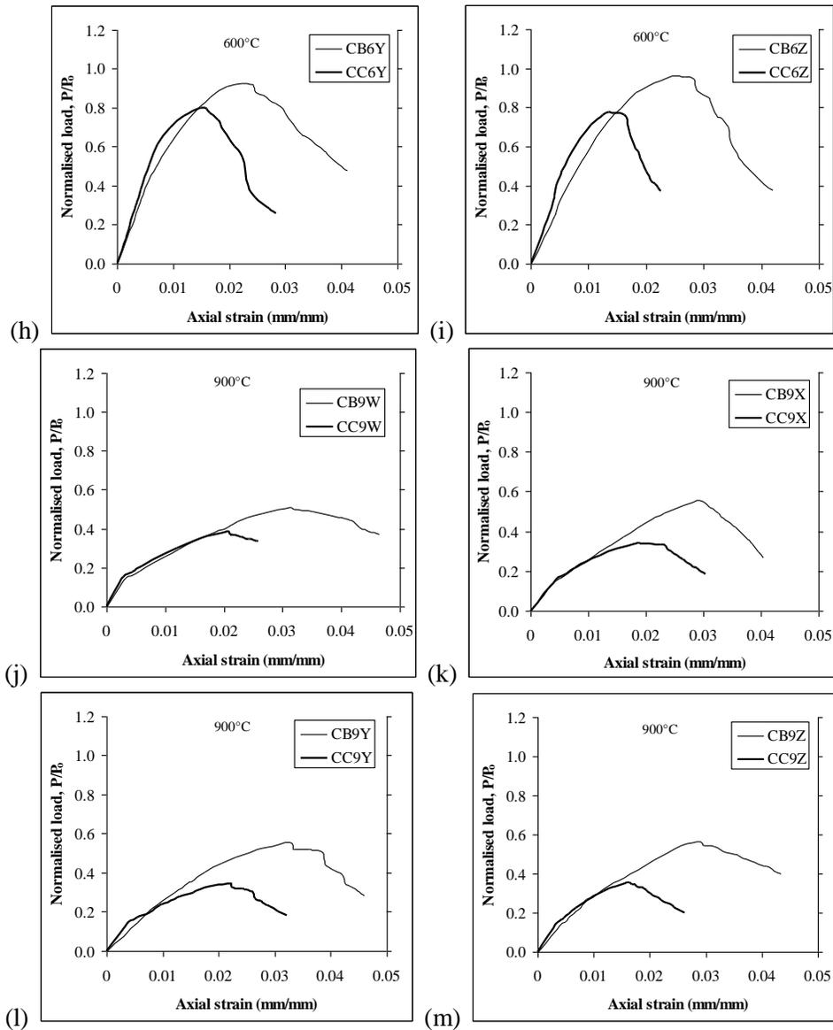
Figure 4. (h-m). Normalized applied load vs axial-strain for pre-damaged confined column (continued)
