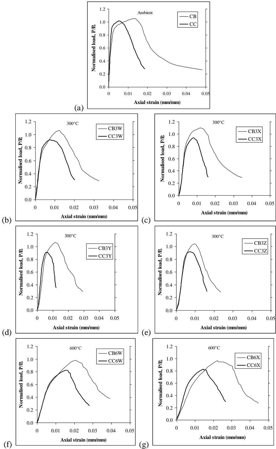
**Figure 4.** (a-g). Normalized applied load vs axial-strain for pre-damaged confined column (continues)
