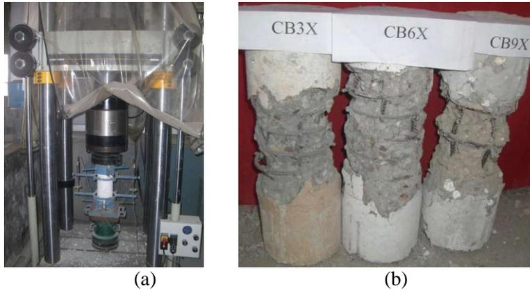
**Figure 2.** (a). Test set up with specimen in place (b) Appearance of CB tested specimens
