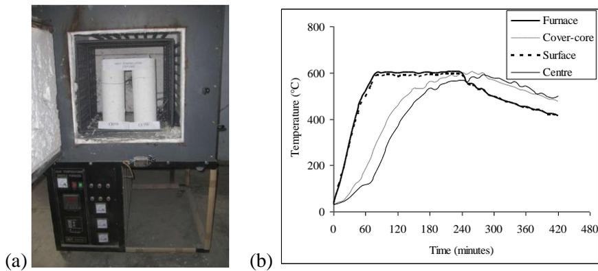
**Figure 3.** Temperature histories of CC6 series (a) Electric furnace (b) Time-temperature curves
