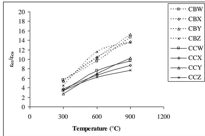
Figure 6. Variation of strain ratio  $\epsilon_{cc}/\epsilon_{cc0}$  with temperature of pre-damaged confined column
