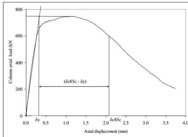
**Figure 1.** Initial damage determination for confined concrete
