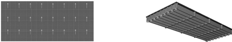
**Figure 2.1.** Analysis *5TBA*: plan (left) and axonometric (right) view of the finite element model
