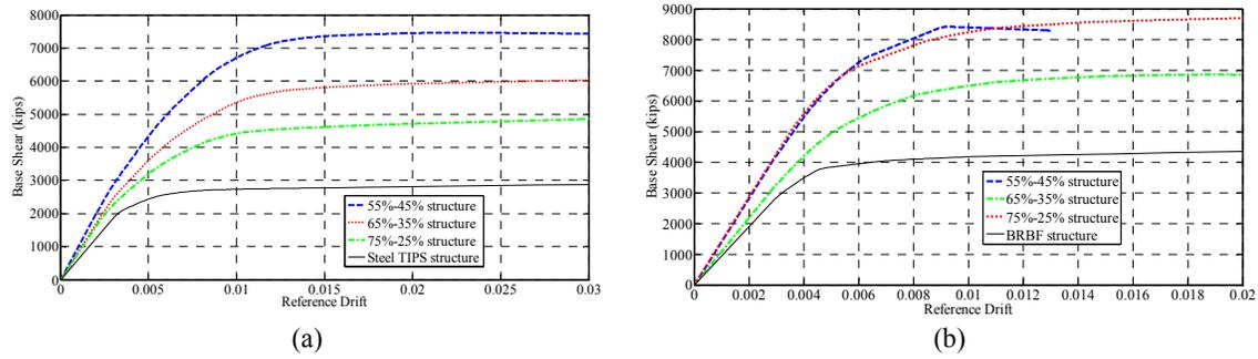
**Figure 4.** Pushover curves, (a) 7 story structures, (b) 12 story structures
