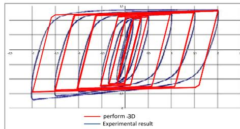
**Figure 2.** Result of calibrated parameters of PERFORM-3D
