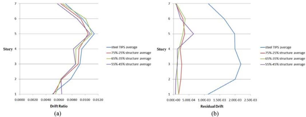
**Figure 8.** (a) Average max drift ratio vs. story, (b) Average residual drift vs. story; (7 story structures)
