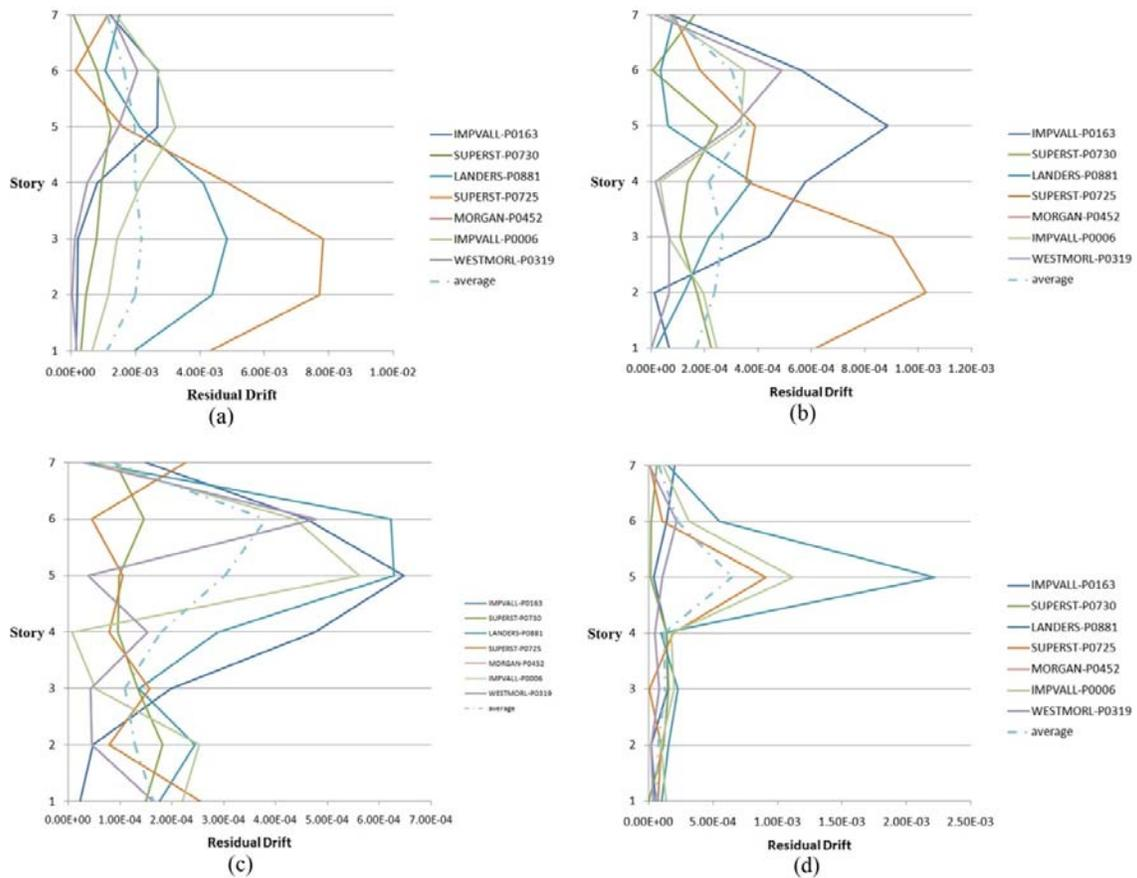
**Figure 7.** Residual drift vs. story; 7 story structures, (a) Steel TIPS structure, (b) 75%-25% structure, (c) 65%-35% structure, (d) 55%-45% structure
