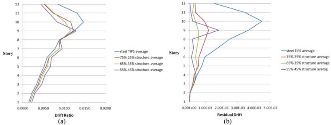
**Figure 10.** (a) Average max drift ratio vs. Story, (b) Average residual drift vs. story; (12 story structures)
