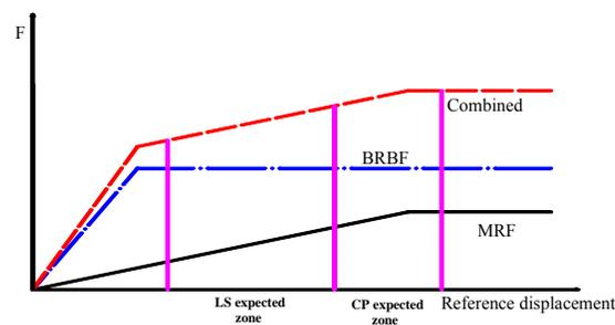
**Figure 1.** Force displacement response of the systems.
