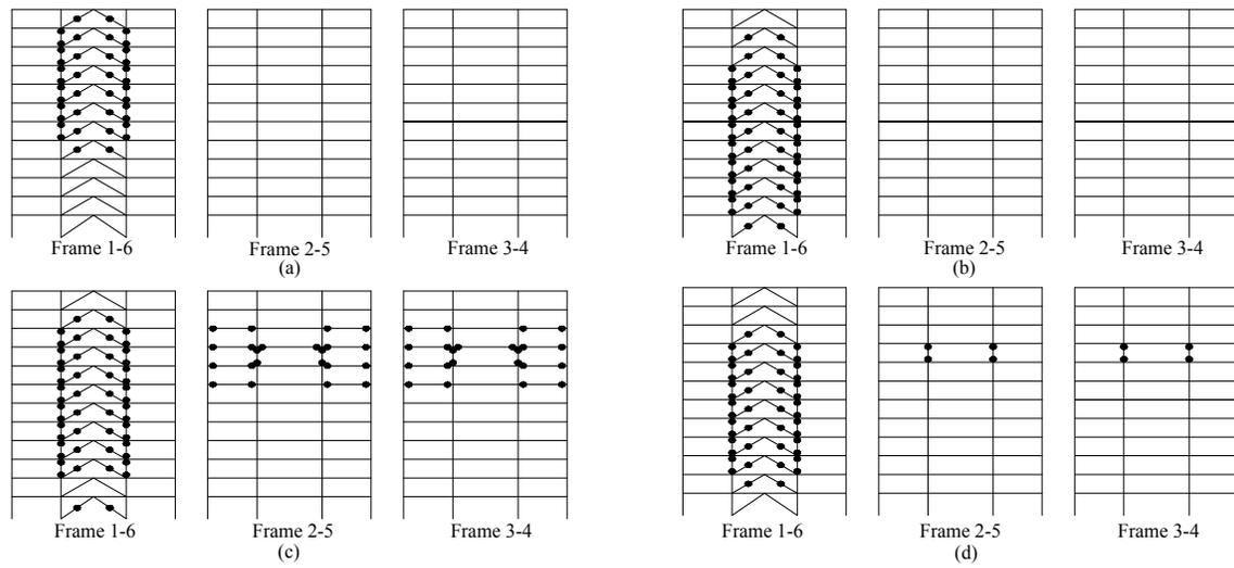
**Figure 6.** Plastic hinge formation at 12 story structures, (a) BRBF structure, (b) 75%-25% structure, (c) 65%-35% structure, (d) 55%-45% structure
