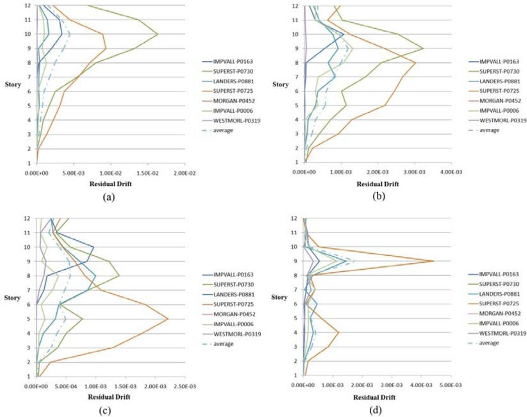
**Figure 9.** Residual drift vs. story; 12 story structures, (a) BRBF structure, (b) 75%-25% structure, (c) 65%-35% structure, (d) 55%-45% structure
