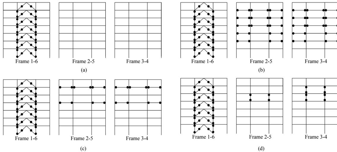
**Figure 5.** Plastic hinge formation at 7 story structures, (a) Steel TIPS structure, (b) 75%-25% structure, (c) 65%-35% structure, (d) 55%-45% structure
