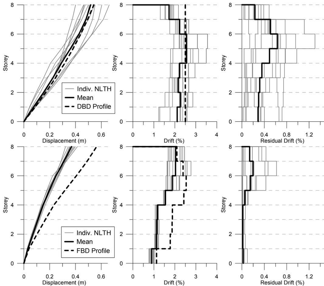
**Figure 5.2.** NTHA peak displacement (left panels), drift (central panels), and residual drift (right panels) results for DBD (upper panels) and FBD (lower panels) mixed systems at 100% of the design intensity
