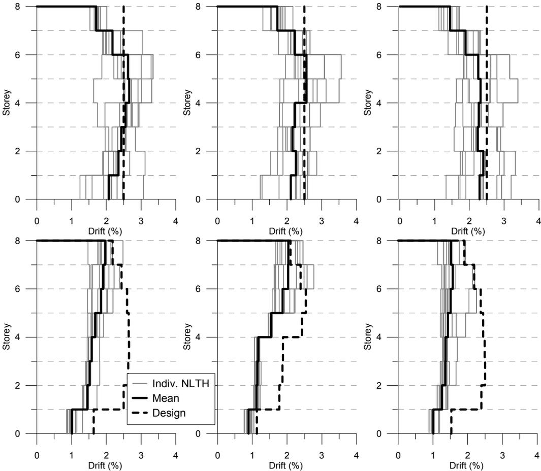
**Figure 5.1.** NTHA peak drift results for steel (left panels), mixed (central panels), and concrete (right panels) systems for DBD (upper panels) and FBD (lower panels) systems at 100% of the design intensity
