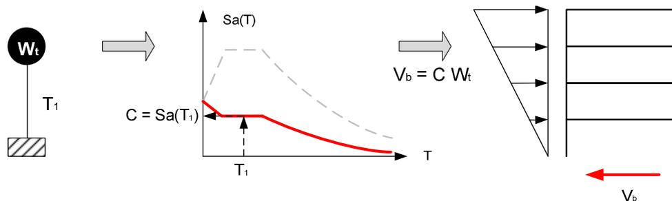
**Figure 3.1.** Outline of ASCE/SEI 7-10 ELF method based on the fundamental mode response
