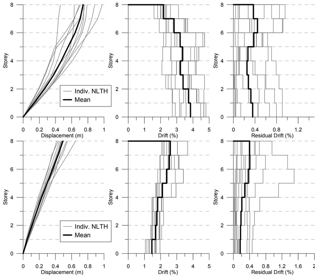
**Figure 5.3.** NTHA peak displacement (left panels), drift (central panels), and residual drift (right panels) results for DBD (upper panels) and FBD (lower panels) mixed systems at 150% of the design intensity
