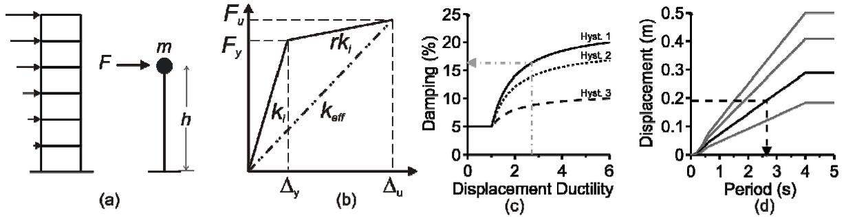
**Figure 2.1.** Key steps of DBD for MODF systems: (a) equivalent SDOF system, (b) effective stiffness and ductility, (c) EVD vs. ductility, (d) design displacement spectra (adapted from Priestley *et al.*, 2007)
