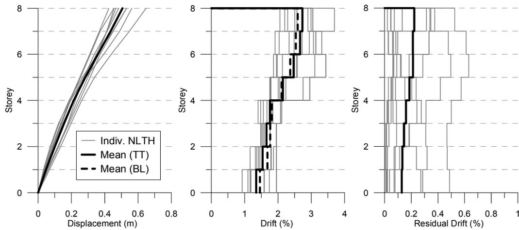
**Figure 5.4.** NTHA peak displacement (left panel), drift (central panel), and residual drift (right panel) results for FBD mixed systems with Takeda thin (TT) rule used for steel portion of frame at 150% of the design intensity
