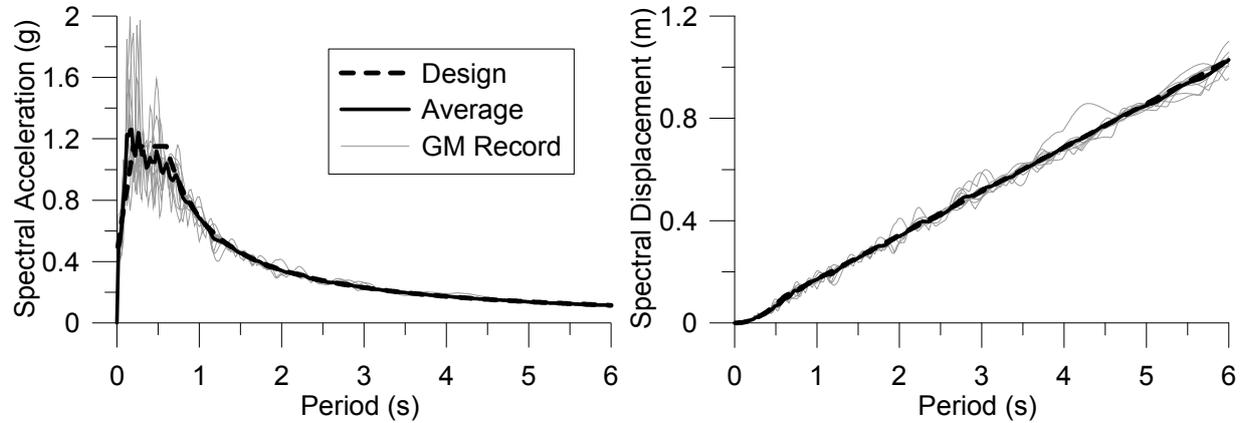
**Figure 4.2.** Design acceleration spectra (left panel) and displacement spectra (right panel) with spectra from ground motion set used for NTHA
