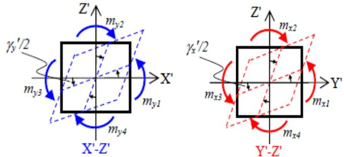
**Figure 3.2.2.** Shearing moment and shearing deformation angle (Kozo System Corporation)
