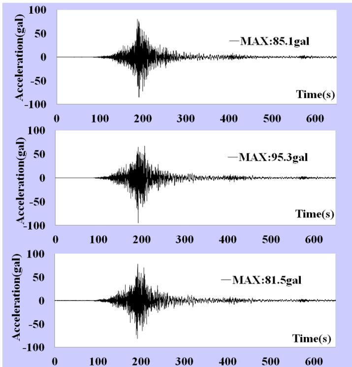
**Figure 3.2.1.** Input acceleration wave (Top: EW, Center: NS, Under: UD)
