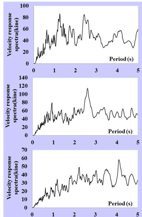
**Figure 3.2.2.** Velocity response spectra (Top: EW, Center: NS, Under: UD)
