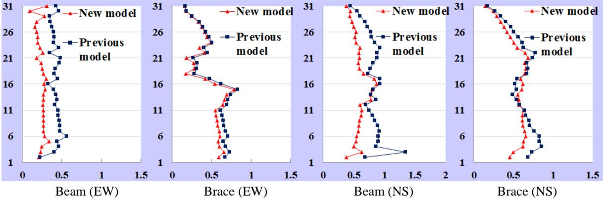
Figure 4.5. The maximum plasticity rate
