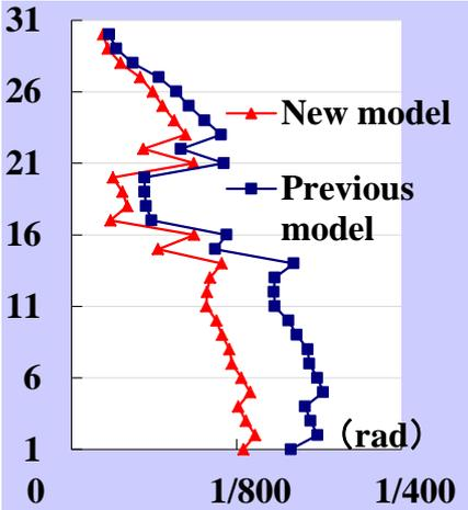
Figure 4.6. The maximum story drift angle (EW)
