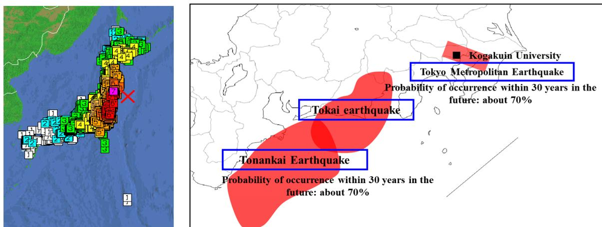
**Figure 1.1.** Distribution of seismic intensities of Tohoku Earthquake (Japan Meteorological Agency) and distribution of scenario earthquakes (The Headquarters for Earthquake Research Promotion)
