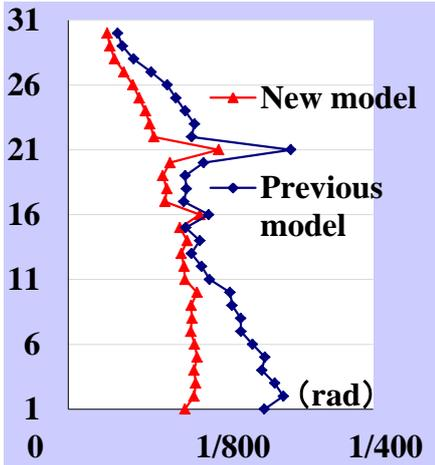
Figure 4.7. The maximum story drift angle (NS)
