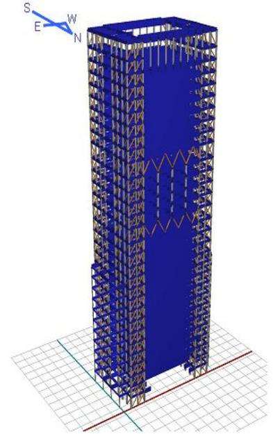
**Figure 3.2.1.** Axonometry of 3-D moment frame model
