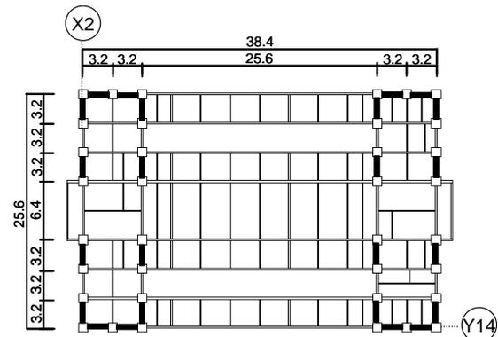
**Figure 2.2.** University standard flaming plan
