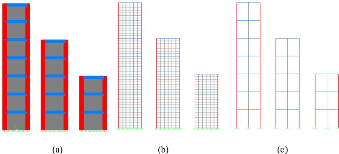
**Figure 4.** Two dimensional 3, 5 and 7-story frames (a) physical model (b) analytical model with multi-layer shell elements (c) analytical model with mid-pier frame elements
