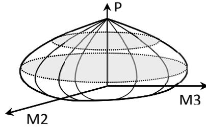
**Figure 3.** Typical P-M-M interaction curve
