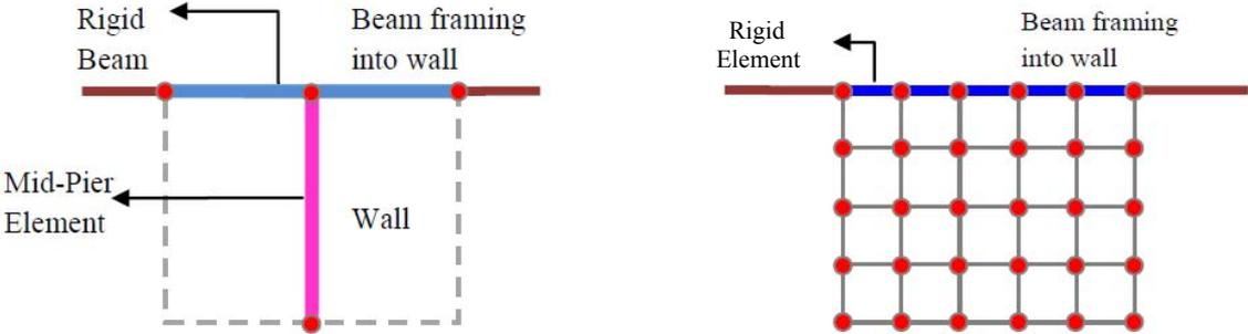
**Figure 1.** FE model definition of RC shear wall
