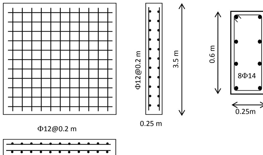
**Figure 5.** Reinforcement distribution in the shear wall and column
