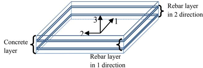
**Figure 2.** Multi-layer shell elements
