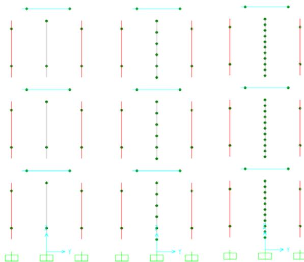
**Figure 7.** Variation of potential plastic hinge for 3-story frame
