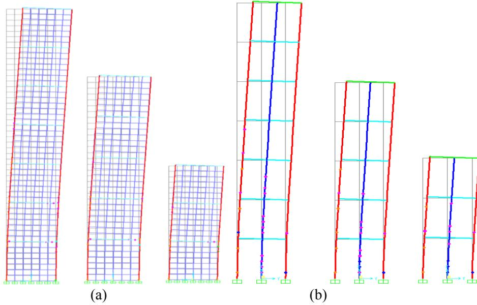
**Figure 6.** Deformed shapes (a) Multi-layer shell element model (b) Shear walls with mid-pier frame models
