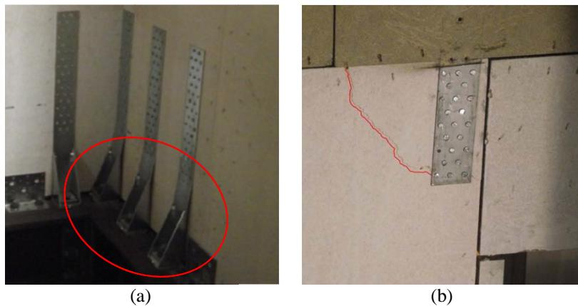
**Figure 3.1** Seismic induced damages: (a) buckled hold-down; (b) crack on the panel hardboard
