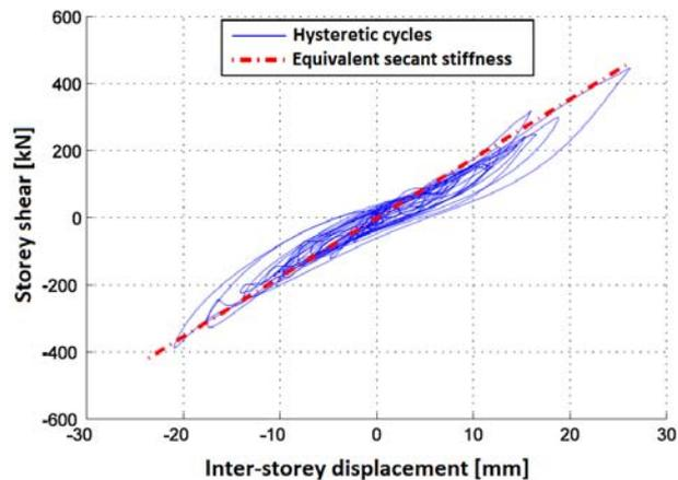
**Figure 4.2** Example of storey shear – inter-storey displacement hysteretic cycles
