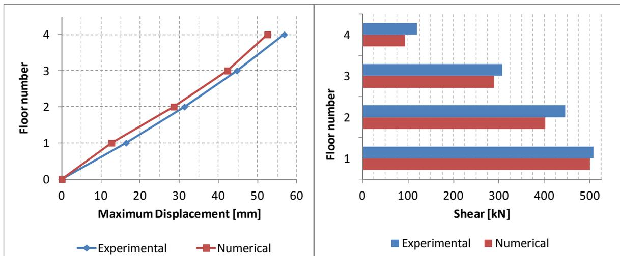
Figure 5.3 Test 0.90g: storey displacements (left) and shear values (right)
