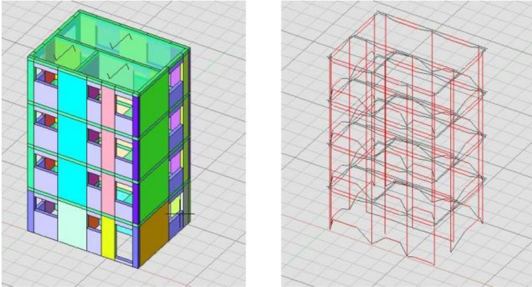
**Figure 4.1** Equivalent macro-frame modelling of the building
