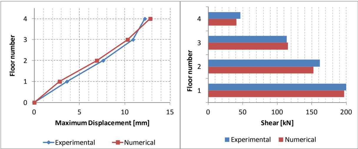
Figure 5.1 Test 0.33g: storey displacements (left) and shear values (right)
