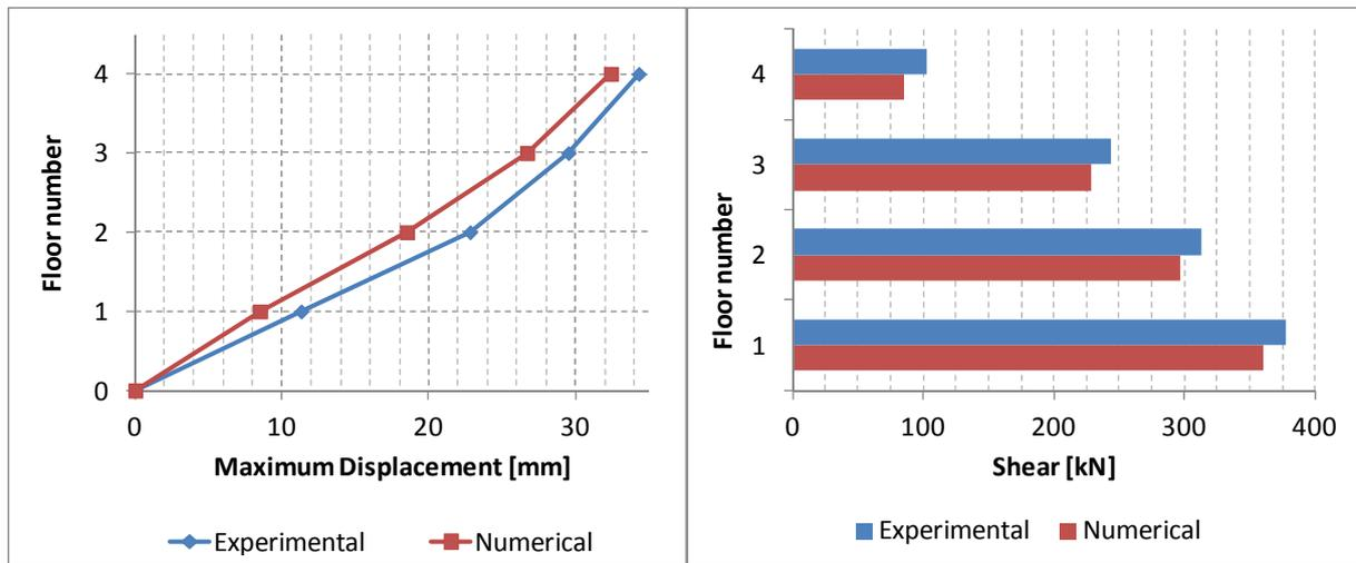
Figure 5.2 Test 0.66g: storey displacements (left) and shear values (right)
