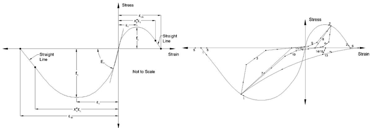
Figure 2. Stress-strain relation (left) and hysteresis behavior (right) – “Concrete07” (OpenSees)
