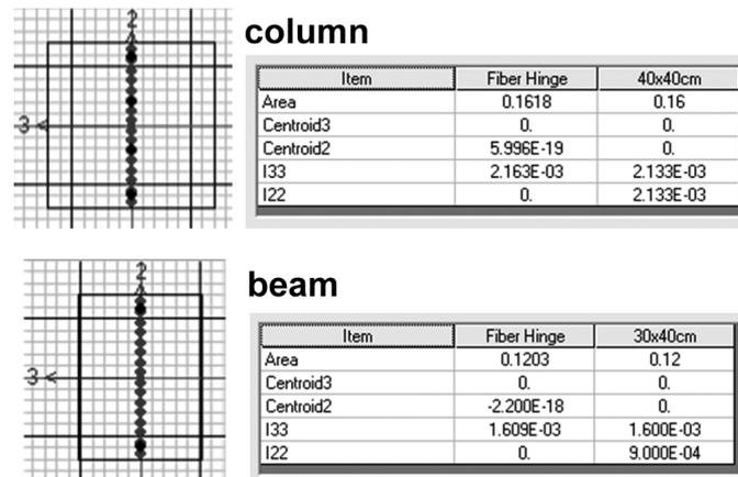
Figure 6. Fibre model for the column and beam cross sections (SAP2000 and OpenSees)
