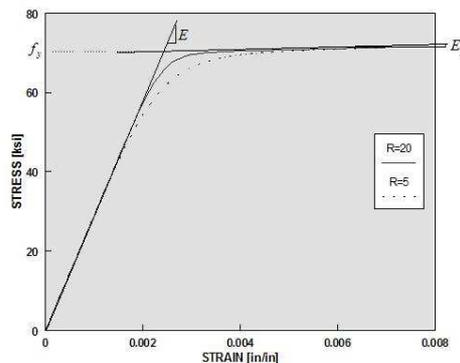
Figure 3. Stress-strain relation – “Steel02” (OpenSees)
