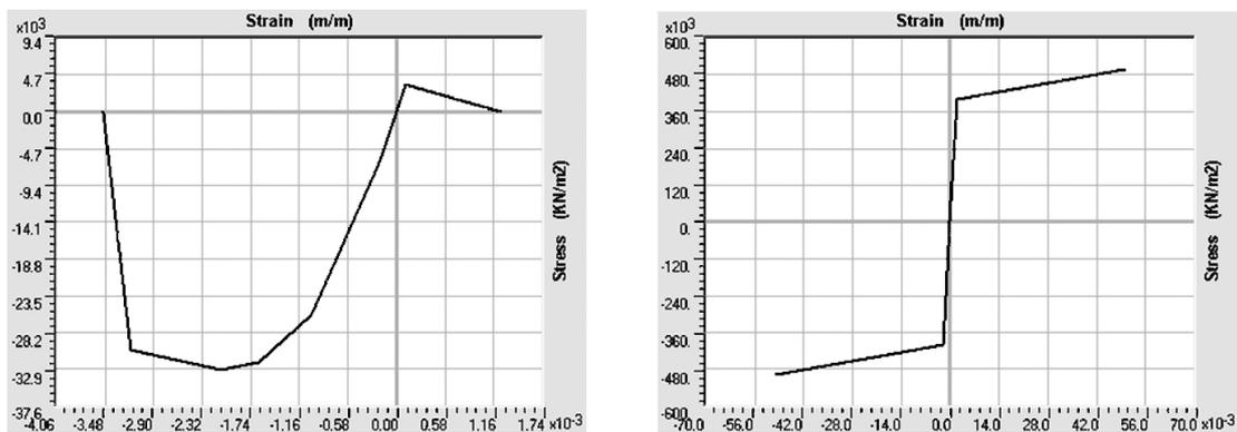
Figure 5. Stress-strain relation for concrete (left) and for reinforcement (right) – SAP2000
