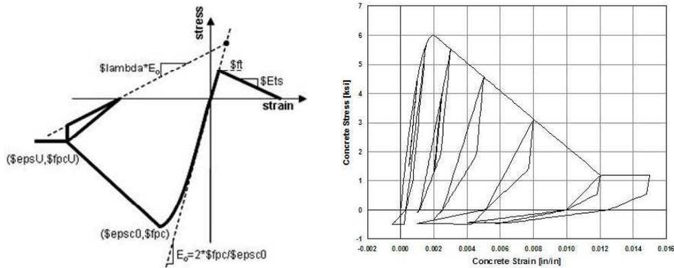
Figure 1. Stress-strain relation (left) and hysteresis behavior (right) – “Concrete02” (OpenSees)
