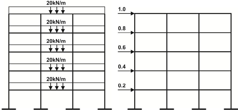
Figure 8. Gravity load (left) and distribution of the lateral forces at the structural height (right)
