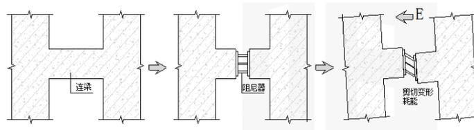
**Figure 5.1.** Composition of energy dissipation lintel
