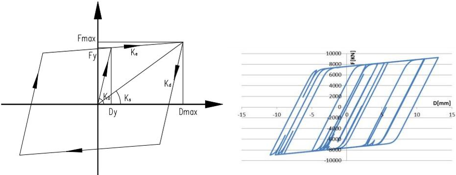
Figures 3.2 and 3.3 Ideal elastic-plastic model Hysteresis curve of typical
