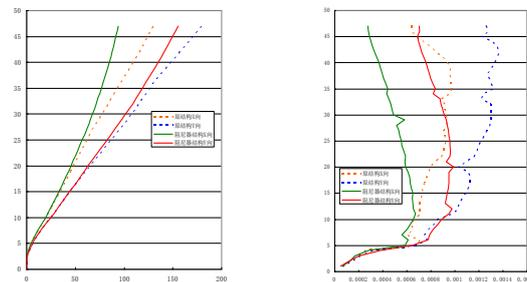
**Figure 5.5.** Comparison of floor displacement and interlayer displacement angle between traditional structure and energy dissipation structure
