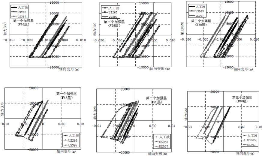
(c) Buckling Restrained Braced hysteresis curve
