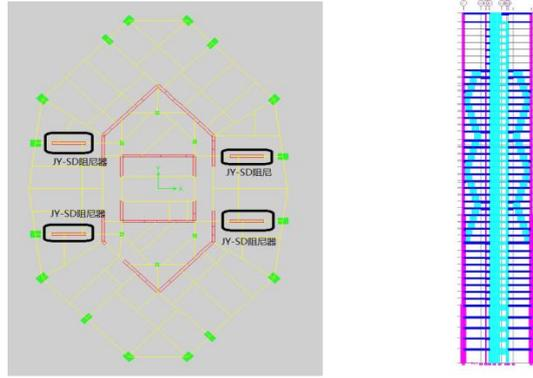
**Figure 4.4.** Plane and façade arrangement of damper
