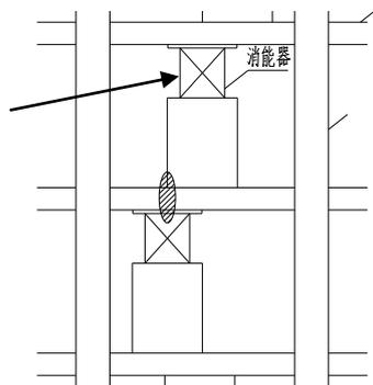
**Figure 4.5.** Vertical arrangement of damper
