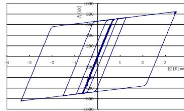
**Figure 5.3.** Hysteresis curve of energy dissipation lintel when ideal elastic-plastic model is adopted
