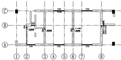
**Figure 5.2.** Arrangement plane of energy dissipation lintel
