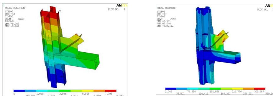
**Figure 2.3 (left).** Schematic diagram for the BUCKLING RESTRAINT BRACE node
