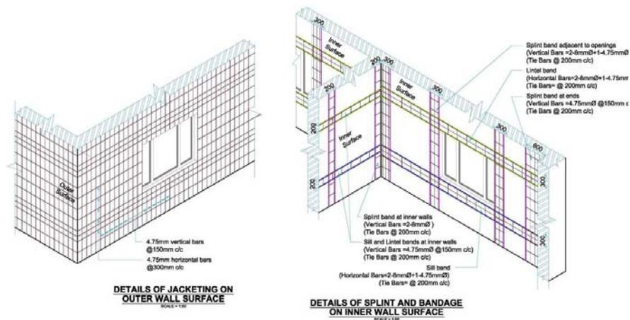
Figure 2. Typical design of proposed retrofitting ( source NSET)
