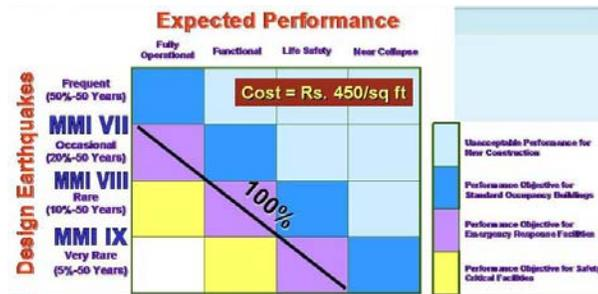
Figure 4. Expected performance of the buildings after retrofitting (source NSET)
