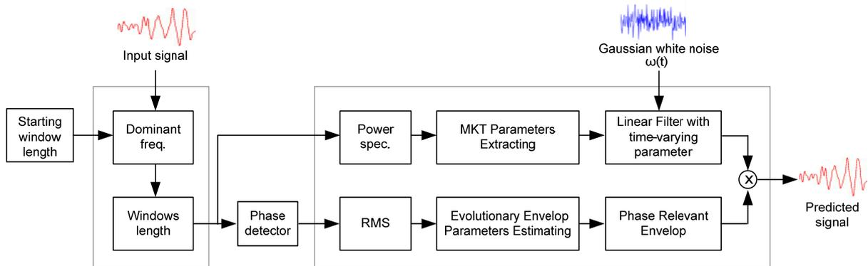
**Figure 1.** Schematic of the real-time stochastic prediction model
