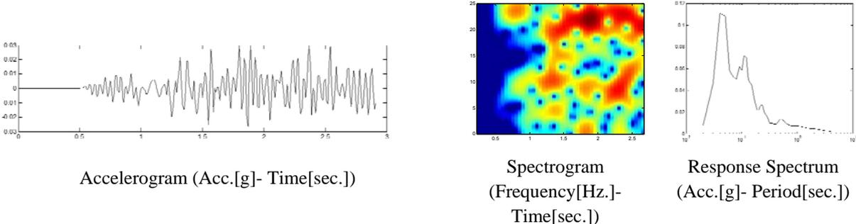
**Figure 10.** Predicted strong ground motion accelerogram, spectrogram and response spectrum of dominant P-wave of Northridge 1994 recorded at LA - Chalon Rd
