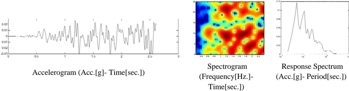
**Figure 9.** Observed strong ground motion accelerogram, spectrogram and response spectrum of dominant P-wave of Northridge 1994 recorded at LA - Chalon Rd
