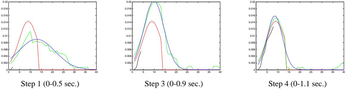
**Figure 8.** Evolutionary envelope function for dominant P wave. The red, green, blue and black curves represent the target, the predicted, the fitted predicted and the real-time measured envelope functions, respectively
