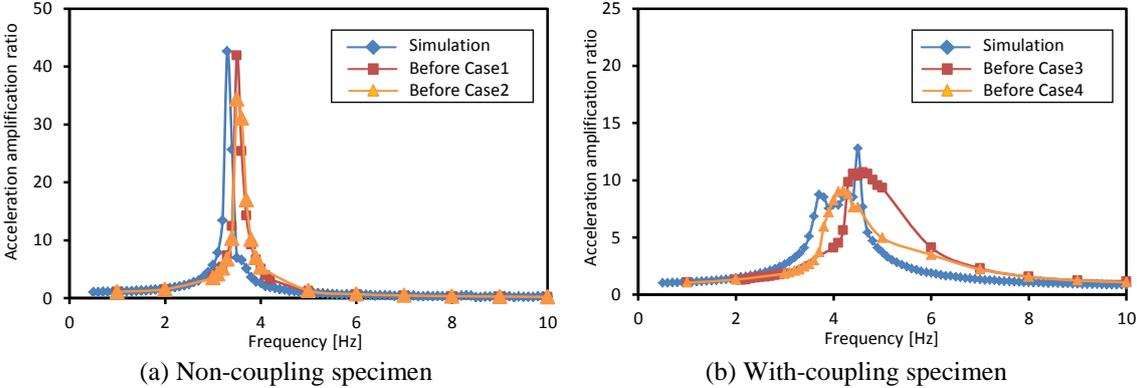
**Figure 14.** Comparison of the experimental results with the FEA results in the resonance tests
