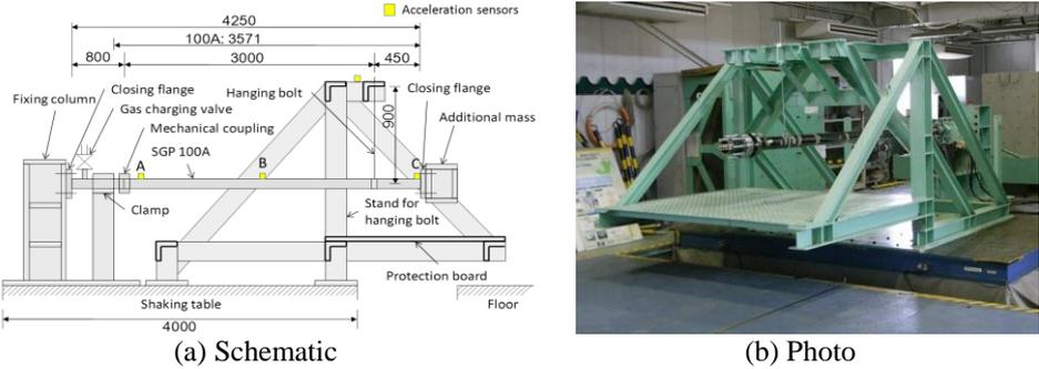
Figure 2. Shake-table test apparatus and partial-piping specimen
