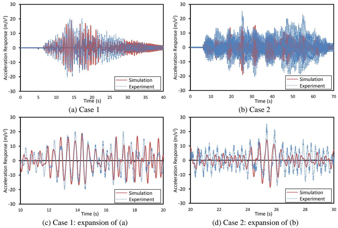
**Figure 15.** Comparison of the experimental results with the FEA results in the seismic response tests for the non-coupling specimens
