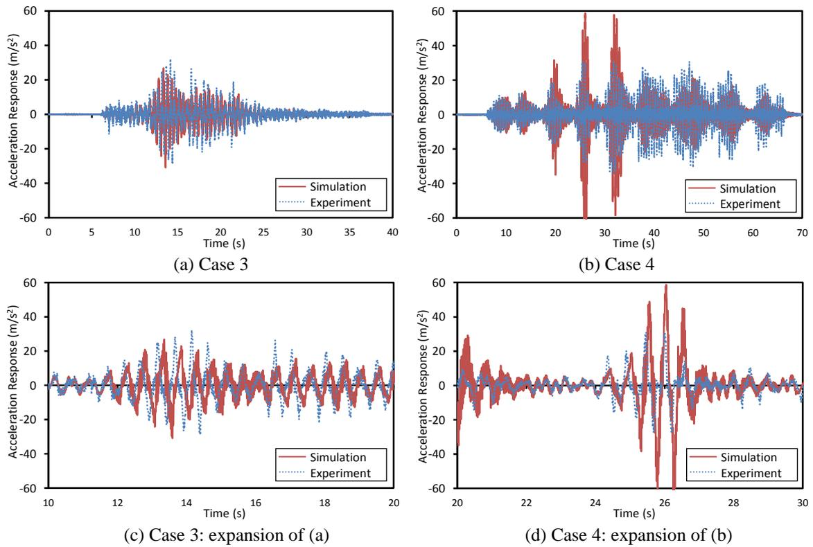
**Figure 16.** Comparison of the experimental results with the FEA results in the seismic response tests for the with-coupling specimens
