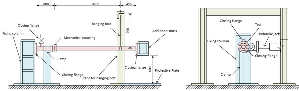
**Figure 8.** Schematic of the static bending test apparatus
