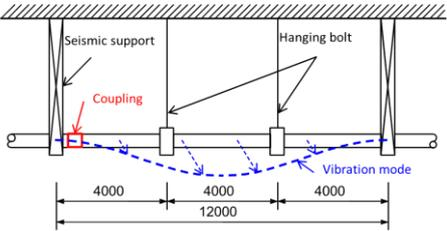
Figure 1. Illustration of the dominant vibration mode in the three spans
