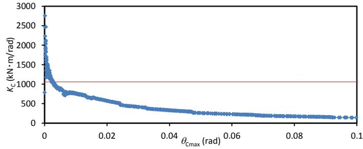
**Figure 11.** Stiffness of the rotational spring vs. the maximum experienced rotational angle
