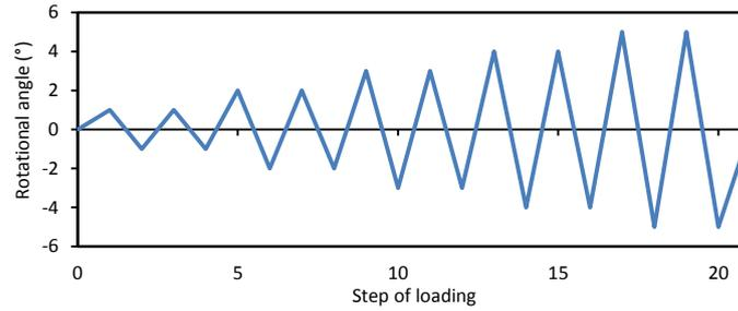
**Figure 9.** Target alternative loading program in the static bending test
