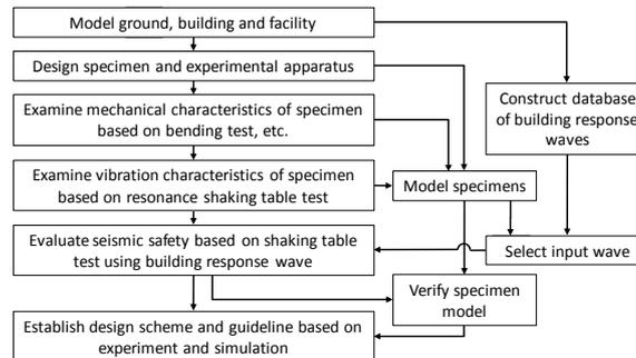
Figure 17. Proposed framework for the method of evaluation of seismic safety for the interior-piping
