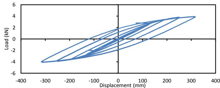
**Figure 10.** Result of the static bending test for the non-coupling specimen
