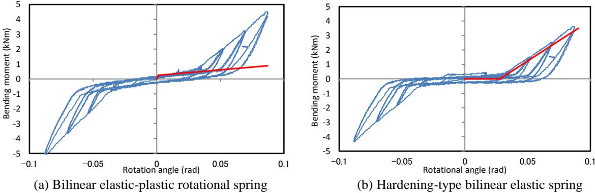
**Figure 13.** Result of the static bending test for the with-coupling specimen and the determined characteristics of the two bilinear springs (shown as red lines)
