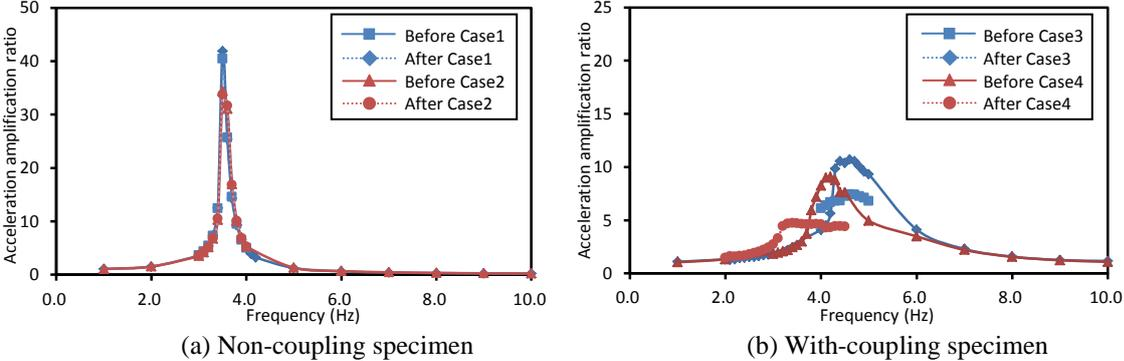
Figure 6. Results of the resonance tests using the shake-table
