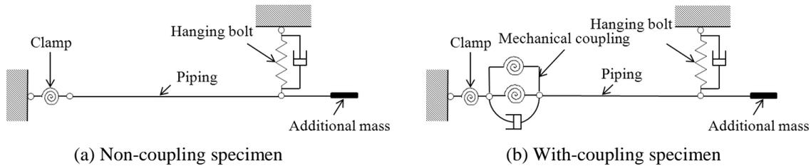
**Figure 12.** Proposed simplified analytical models
