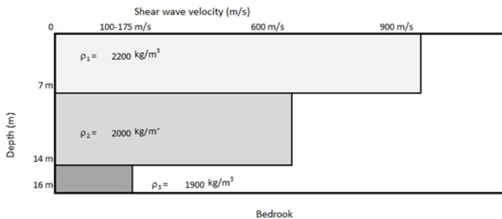
**Figure 3.2.** (a) A schematic drawing of a section showing a hypothetical shear wave velocity profile from the building site (Stray 2010).
