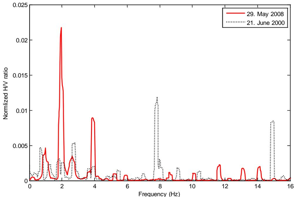
**Figure 2.4.** The normalised H/V-ratio as a function of frequency for the two earthquakes in 2000 and 2008.
