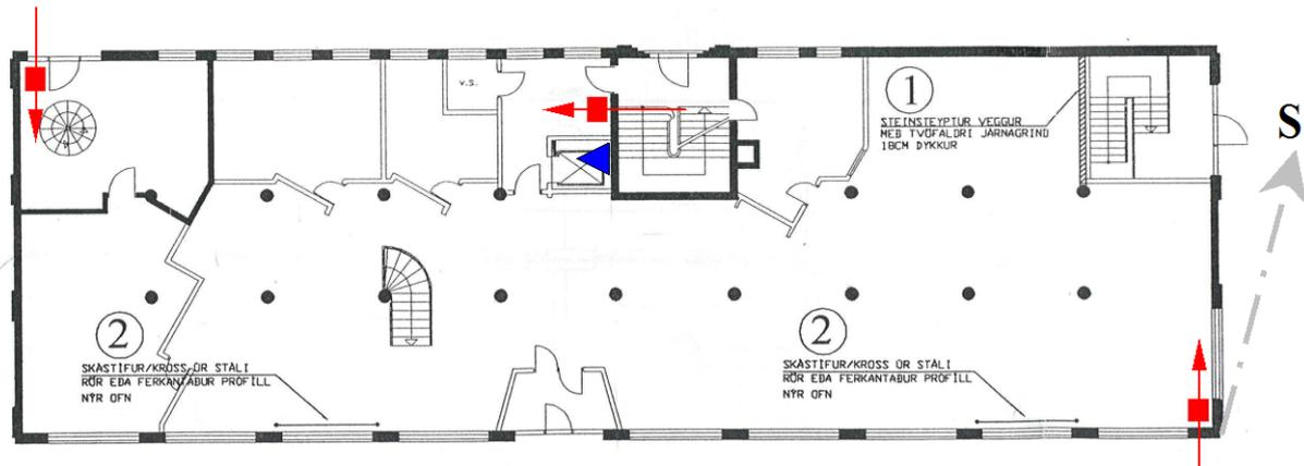
**Figure 1.3.** The Town Hall at Selfoss, plan view of the ground floor. The location of uni-axial (squares) and tri-axial (triangle) accelerometers within the building plan as well as their positive direction is shown. Note the location of the steel cross-braces (2) and reinforced concrete wall (1) installed in spring 2000 for retrofitting.
