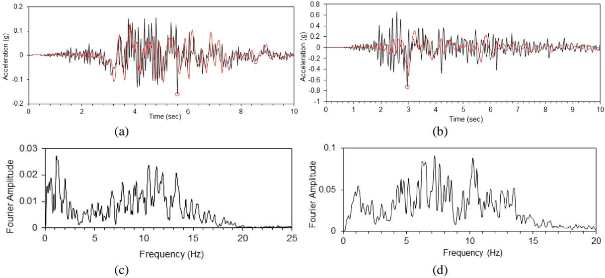
**Figure 3.3.** N-S acceleration component, the red line is the recorded accelerations from the basement and the black line is calculated accelerations on the bedrock. Fourier spectra of the calculated N-S bedrock component.
