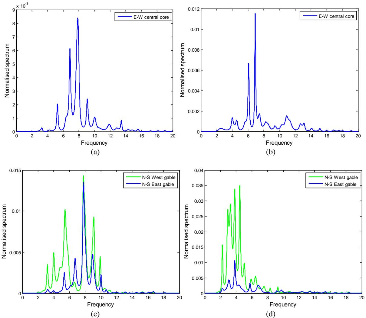
**Figure 2.3.** Power spectral densities of relative acceleration response on the third floor. (a) The E-W component from the event on June 21. 2000; (b) The E-W component from the event on May 29. 2008; (c) The N-S components from the event on June 21. 2000; (d) The N-S components from the event on May 29. 2008. The blue line in (c) and (d) represents the motion of the west gable but the green line the motion of the east gable.
