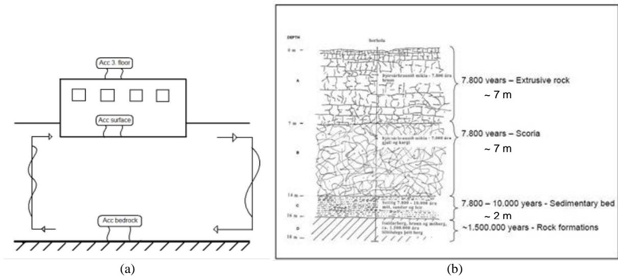
**Figure 3.1.** (a) A schematic drawing of the structure-soil interaction system. (b) A section showing a hypothetical rock-soil profile from the building site (Stray 2010).
