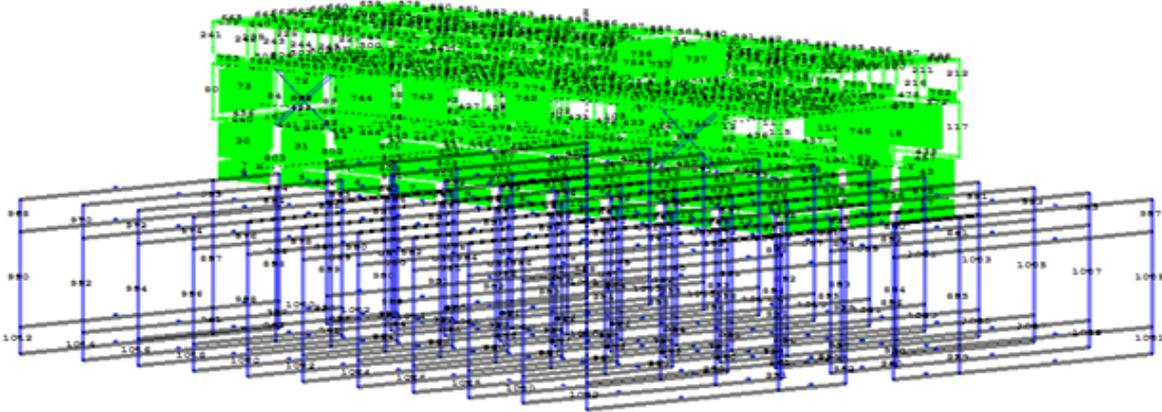
**Figure 3.4.** The Ruaumoko 3D -finite element model. The blue squares indicate the soil springs. The concrete beam- and shells elements representing the building are green and the steel beam x-bracing elements in the two frontal windows are blue.
