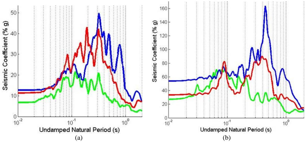
**Figure 2.1.** Response spectra evaluated from the basement records. (a) The event on June 21, 2000; (b) The event on May 29, 2008. The blue line is the N-S component, red line is the E-W component and the green line is the vertical direction. The damping is 5% of critical damping.
