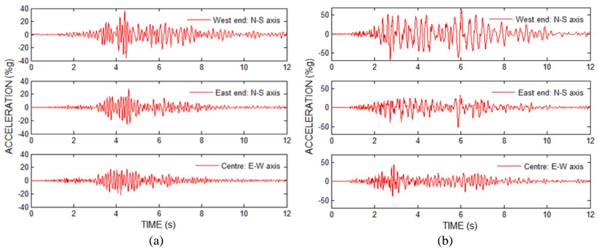
**Figure 2.2.** Time-series of acceleration response on the third floor. (a) The event on June 21, 2000; (b) The event on May 29, 2008.
