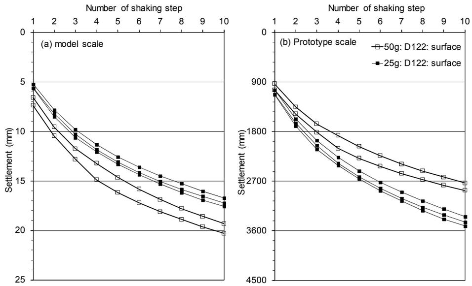
**Figure 11.** Cumulative settlements after each shaking: (a) model scale, (b) prototype scale
