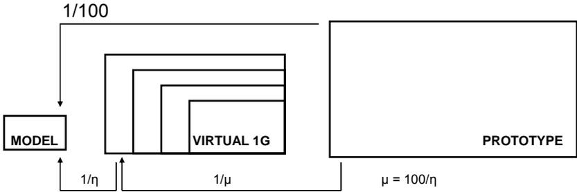
**Figure 1.** Relationship among prototype, virtual 1G model and centrifuge model for the case of scaling factor of 1/100 ( $\lambda = \mu\eta = 100$ )
