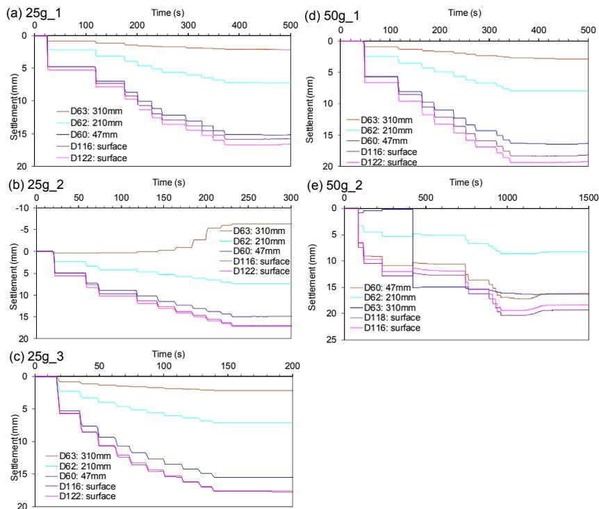
**Figure 10.** Time histories of ground settlements due to shaking (model scale)
