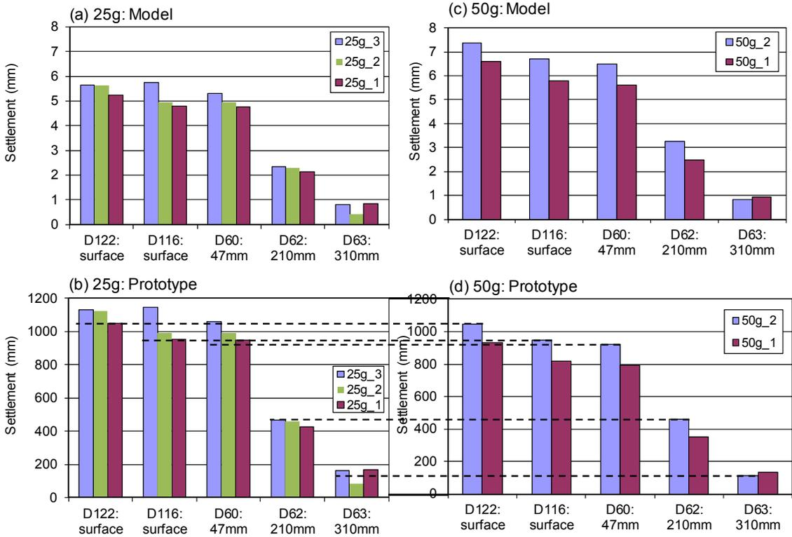
**Figure 13.** Summary of settlements measured in all the test cases: (a) 25 g in model scale, (b) 25 g in prototype scale, (c) 50 g in model scale, (d) 50 g in prototype scale
