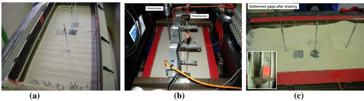
**Figure 4.** Model setup (a) Installation of settlement gauge, (b) Setup of penetrometer and potentiometers, and (c) settlement gauges and PVC plates after the test
