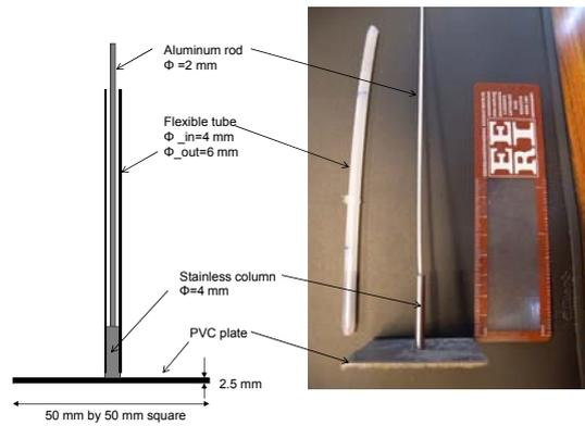
**Figure 3.** Detail of a settlement gauge
