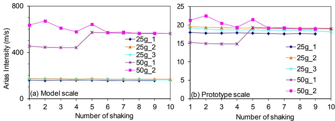
**Figure 6.** Arias intensity of the recorded input acceleration: (a) model scale and (b) prototype scale
