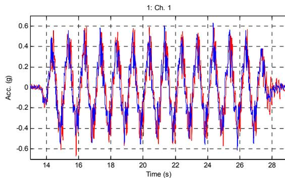
**Figure 5.** Time histories of input acceleration in prototype scale (red 25g\_1, blue 50g\_1)
