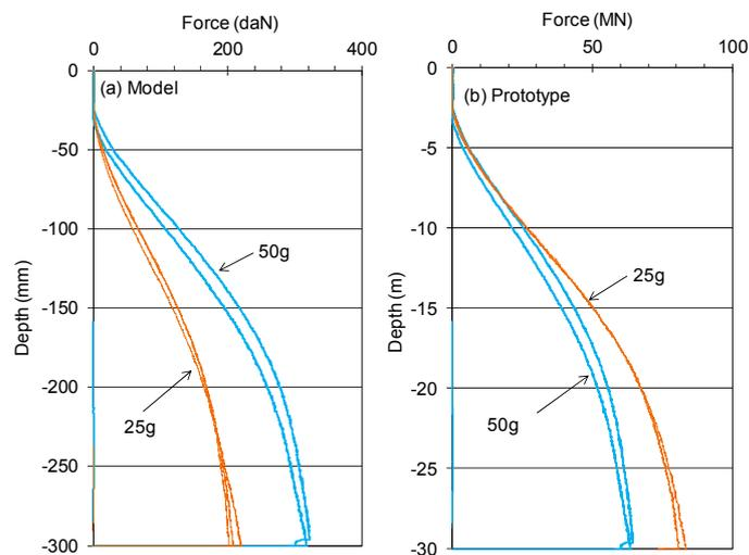
**Figure 8.** Penetrometer resistance after the 10th shaking in model scale (a) and prototype scale (b).
