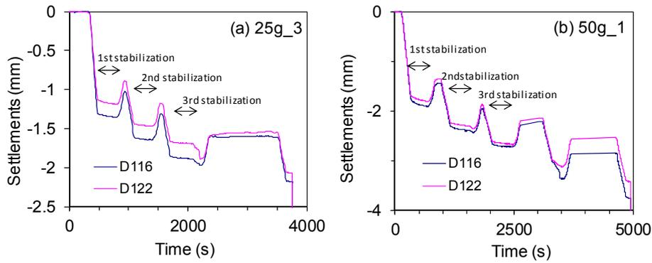
**Figure 9.** Time histories of ground settlements due to consolidation before shaking (model scale): (a) 25g\_1 and (b) 50g\_1
