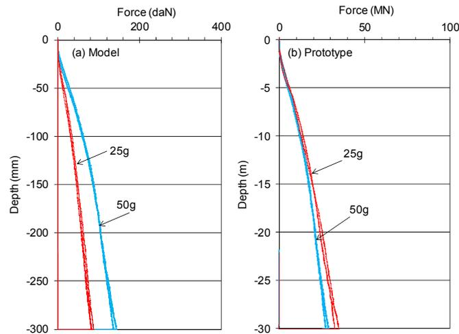
**Figure 7.** Penetrometer resistance before the initial shaking in model scale (a) and prototype scale (b).
