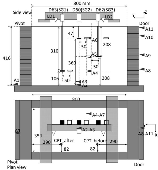
**Figure 2.** Schematic view and sensor location of the model
