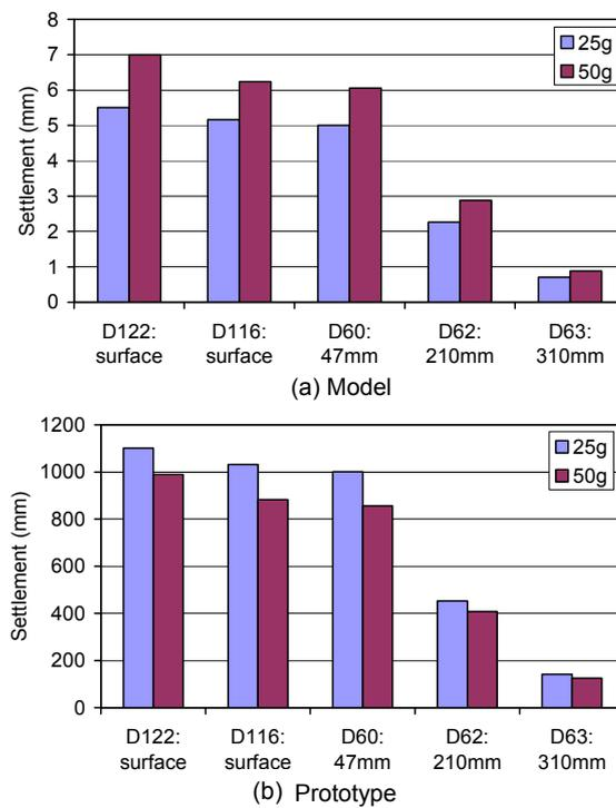
**Figure 12.** Comparison of averaged settlements measured in 25 g and 50 g: (a) model scale, and (b) prototype scale
