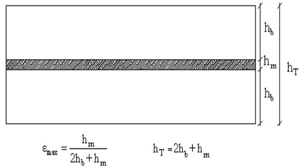
**Figure 2.2** Definition for the fracture of an interface and maximum tensile assumption (Jafarov and Köksal, 2011)
