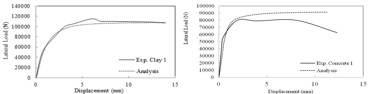
**Figure 2.4** Load- displacement curves for URM walls
