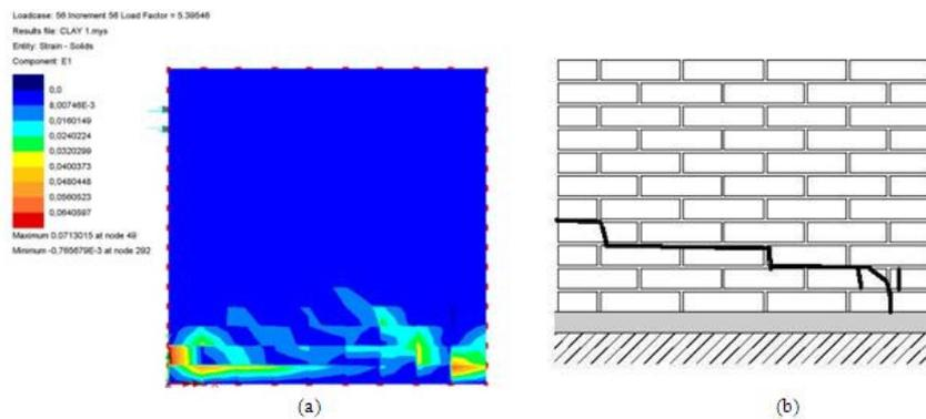
**Figure 2.6** (a)Maximum stains over the URM wall (b) and crack patterns on clay1 wall (Stratford et.al 2004)
