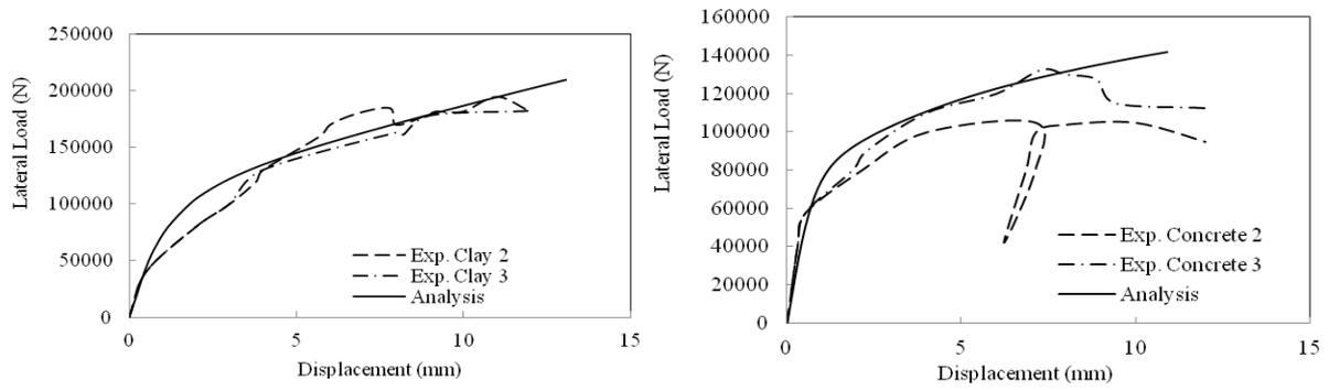
**Figure 2.5** Load- displacement curves for strengthened walls with GFRP
