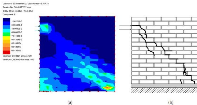
**Figure 2.7** (a) Maximum stains over the strengthened wall with GFRP (b) and crack patterns on concrete 2 wall (Stratford et. al 2004)
