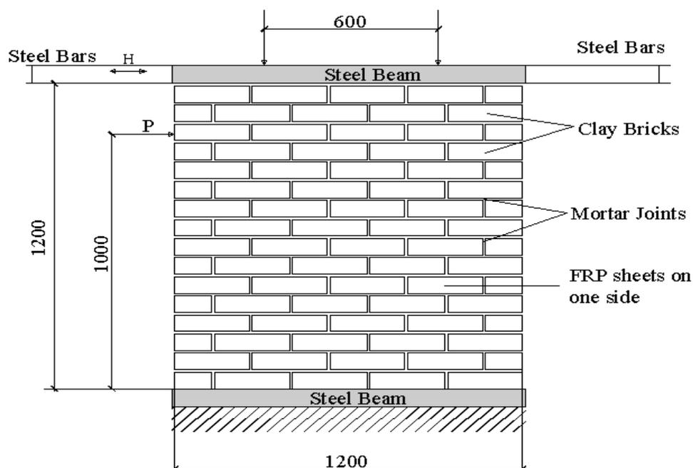
**Figure 2.3** Experimental setup (Stratford et al., 2004)
