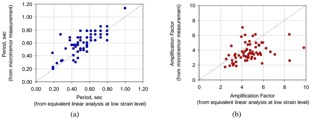
**Figure 5.1.** Comparison of results from microtremor measurements and linear analysis; (a) Predominant period and (b) Amplification factor.
