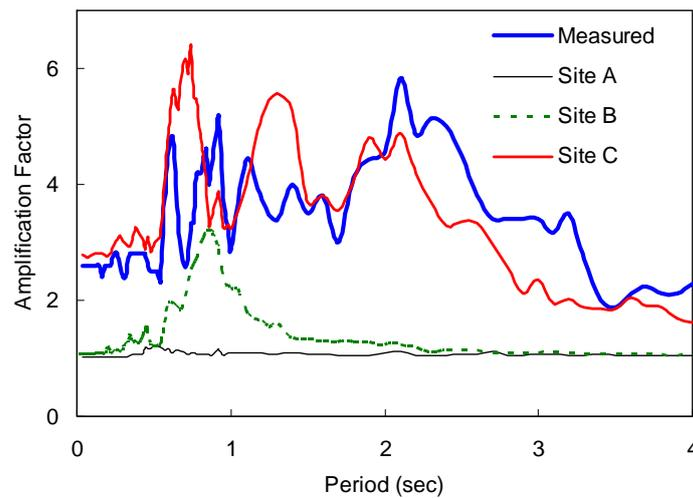
**Figure 5.2.** Amplification factor of four sample sites from the effect of an earthquake of magnitude 6.9 at 780 km distance.
