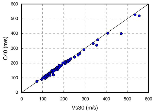
**Figure 4.1.** Comparison of  $V_{S30}$  and its estimation by phase velocity with wave length of 40 m
