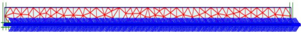
**Figure 3.** FEM-RO model used to compare results with one-dimensional analysis (Chitas, 2008)
