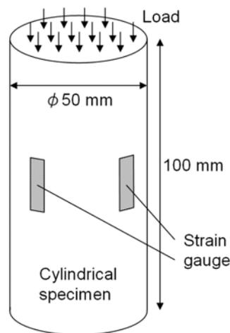
**Figure 1.** Cylindrical mortar specimen
