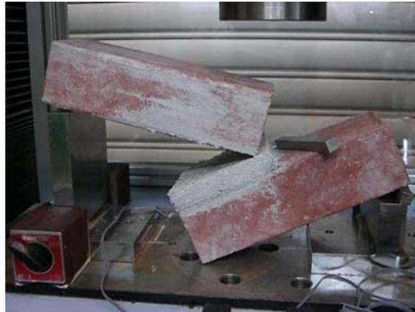
**Photo 2.** Failed specimen of peeling strength test
