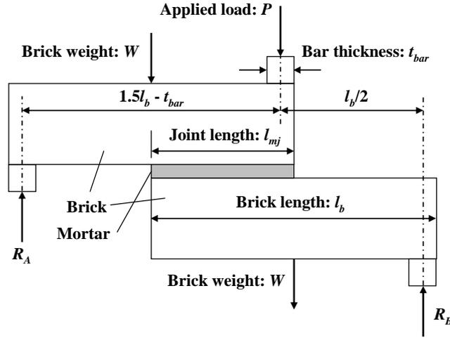
**Figure 2.** Masonry specimen of peeling strength test
