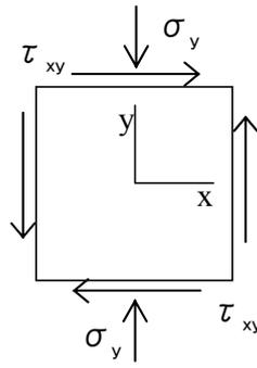
**Figure 8.** Stress element of biaxial stress state
