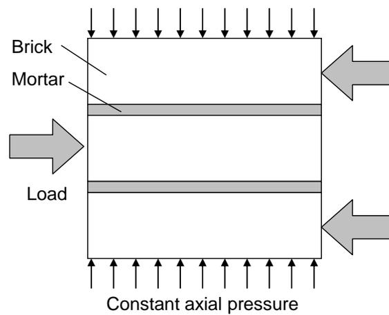
**Figure 4.** Brick triplet specimen of shear strength test
