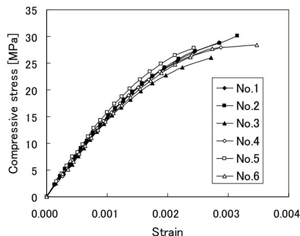
**Figure 5.** Stress-strain relations of mortar
