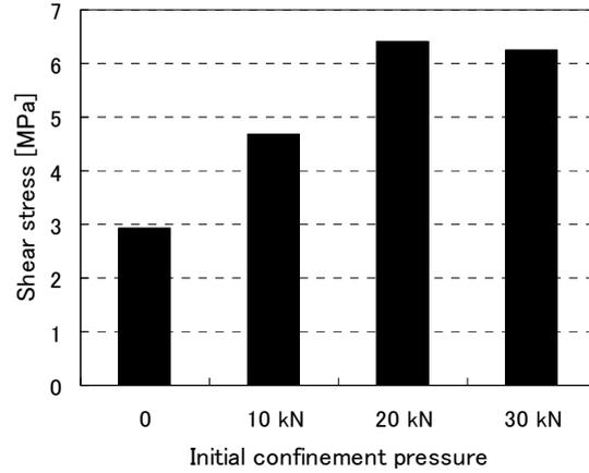
**Figure 6.** Shear stress-initial confinement pressure relation
