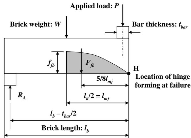
**Figure 3.** Free body diagram of peeling strength test
