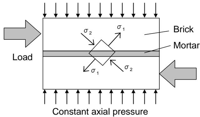
**Figure 7.** Stress state of the specimen in shear strength test
