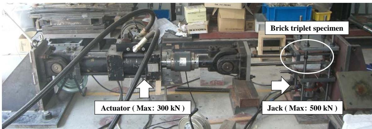
**Photo 1.** Devices of shear strength test
