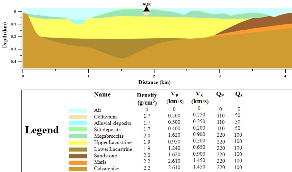
**Figure 3.1.** Computing cross section at L’Aquila through the AQK station with the physical parameters attributed to lithotypes.
