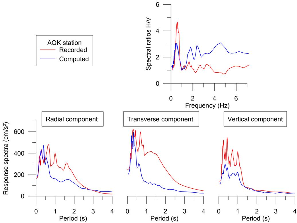
**Figure 3.2.** Comparison at the AQK station of the computed and recorded main shock: (top) H/V spectral ratio; (bottom) response spectra computed for 5% damping.
