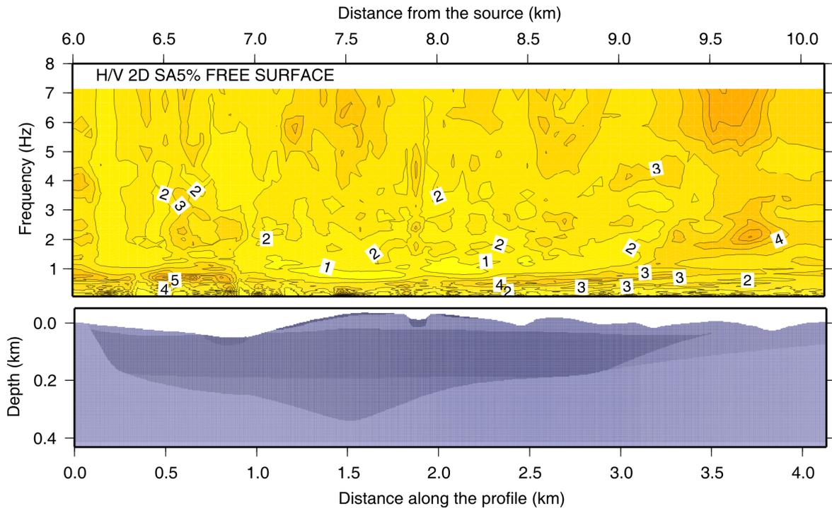
**Figure 3.3.** H/V spectral ratios computed along the cross section at L'Aquila
