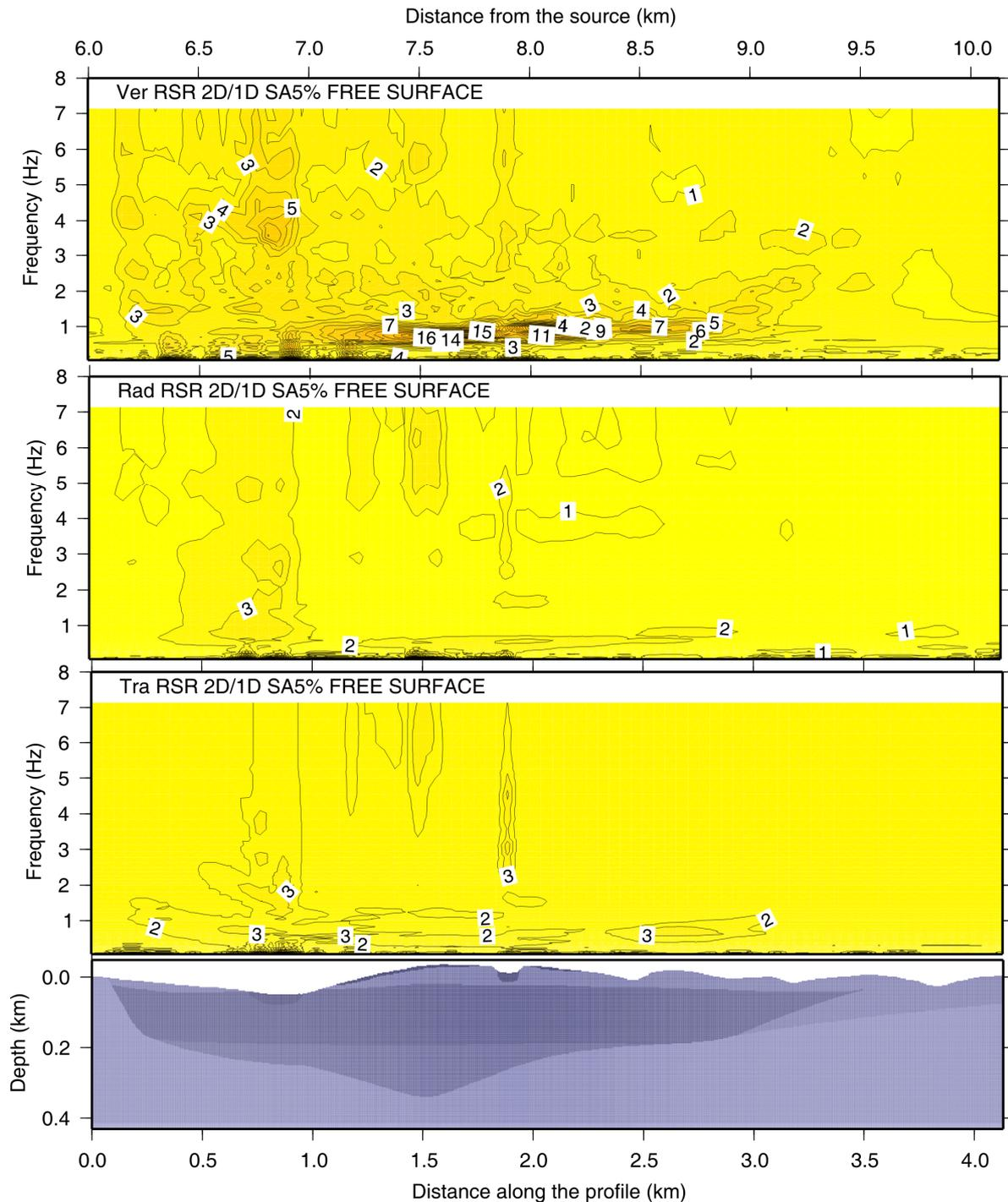
**Figure 3.4.** Spectral amplifications (RSR 2D/1D) along the cross section at L'Aquila. Response spectra are computed for 5% damping. From the top vertical, radial and transverse components of the computed ground motion.
