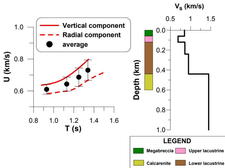
**Figure 2.1.** Rayleigh waves group velocity dispersion curves of fundamental mode extracted by FTAN method from radial and vertical components of the recorded main shock at the AQK station (on the left);  $V_s$  velocities obtained from the non-linear inversion (Hedgehog method) of the average dispersion curve with interpretative stratigraphy (on the right).
