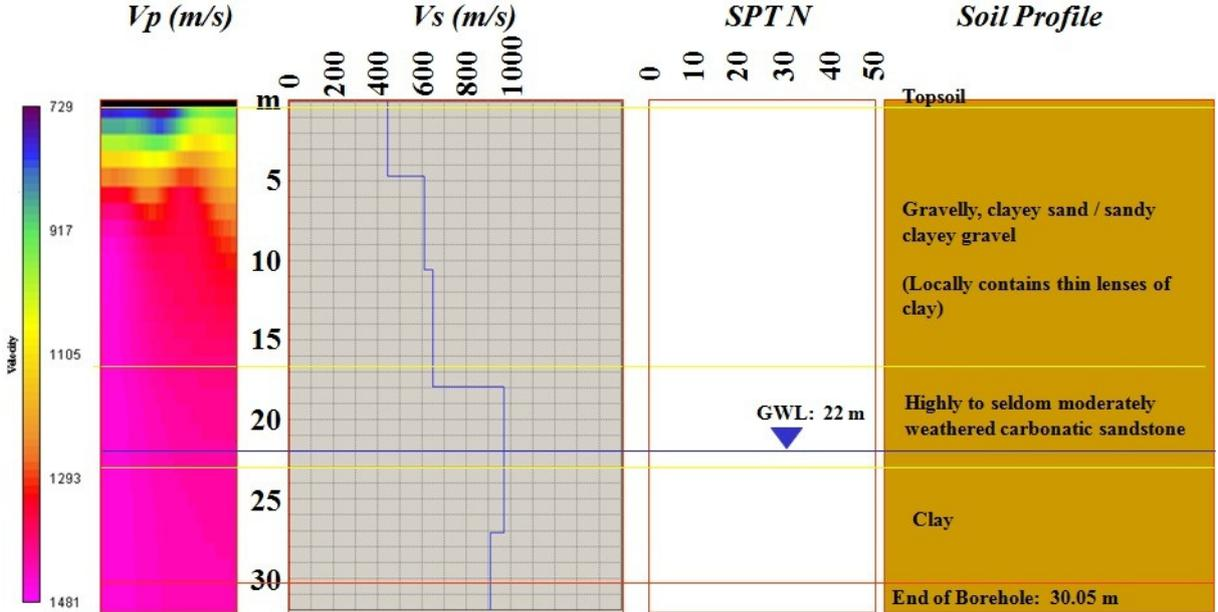
Figure 6. Results of seismic and geotechnical investigations completed at Esentepe station site.
