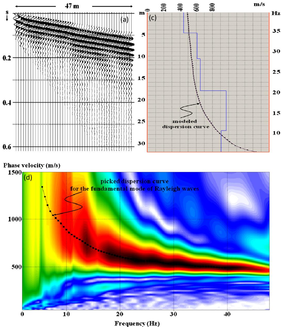
**Figure 5.** (a) off-end shot record, (b) the dispersion spectrum of the surface waves and (c)  $V_s$ -depth profile (blue curve) and the modeled dispersion curve (black curve) for Esentepe station site.
