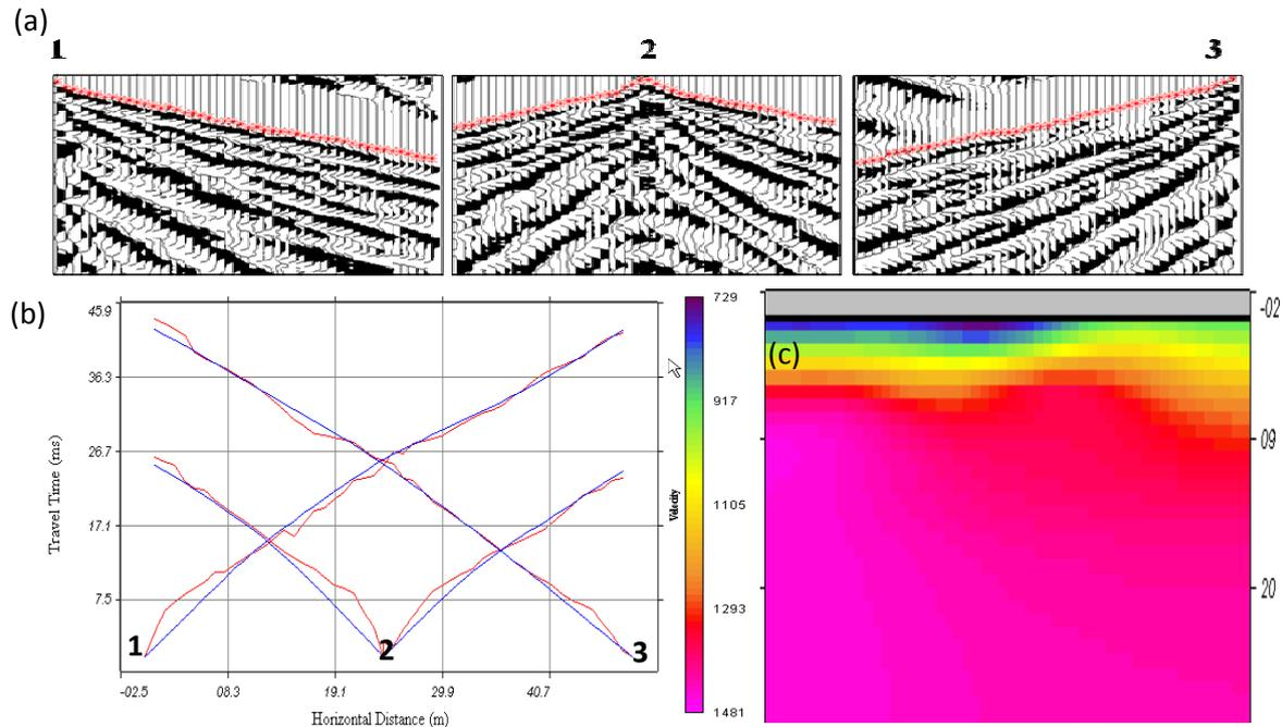
**Figure 4.** (a) First arrival times, (b) travel time curves with blue curve corresponding to modeled and red curve corresponding to actual travel times, (c) a P-wave velocity–depth model along the receiver spread for the Esentepe station
