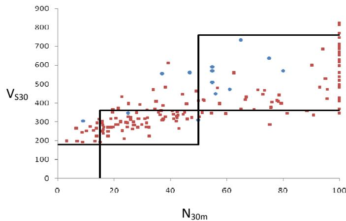
**Figure 7.**  $N_{30m}$ - $V_{s30}$  relationship obtained from this study (blue dots) together with from Sandikkaya et al. (2010) study (red dots). The NEHRP Provision based  $N_{30m}$  and  $V_{s30}$  bands corresponding to site classes C, D and E are shown as well.
