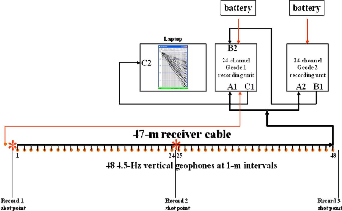
Figure 2. Workflow diagram of field survey in MASW
