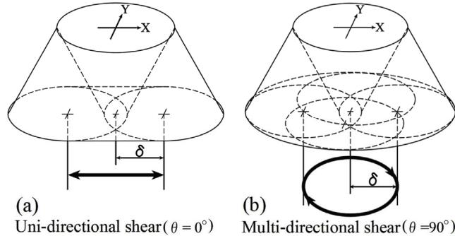
Figure 2.3. Typical deformations of specimen
