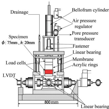
**Figure 2.1.** Outline of the test device
