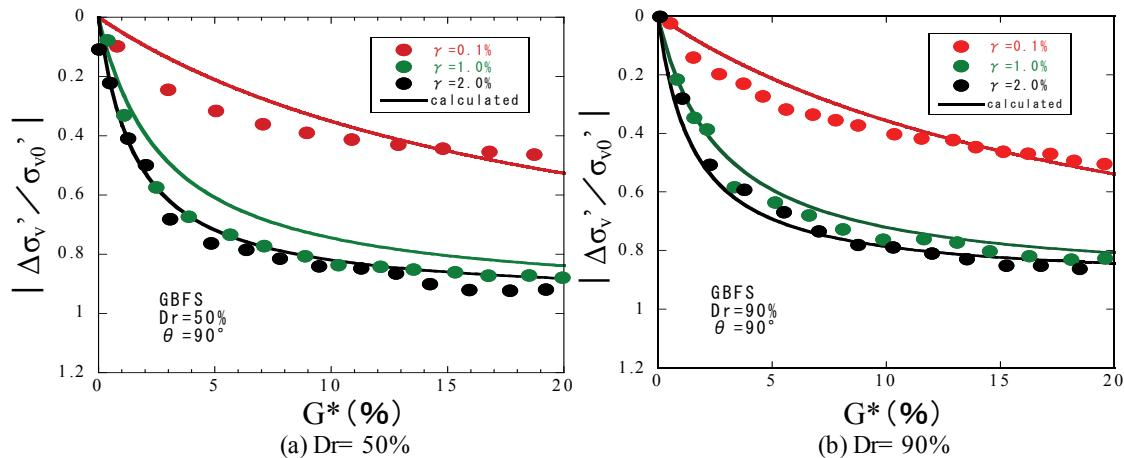
**Figure 3.4.** Comparison between the observed and calculated results for effective stress reduction ratio induced by multi-directional cyclic shear ( $\theta=90^\circ$ ) on GBFS at different relative densities
