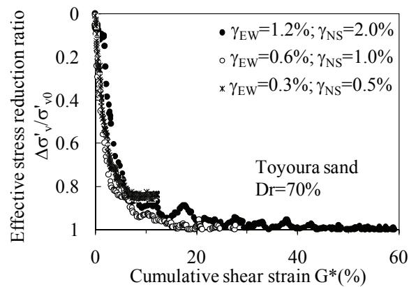
**Figure 3.9.** Relationships between stress reduction ratio and cumulative shear strain during multi-directional irregular cyclic shear tests performed for different scales of shear strain amplitude
