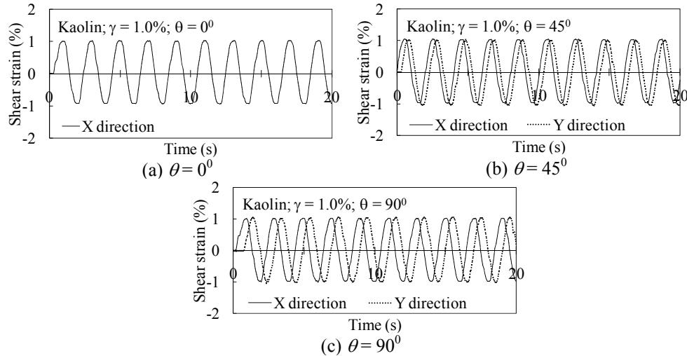
**Figure 2.4.** Time histories of cyclic shear strain at  $\gamma = 1.0\%$  under various phase differences
