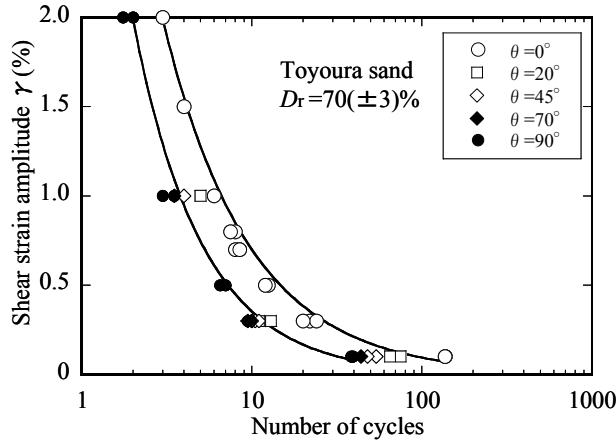
**Figure 3.6.** Relationship between the number of cycles and shear strain amplitude required for liquefaction
