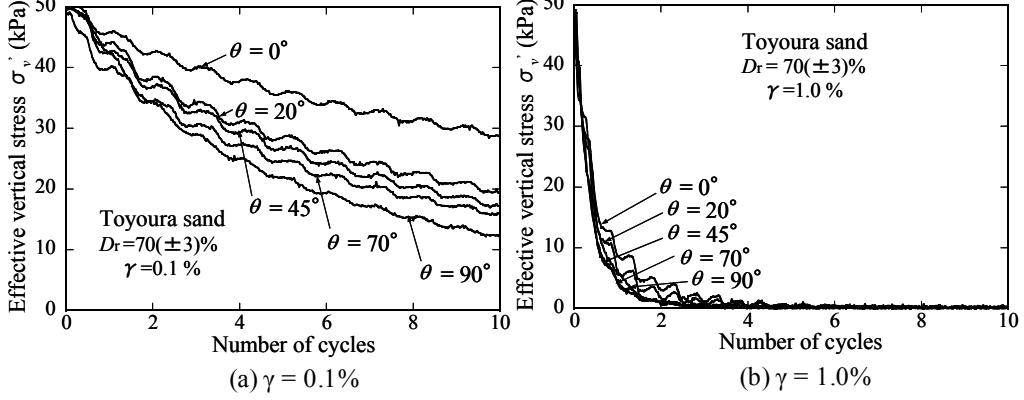
**Figure 3.1.** Effective stress change versus number of cycles
