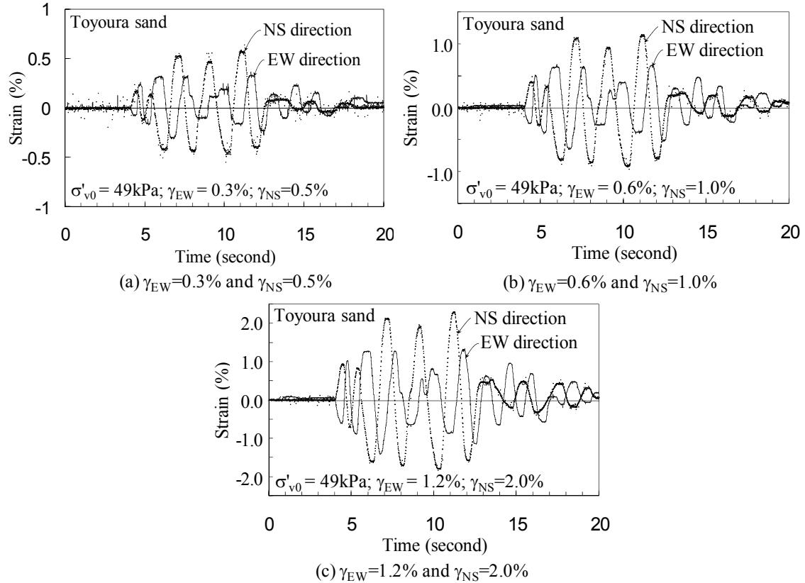
**Figure 3.8.** Time histories of shear strain in multi-directional irregular cyclic shear tests conducted for different scales of shear strain amplitude
