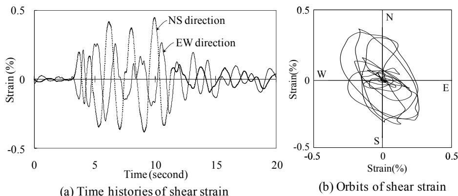
**Figure 1.1.** Time histories and orbits of shear strain at Hyogo-ken Nanbu Earthquake 1995
