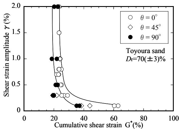
**Figure 3.7.** Relationship between the cumulative shear strain and shear strain amplitude required for liquefaction
