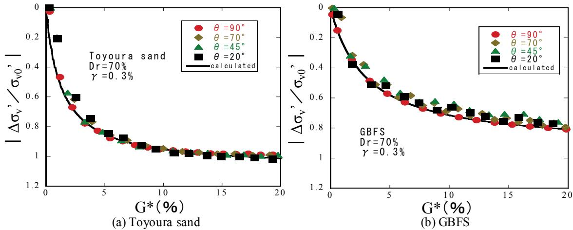
**Figure 3.5.** Comparisons between the observed and calculated results for effective stress reduction ratio on Toyoura sand and GBFS under multi-directional cyclic shear at various phase differences
