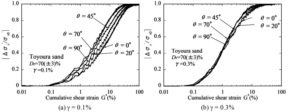
**Figure 3.2.** Effective stress reduction ratio versus cumulative shear strain
