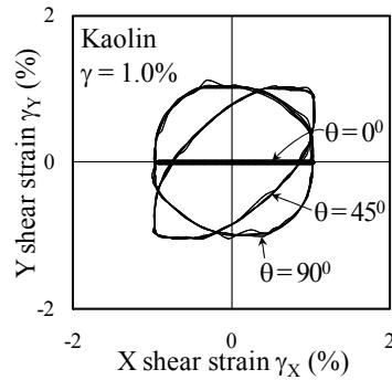
**Figure 2.5.** Orbits of shear strain at  $\gamma = 1.0\%$  under various phase differences
