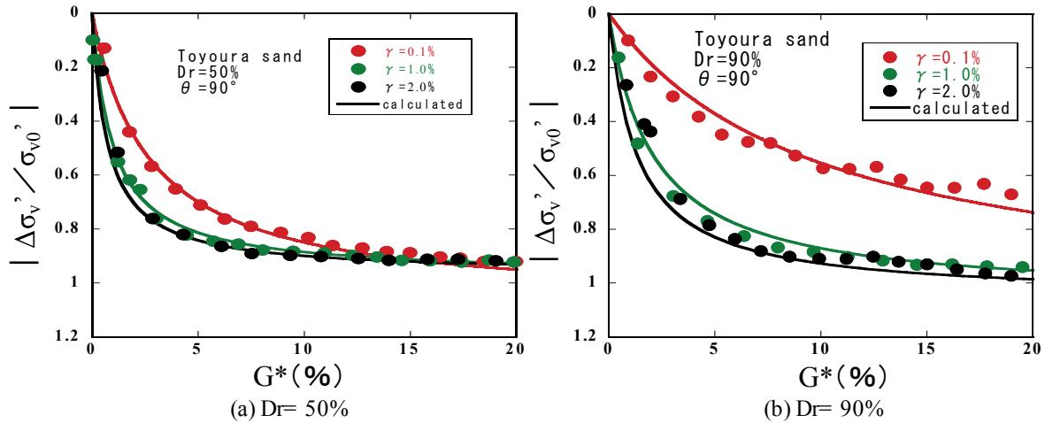
**Figure 3.3.** Comparison between the observed and calculated results for effective stress reduction ratio induced by multi-directional cyclic shear ( $\theta=90^\circ$ ) on Toyoura sand at different relative densities
