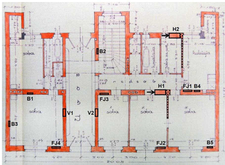
**Figure 2.** Plan of ground floor with positions of in-situ lateral resistance tests (H1 and H2), flat-jack tests (FJ1 to FJ4) and places of the extraction of brick specimens (B1 to B5) and small walls for laboratory compression tests (V1 and V2)
