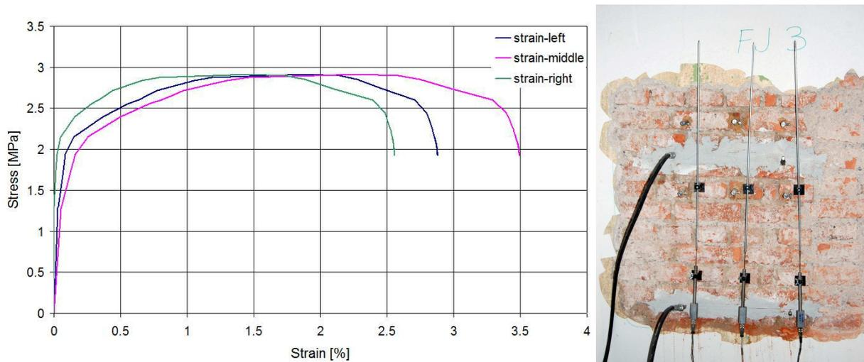
**Figure 4.** Double flat-jack test at the position FJ3: relationships between stress and strain (left) and arrangement of double flat-jack and instrumentation with LVDT's (right)
