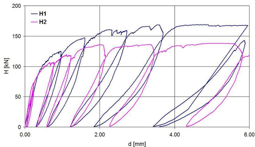
**Figure 7.** Relationships between lateral load and displacement of specimens H1 and H2
