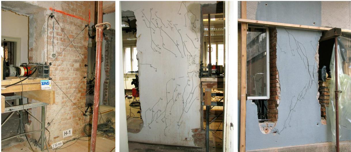
**Figure 6.** Arrangement of hydraulic jack and instrumentation of specimen H1 (left) and typical crack pattern at maximum resistance on the rear surface of specimen H1 (middle) and specimen H2 (right)
