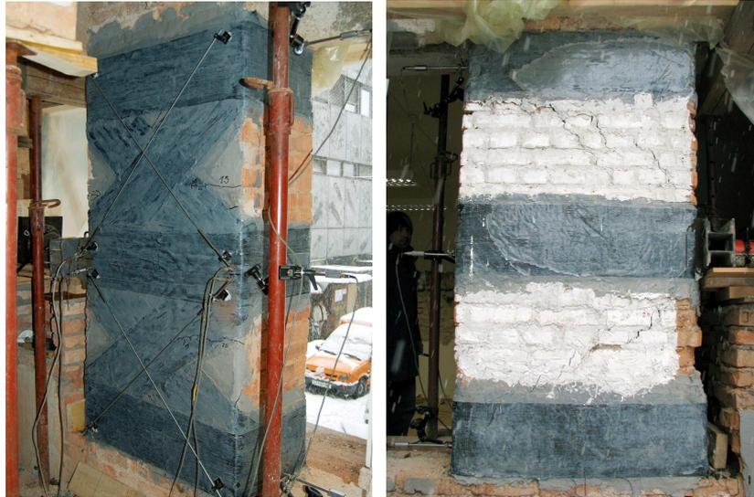
**Figure 10.** Specimen H2w: distribution of cracks on the inner surface (left) and on the outer surface (right)
