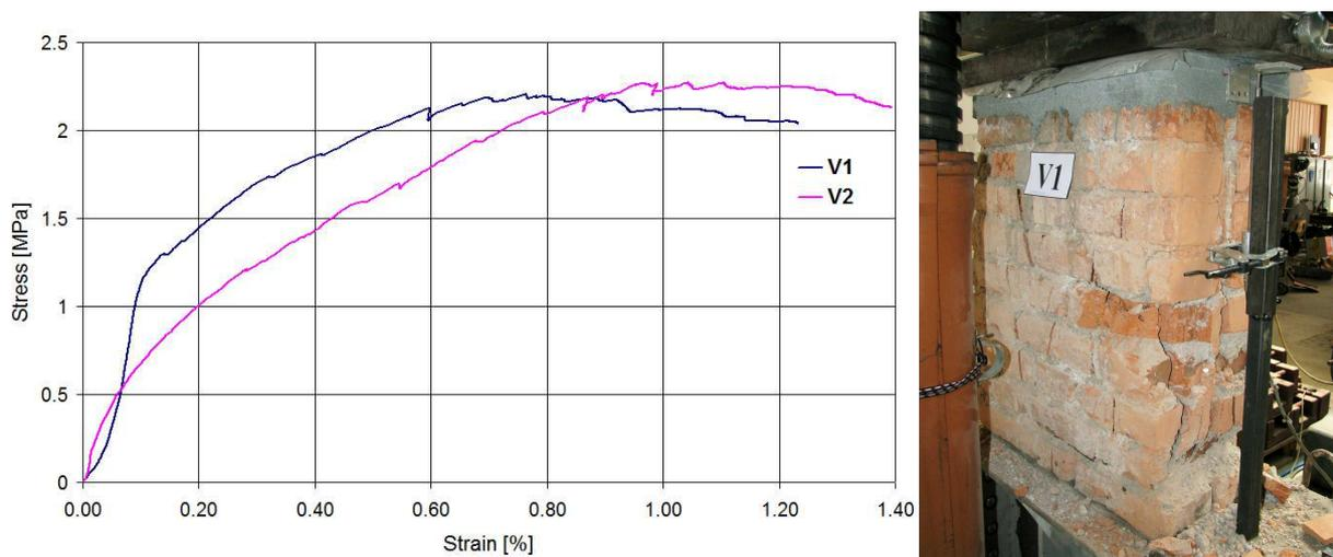
**Figure 3.** Relationship between the vertical load and strain of specimens during compression tests (left) and typical compression failure mode of specimen V1 (right)
