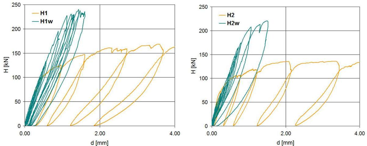
**Figure 11.** The influence of strengthening of specimens on the relationships between lateral load and displacement
