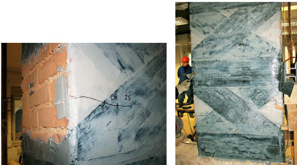
**Figure 9.** Specimen H1w: the development of first cracks (left) and the final stage of the test (right)
