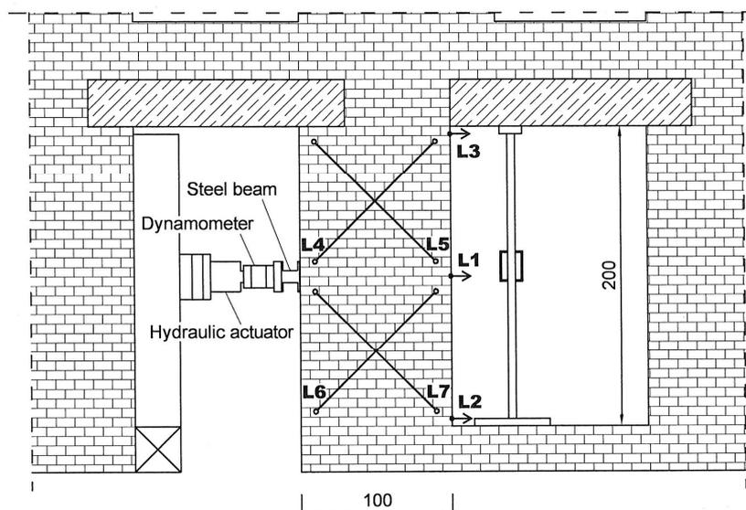
**Figure 5.** In-situ lateral resistance testing set-up
