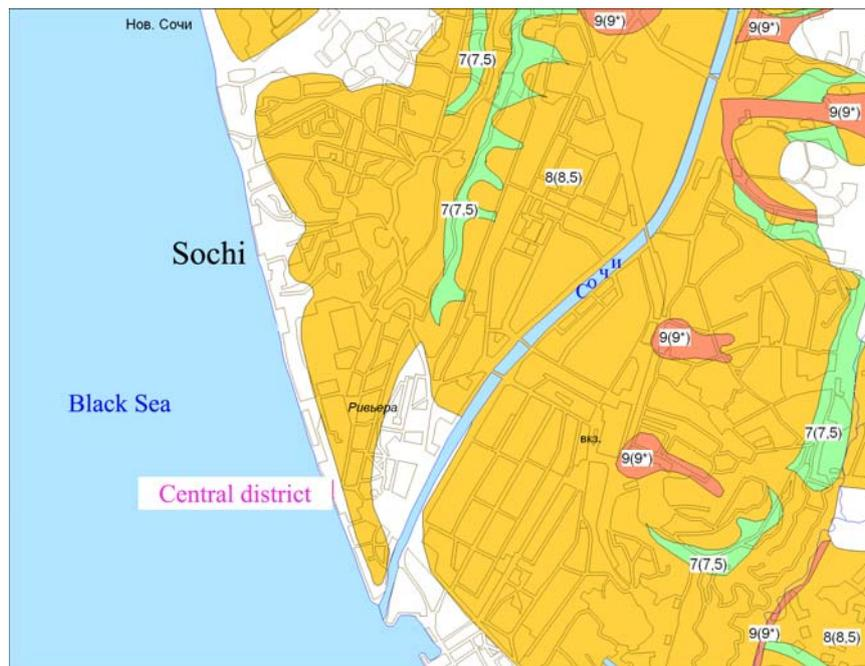
**Figure 2.2.** Fragment of the seismic microzonation map for the Big Sochi territory: figures on map correspond to different level of background seismicity for T=500 years and in brackets for T=1000 years
