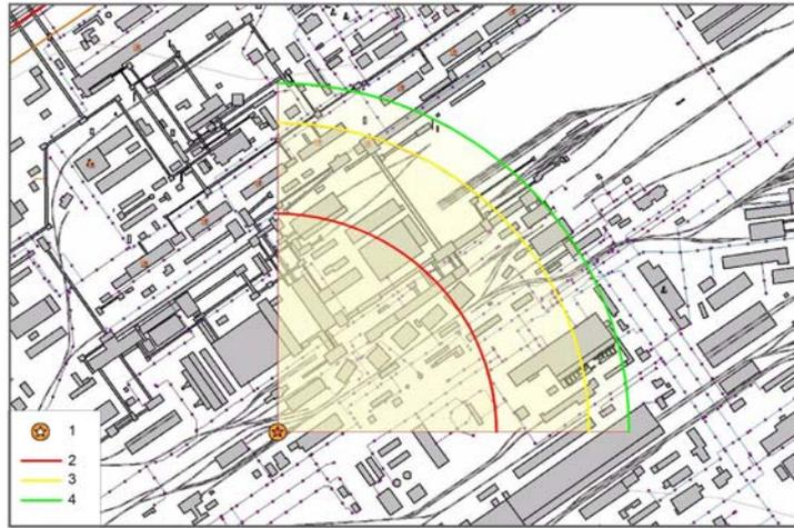
**Figure 5.7.** Simulation of possible contaminated zones in the case of an accident with chemical material release: 1 –source of release of 0.3 tons liquid chlorine; 2 – after 1 hrs; 3 – after 3 hrs and 4 – after 4 hrs.
