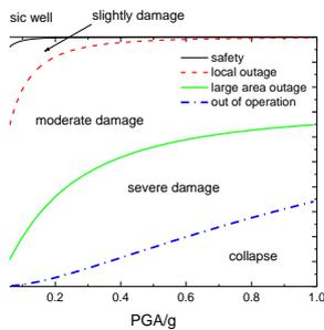
Figure 4. Seismic Vulnerability Curves
