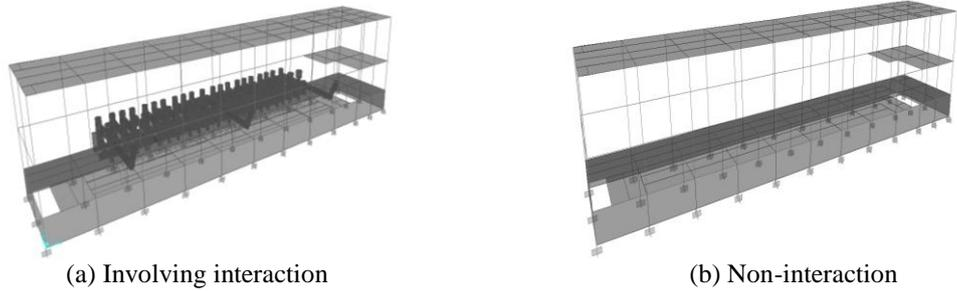
Figure 1. Finite element model of substation
