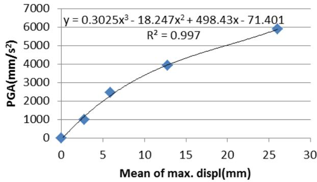
Figure 2.5. Mean of maximum displacements of the reference structure
