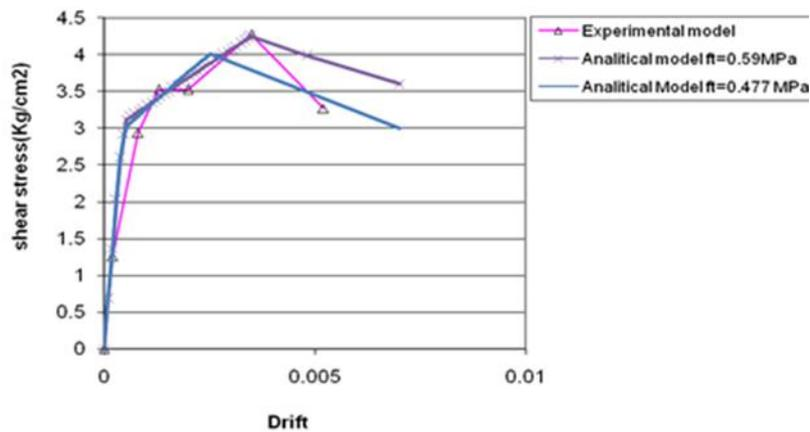
**Figure 1.2.** Comparison of capacity curves obtained by experimental and numerical model (Ranjbaran et al. 2012)
