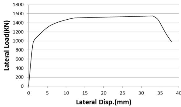
Figure 2.6.A Sample of the capacity curve of the reference structure
