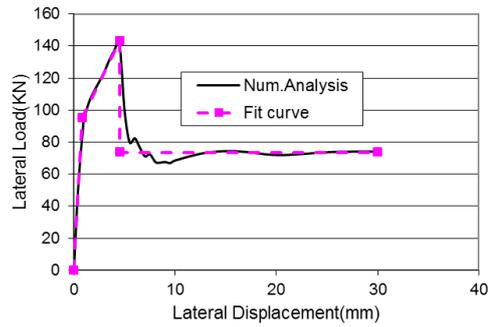
**Figure 1.1.** A sample of the lateral force-displacement curves of confined masonry walls (Ranjbaran et al. 2012)
