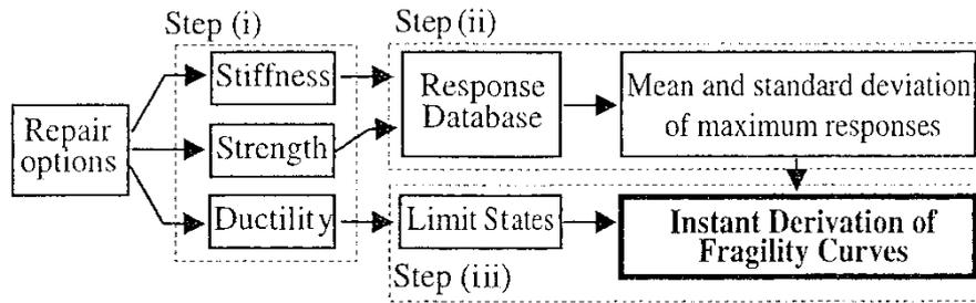
**Figure 2.1.** Overall procedure of the parameterized fragility curves (Jeong and Elnashai, 2007)
