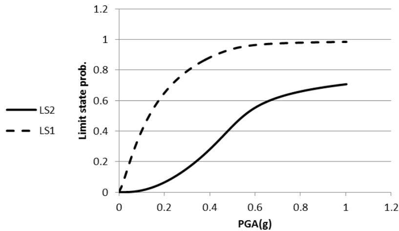
Figure 2.7. Fragility curves (LS1=Elastic limit strength, LS2=Maximum strength)
