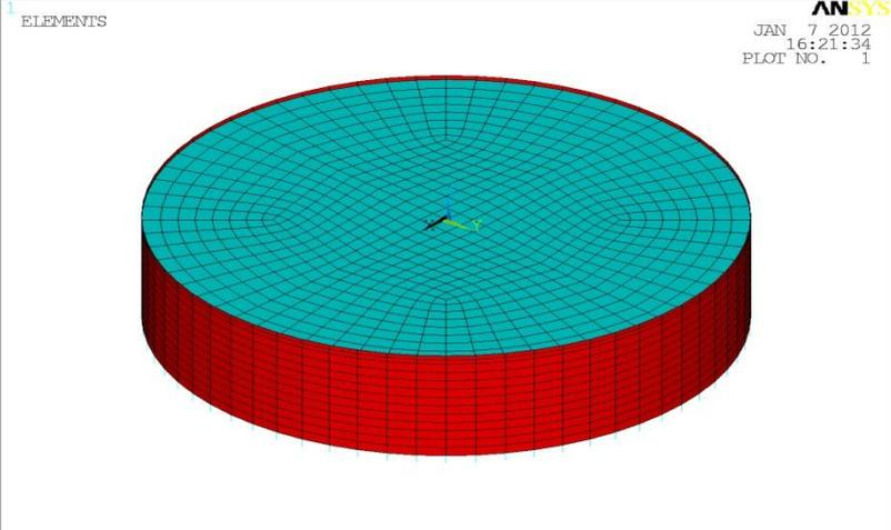
Figure 2. Used FEM model of the tank TK3001 in analysis
