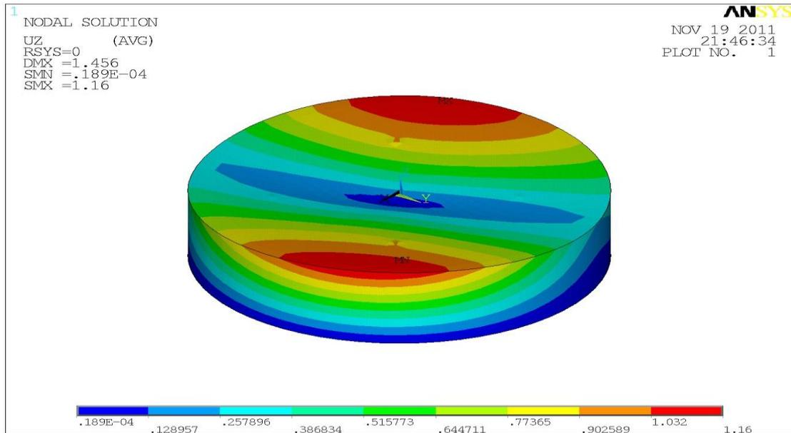
Figure 4. Maximum fluid wave height in tank TK3001 due to spectral analysis
