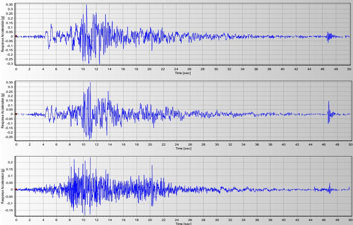
Figure 3. Horizontal(L,T) and Vertical (V) components of Tabas earthquake acceleration record
