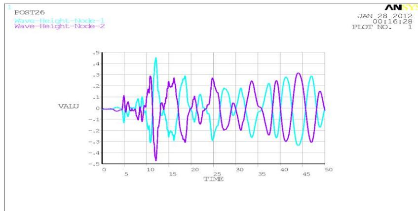
Figure 5. Maximum sloshing wave of liquid affected to Tabas record
