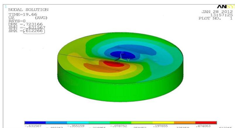
Figure 7. Maximum sloshing wave height in TK3001 tank due to Tabas record
