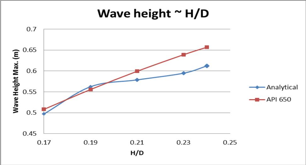
Figure 8. Diagram of sloshing wave height with respect to H/D ratio ( Analytical and API650 values)
