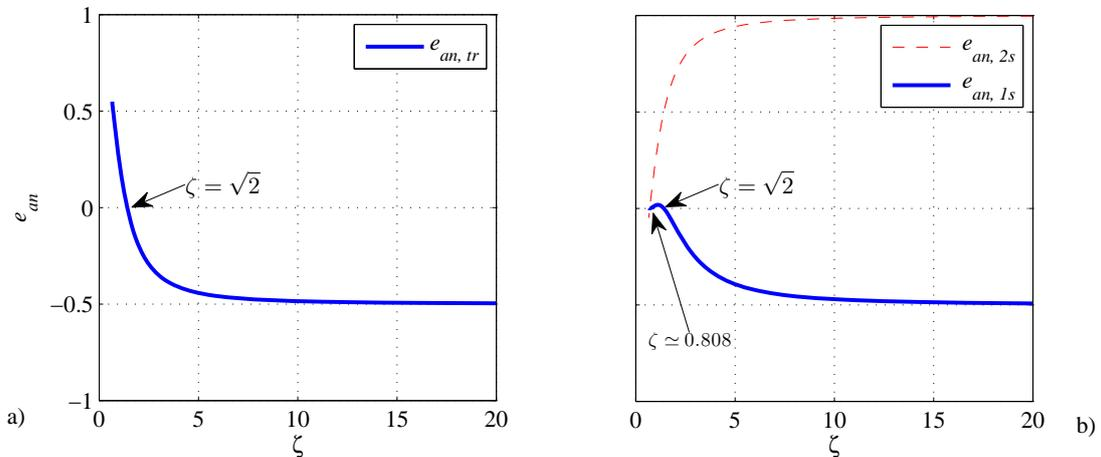
Figure 2. Coefficients of restitution as function of  $\zeta$  = height-to-thickness ratio of the wall. a)  $e_{an,tr}$ ; b)  $e_{an,1s}$ ,  $e_{an,2s}$ . An homogenous, parallelepiped wall has been assumed.
