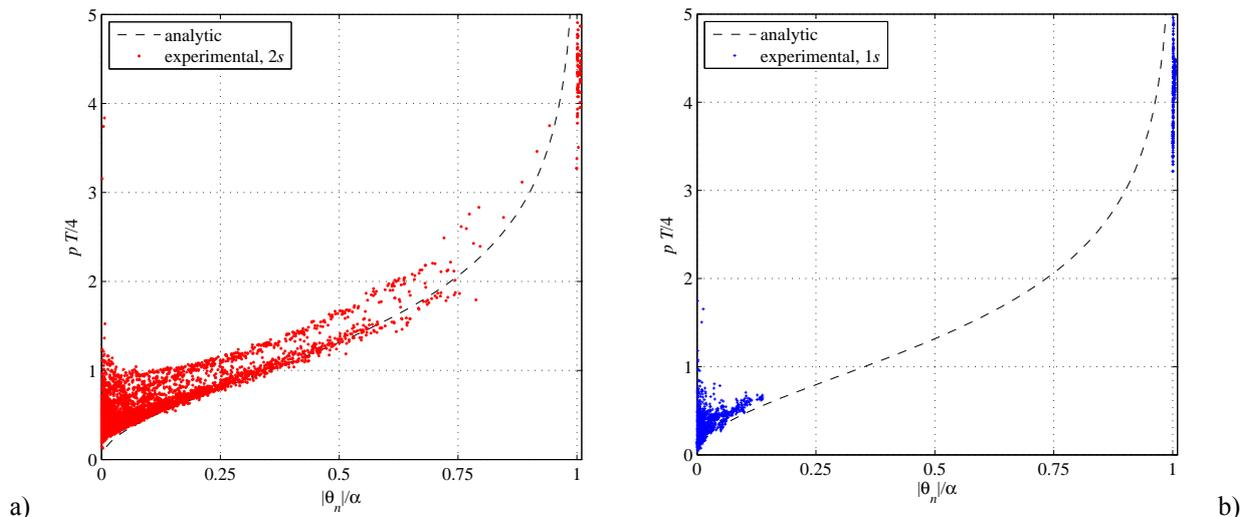
**Figure 5.** Non-dimensional period of the wall,  $T$ , multiplied by the frequency parameter  $p = \sqrt{m g R / I_0}$ . Comparison between experimental data and analytical formulation (Housner 1963).
