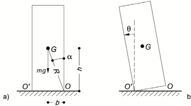
Figure 1. Parapet wall: geometrical parameters and displaced configuration.
