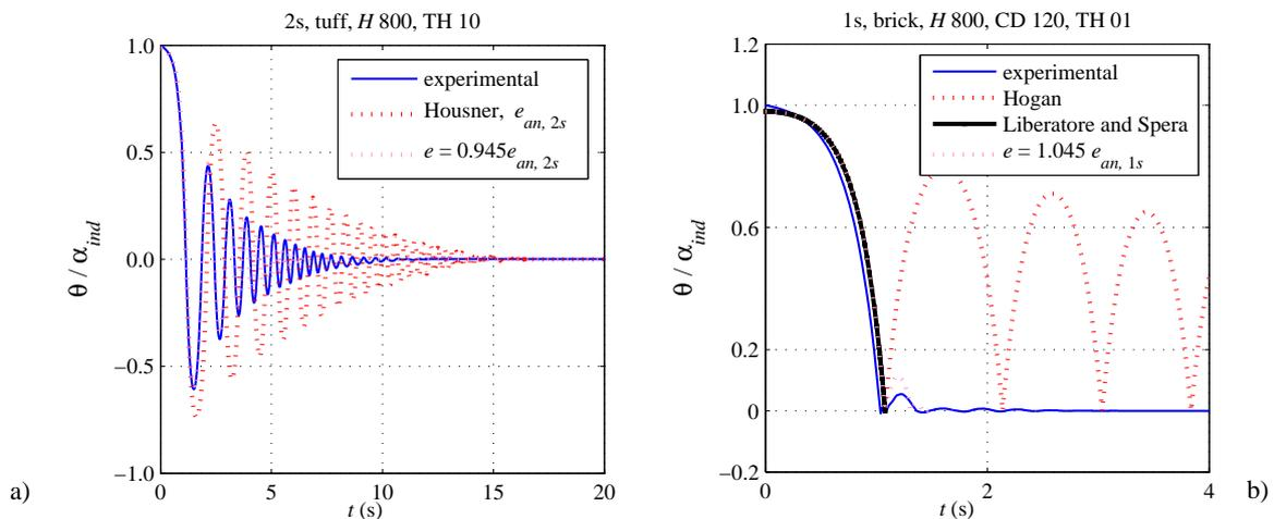
**Figure 4.** Comparison between experimental and analytic time histories. a) Two-sided rocking, b) One-sided rocking. Due to numerical sensitivity issues, all analytic models assume  $\theta_0 / \alpha = 0.985$
