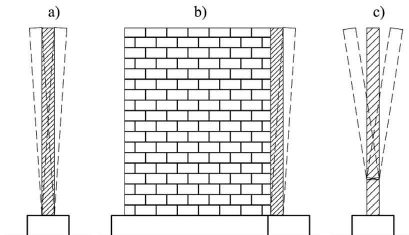
**Figure 3.** a) Two-sided rocking, b) one-sided rocking, c) wall fractured above the base in order to get a different height-to-thickness ratio
