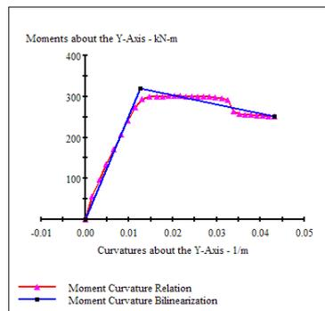
Figure 20. Moment Curvature of retrofitted concrete column.
