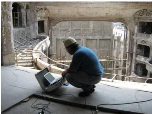
**Figure 16.** Microtremor test of building
