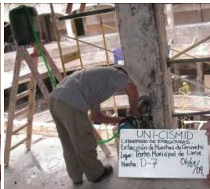
Figure 14. Concrete sample from column of 4<sup>th</sup> floor.
