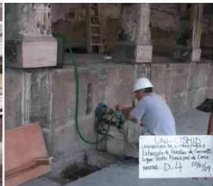
Figure 15. Concrete sample from inverted beam of 4<sup>th</sup> floor.
