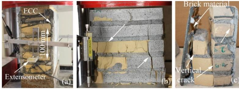
**Figure 2.5.** (a) Test setup, failure mode of the brick prisms: (b) without strengthening layer, (c) with two layers of ECC
