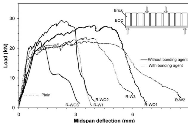
**Figure 2.8.** Flexural response of the masonry beams
