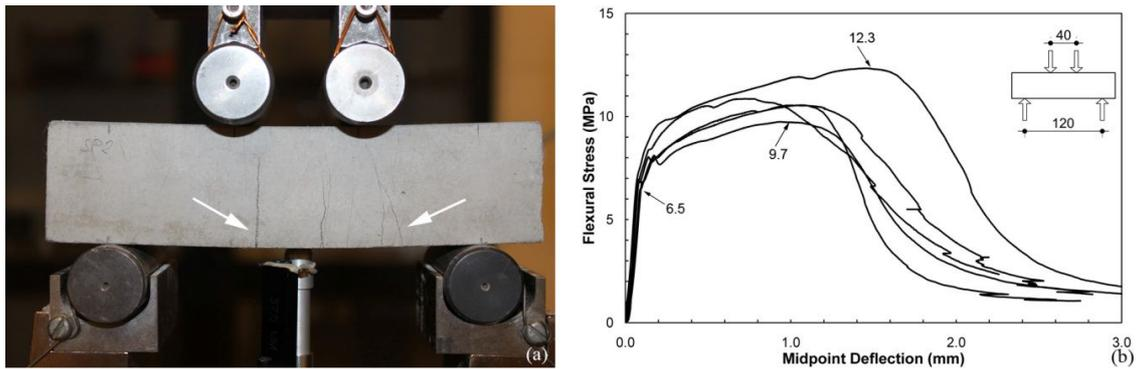
**Figure 2.2.** (a) Four point bending test setup and multiple cracking of ECC (b) ECC flexural Stress-deflection behavior
