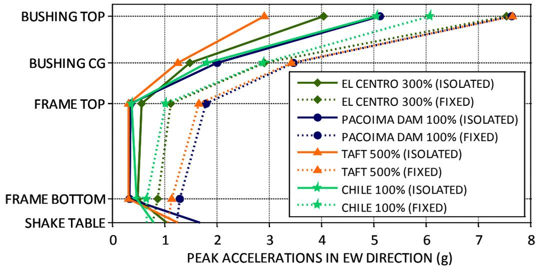
**Figure 10.** Peak Accelerations (EW Direction) for Tri-axial Testing, Reduced Scale Triple FP Isolators and Non-symmetrical Installation of the Bushing
