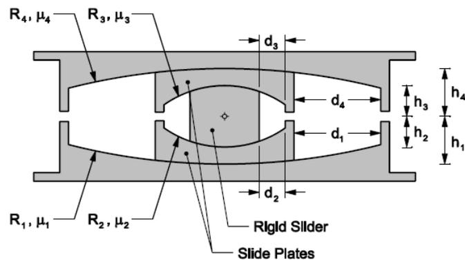
Figure 3. Schematic of Geometrical and Frictional Properties of Triple FP
