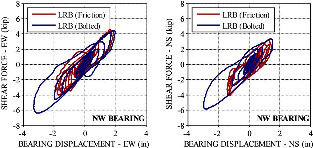
**Figure 9.** Comparison of Force-Displacement Loops in EW and NS Directions for the NW LRB Isolator Bolted and Connected to the Superstructure through Friction (Saratoga at 157% of Original, 2D Horizontal Excitation)
