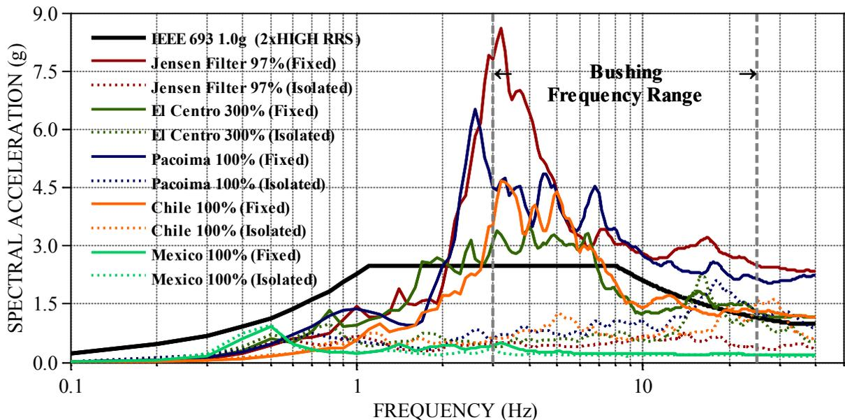
**Figure 5.** Response Spectra (5% Damped) at the Top of the Frame for Fixed and Isolated Conditions
