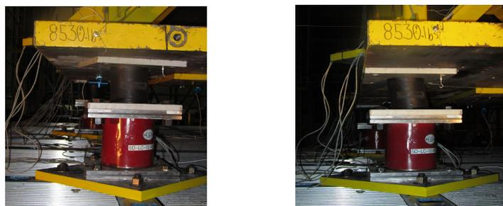
**Figure 8.** Cumulative sliding over the NW LRB isolator
