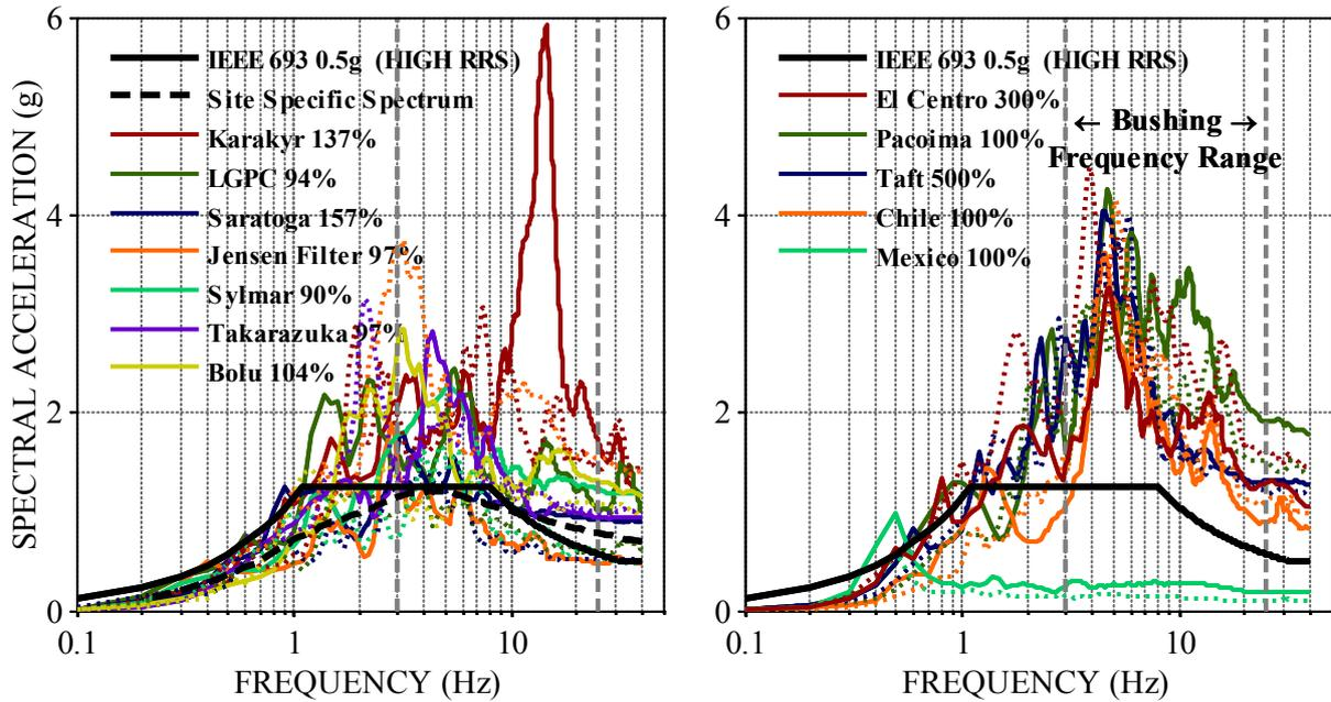
**Figure 4.** Response Spectra of Ground Motions Scaled to Represent the Site Specific Spectrum in an Average Sense (Left) and Historic Ground Motions (Right) as Achieved on the Shake Table (5% Damped)
