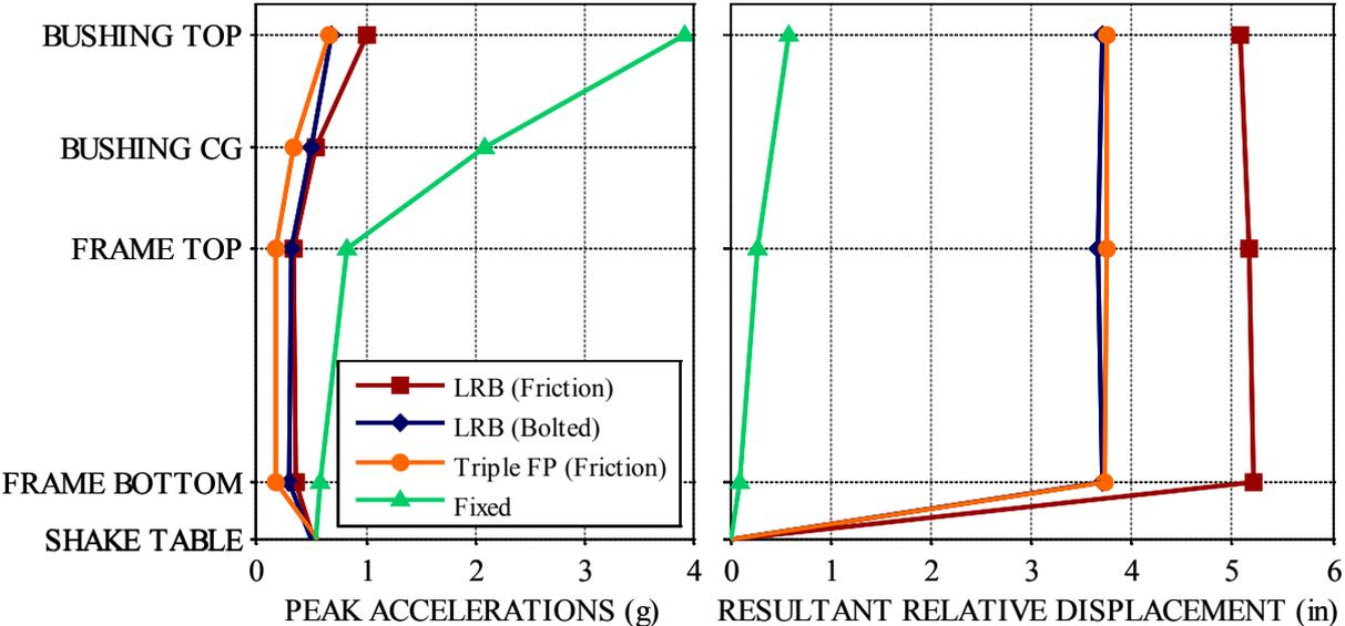
**Figure 6.** Peak Accelerations (NS Direction) and Resultant Displacements for Isolation Systems Tested (Saratoga 157% of Original, 2D Horizontal, Bushing Symmetrically Installed)
