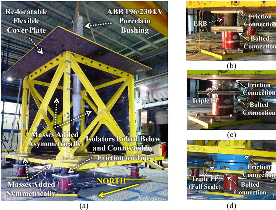
**Figure 2.** Transformer Model with Symmetric Bushing Installation (a) and Seismic Isolation Systems (b, c, d)
