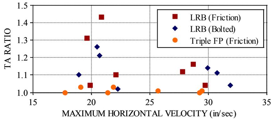
**Figure 7.** TA Ratios for Various Systems Tested Under the Same Motion Ensemble (Reduced Scale Testing)
