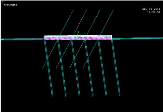
**Figure 5.** The FE model of the box-section beam with axial link supports
