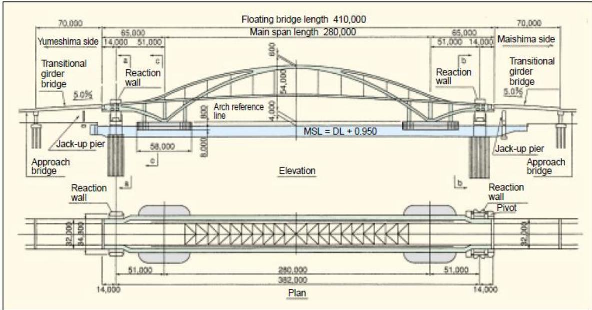
**Figure 3.** Geometric features of the floating bridge considered in this study
