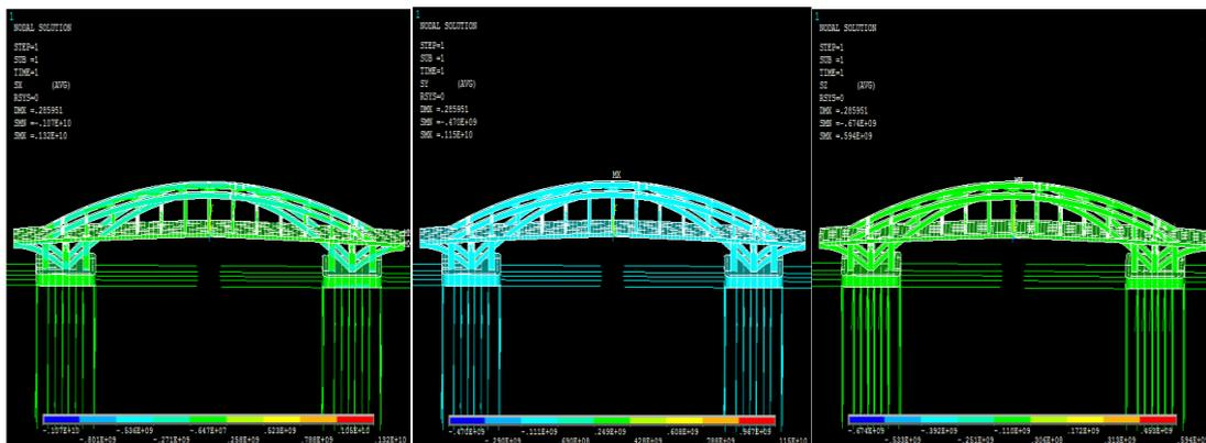
**Figure 7.** Stress values in the bridge body subjected to Chi-Chi earthquake
