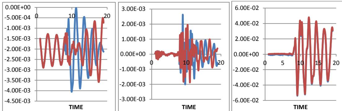
**Figure 6.** Displacement values of the center point of the deck to the arch on both sides of the bridge subjected to Chi-Chi earthquake
