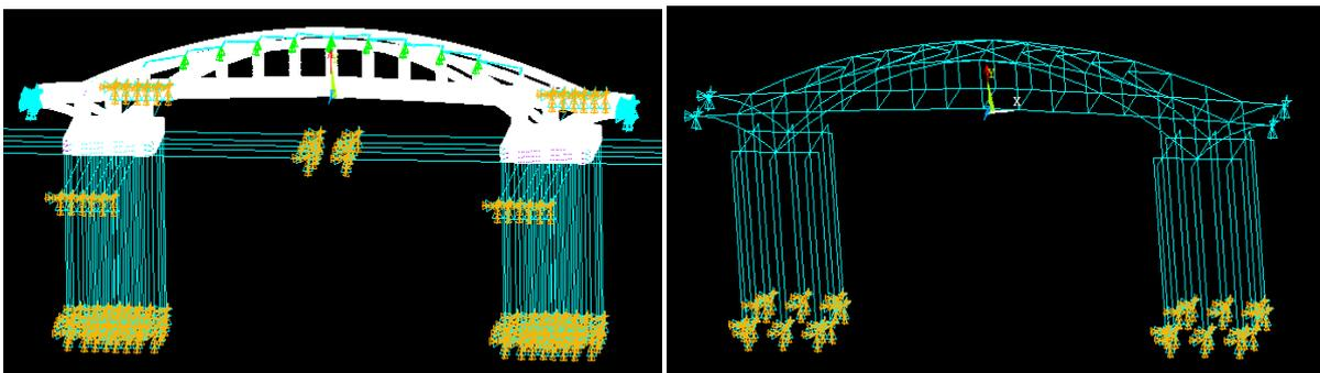
**Figure 4.** The original (left) and the simplified (right) model of the bridge-water system
