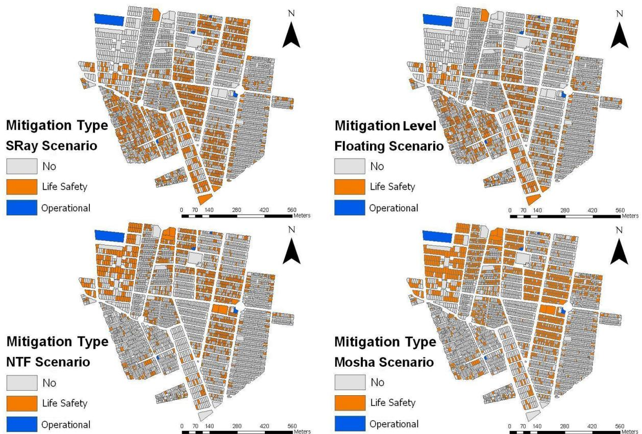
**Figure 2:** Distribution of mitigation alternative in the pilot area for South Ray Fault scenario (2.a Up-left), Floating scenario (2.b Up-right), North Tehran Fault scenario (2.c Bottom-left) and Mosha fault scenario (2.d Bottom-right)
