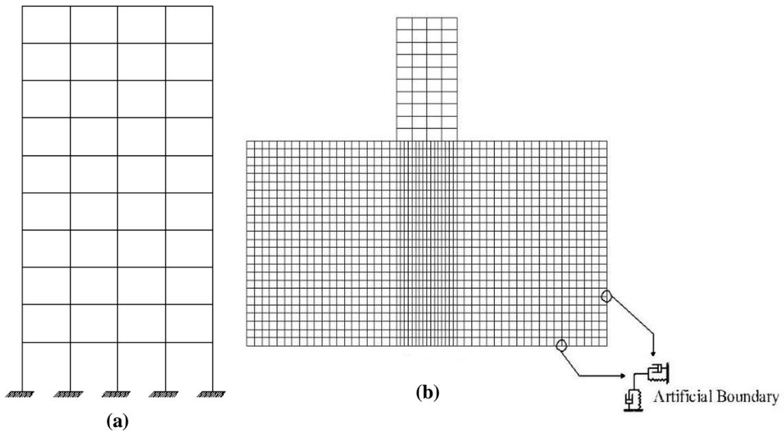
**Figure 1.** Ten-story building models: (a) Fixed foundation; (b) Elastic foundation
