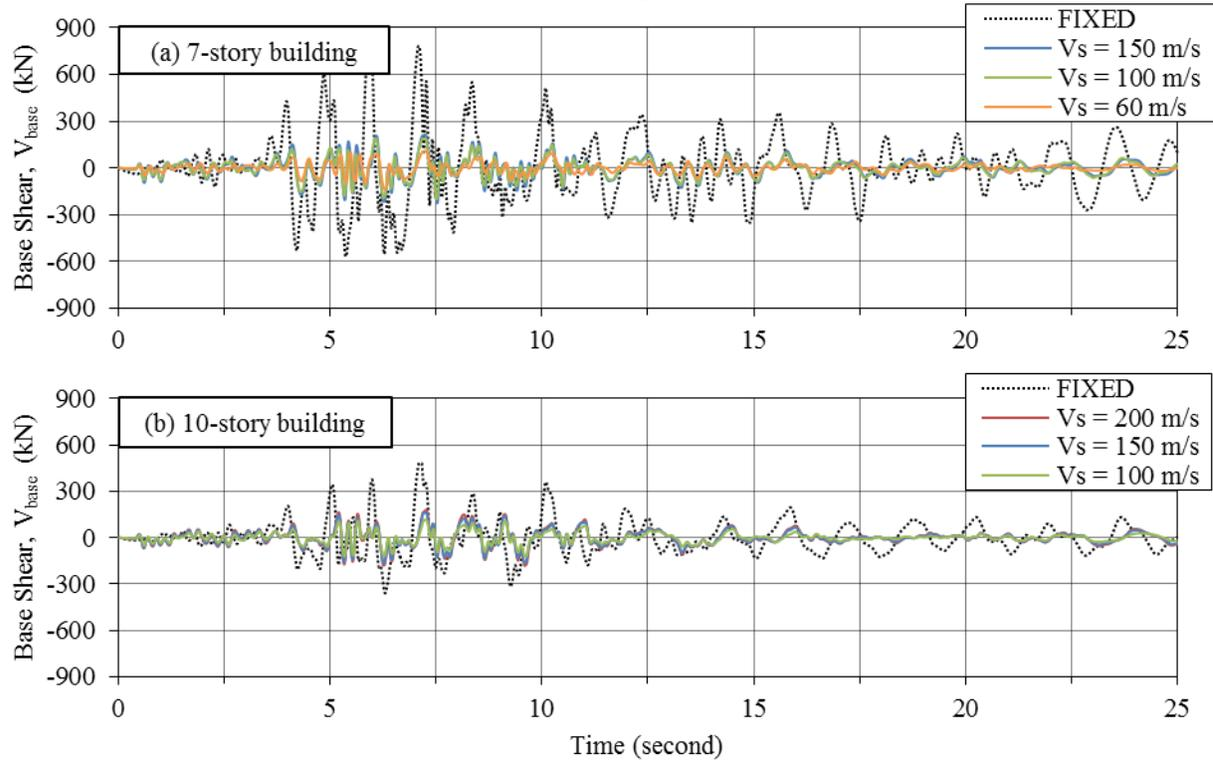
**Figure 8.** Time history of base shear for buildings due to Victoria earthquake (PGA = 0.3g)
