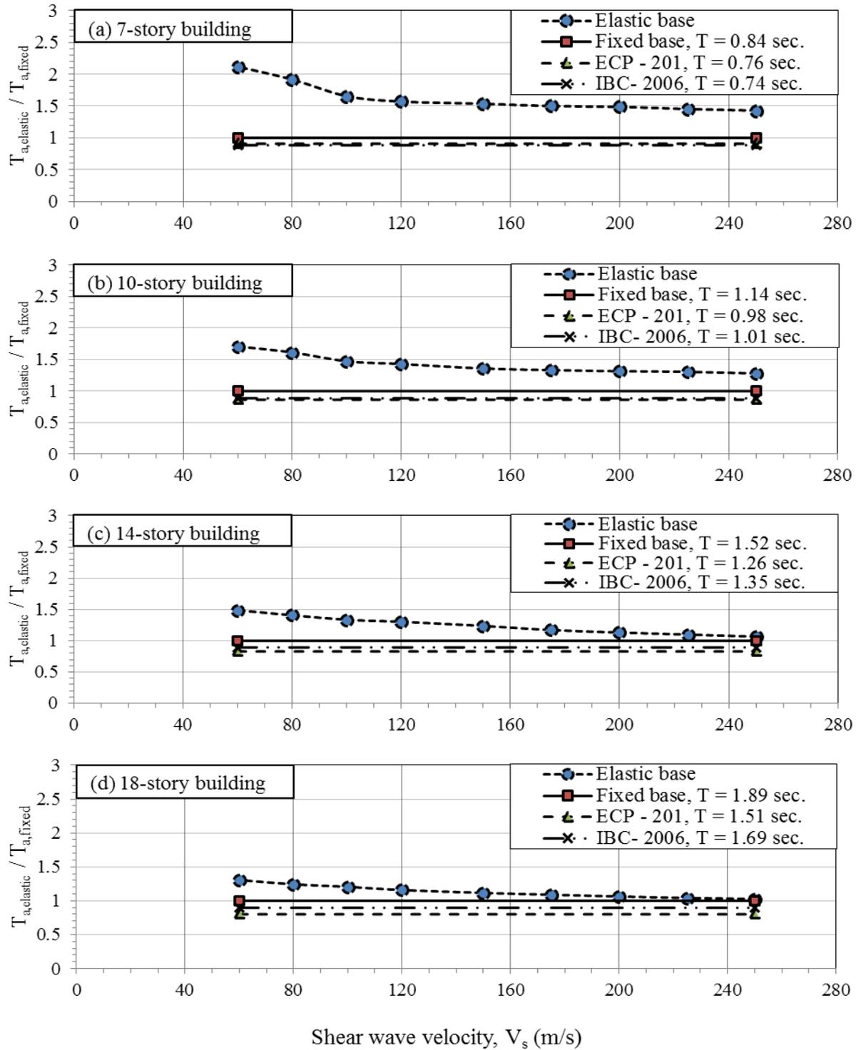
**Figure 3.** Effect of soil shear modulus ( $V_s$ ) on fundamental period of buildings with variable heights: a) 7-story; b) 10-story; c) 14-story; d) 18-story
