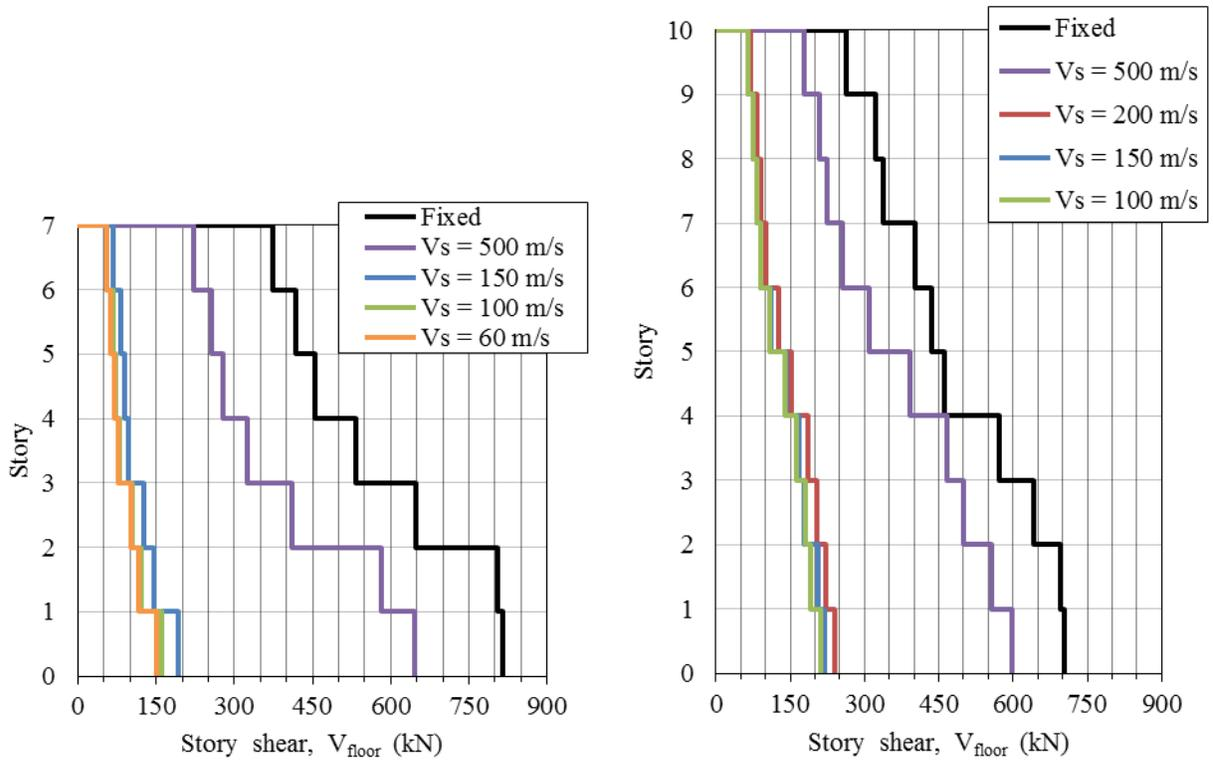
**Figure 5.** Maximum story shear for buildings due to Kobe earthquake (PGA = 0.3g)
