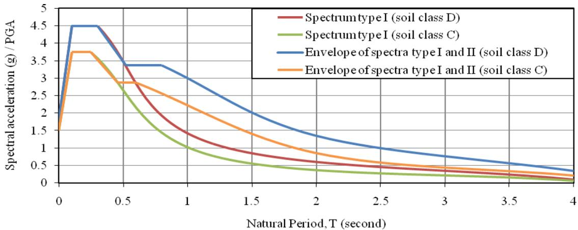
**Figure 4.** Response spectra types I and II for soil classes C and D as in ECP-201
