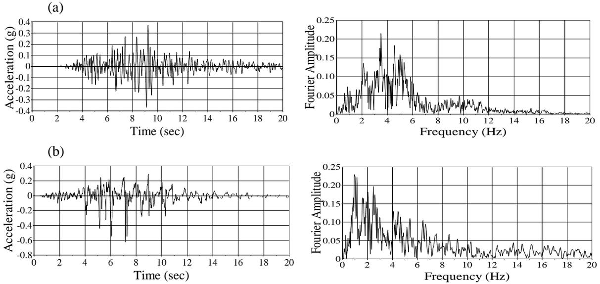
**Figure 2.** Acceleration time histories and corresponding Fourier amplitude spectra of the applied ground motions: (a) Kobe; (b) Victoria
