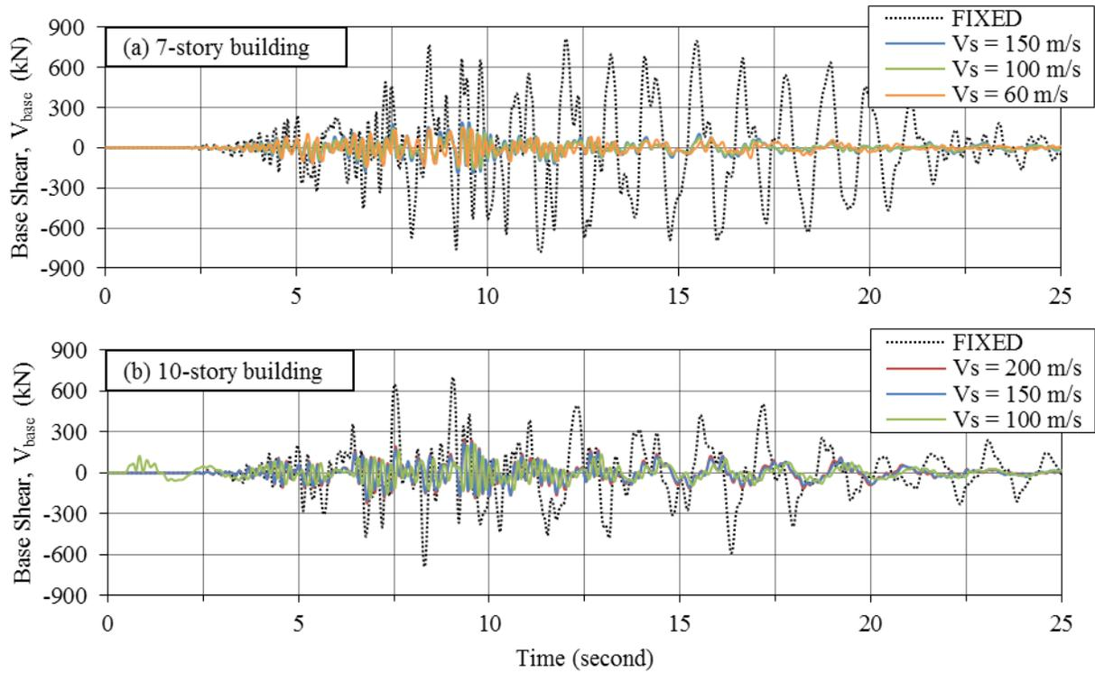
**Figure 7.** Time history of base shear for buildings due to Kobe earthquake (PGA = 0.3g)
