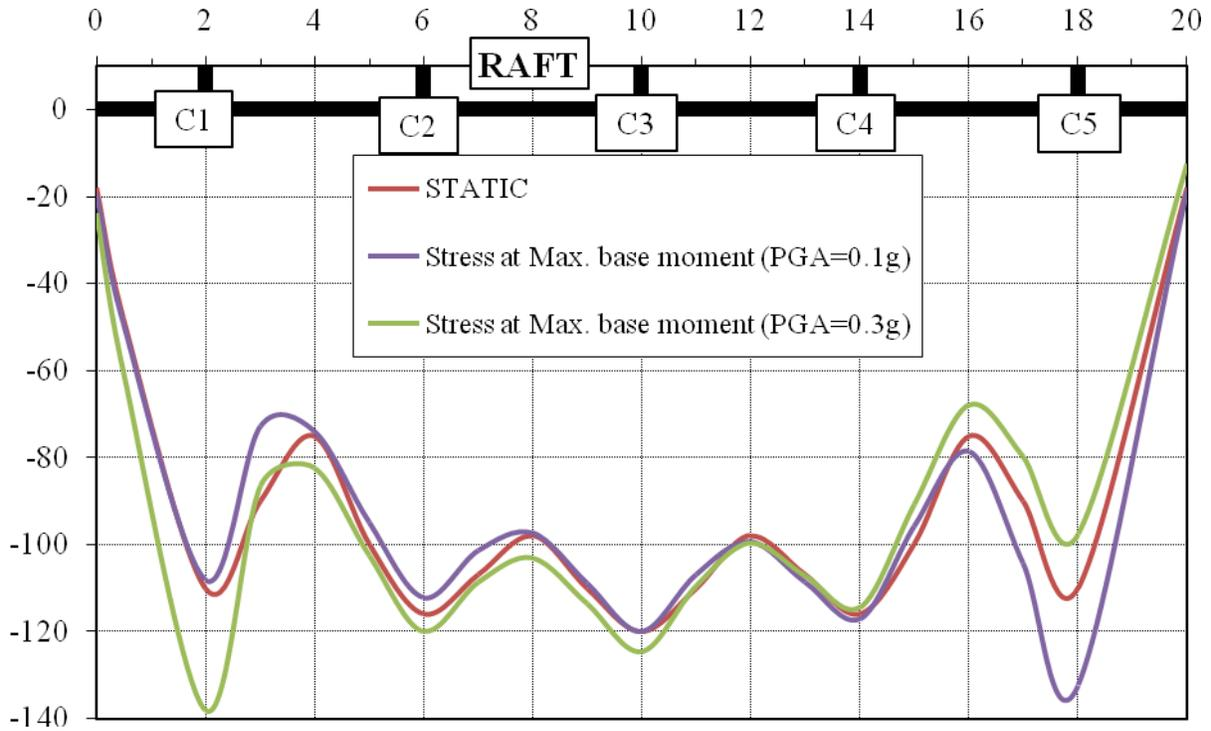
**Figure 9.** Distribution of contact stresses (kPa) for the 10-story building due to different load cases- Kobe earthquake ( $V_s=150$  m/sec)
