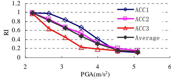
**Figure 4.3.** Repairability index curve of the building
