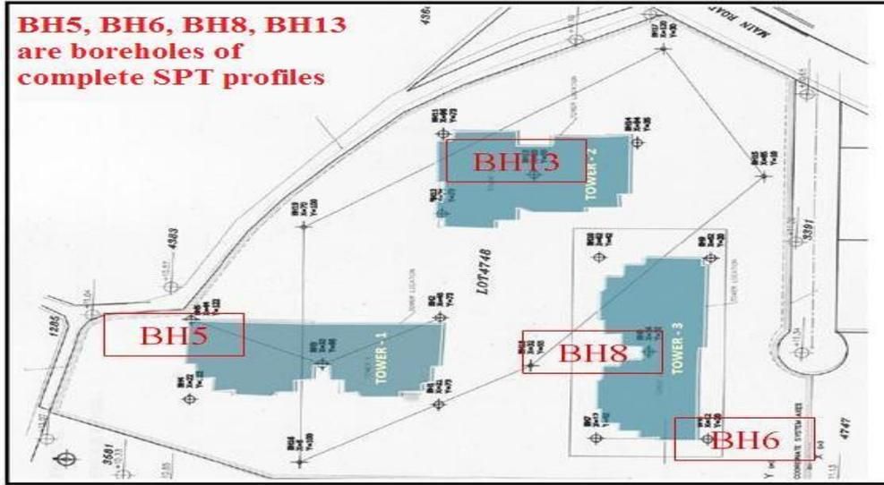
**Figure2.** Boreholes from which complete SPT profiles are obtained
