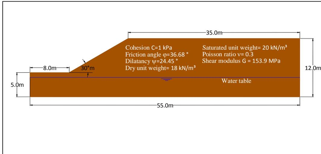
**Figure6.** Slope geometry, soil properties and site conditions (water table at 8 m below NGL)
