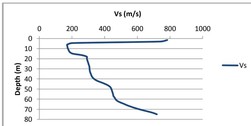
**Figure4.** Shear wave velocity profile from ambient noise test
