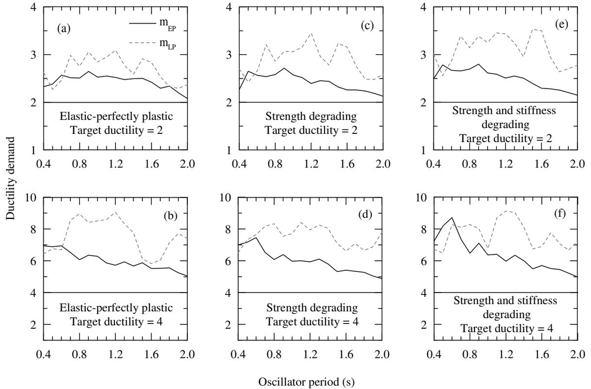
**Figure 5.1:** Mean ductility demand versus oscillator period for the early arriving pulse ( $m_{EP}$ ) and the late arriving pulse ( $m_{LP}$ ) motions for (a, b) elastic-perfectly plastic oscillators, (c, d) strength degrading oscillators, and (e, f) strength and stiffness degrading oscillators for target ductility 2 and 4.
