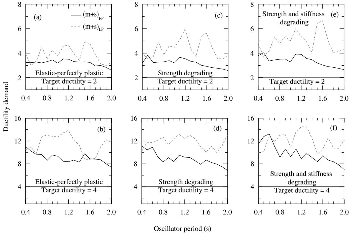
**Figure 5.2:** Mean plus one standard deviation ductility demand versus oscillator period for the early arriving pulse  $(m+s)_{EP}$  and the late arriving pulse  $(m+s)_{LP}$  motions for (a, b) elastic-perfectly plastic oscillators, (c, d) strength degrading oscillators, and (e, f) strength and stiffness degrading oscillators for target ductility 2 and 4.
