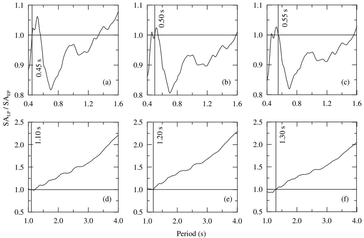
**Figure 5.4:** Ratio of mean acceleration spectrum of the late arriving pulse motions ( $SA_{LP}$ ) to mean acceleration spectrum of the early arriving pulse motions ( $SA_{EP}$ ) versus period for motions (a) scaled at 0.45 s, (b) scaled at 0.50 s, (c) scaled at 0.55 s, (d) scaled at 1.10 s, (e) scaled at 1.20 s, and (f) scaled at 1.30 s.
