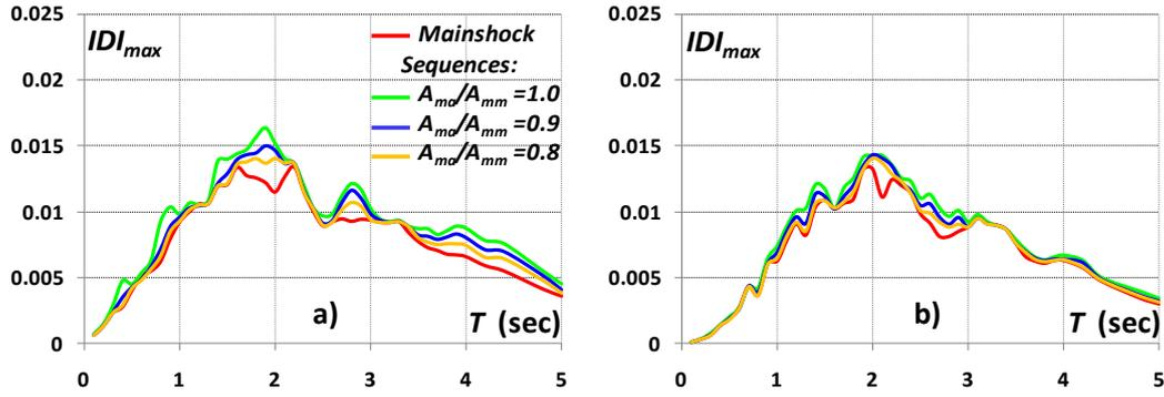
**Figure 3.3.**  $IDI_{max}$  demands for systems subjected to seismic sequences,  $T_{mm}/T_{ma} = 0.9$ ,  $\beta = 0.10$ ,  $\mu = 4$ , a) Standard facilities, b) Essential facilities
