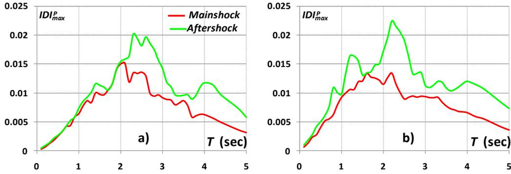
**Figure 3.5.**  $IDI_{max}^p$  demands for systems subjected to seismic sequences,  $T_{ma}/T_{mm} = 1.2$ ,  $A_{ma}/A_{mm} = 1.0$ ,  $\beta = 0.10$ , Standard facilities, a)  $\mu = 2$ , b)  $\mu = 4$
