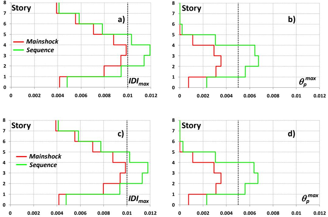
**Figure 4.2.** Maximum deformation demands along height for building under consideration:
