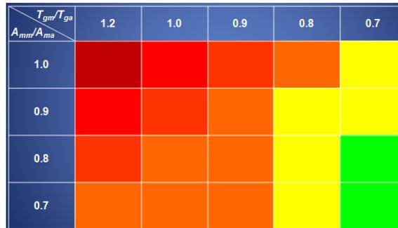
**Figure 3.6.** Color diagram representing influence of parameters  $T_{mm}/T_{ma}$  and  $A_{mm}/A_{ma}$  on response of systems studied herein when subjected to seismic sequences
