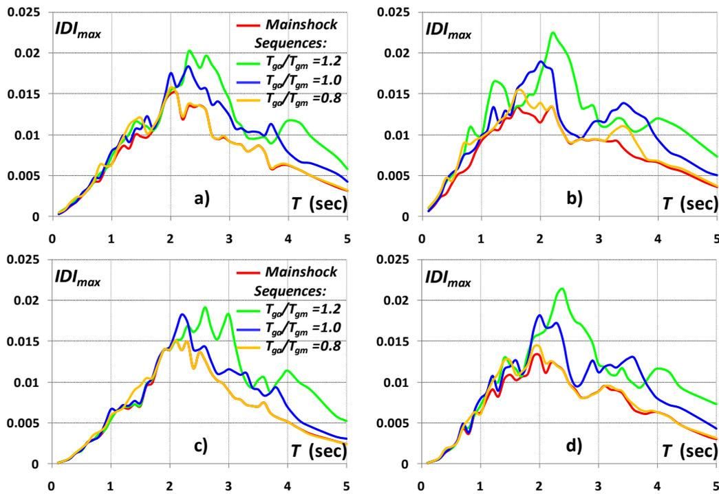
**Figure 3.2.**  $IDI_{max}$  demands for systems (standard group) subjected to artificial seismic sequences with  $A_{nm}/A_{ma} = 1.0$ ,  $\beta = 0.10$ : a) Standard facilities,  $\mu = 2$ , b) Standard facilities,  $\mu = 4$ , c) Essential facilities,  $\mu = 2$ , d) Essential,  $\mu = 4$
