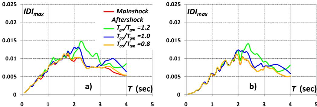
**Figure 3.4.**  $IDI_{max}$  demands for systems subjected to seismic sequences,  $A_{mm}/A_{ma} = 0.8$ ,  $\beta = 0.08$ ,  $\mu = 4$ , a) Standard facilities, b) Essential facilities
