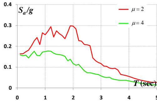
**Figure 3.1.** 5% damped pseudo-acceleration spectra for mainshocks recorded in soft soils
