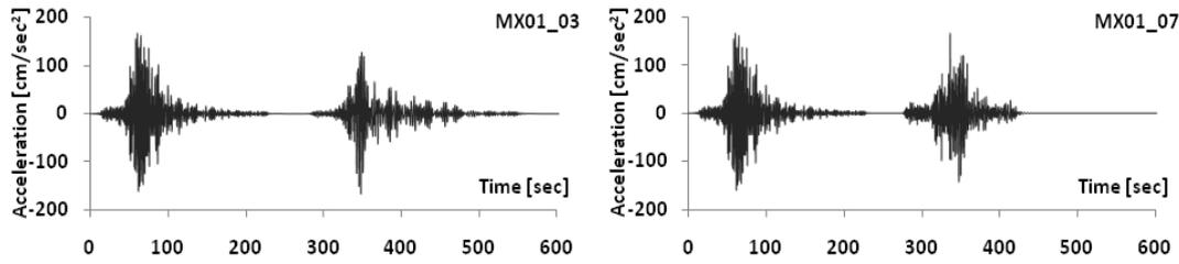
**Figure 2.1.** Artificial seismic sequences used in this study for a specific case of  $A_{ma}/A_{mm} = 1.0$  and  $T_{ma}/T_{mm} = 1.2$
