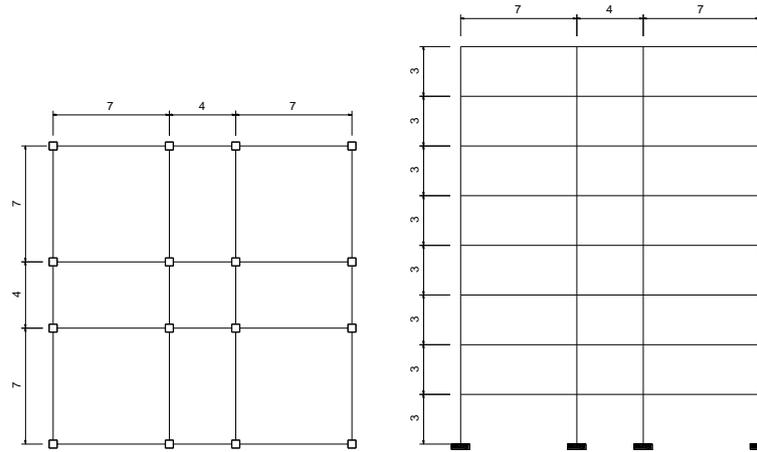
**Figure 4.1.** Plan and elevation view of building under consideration (dimensions in meters)
