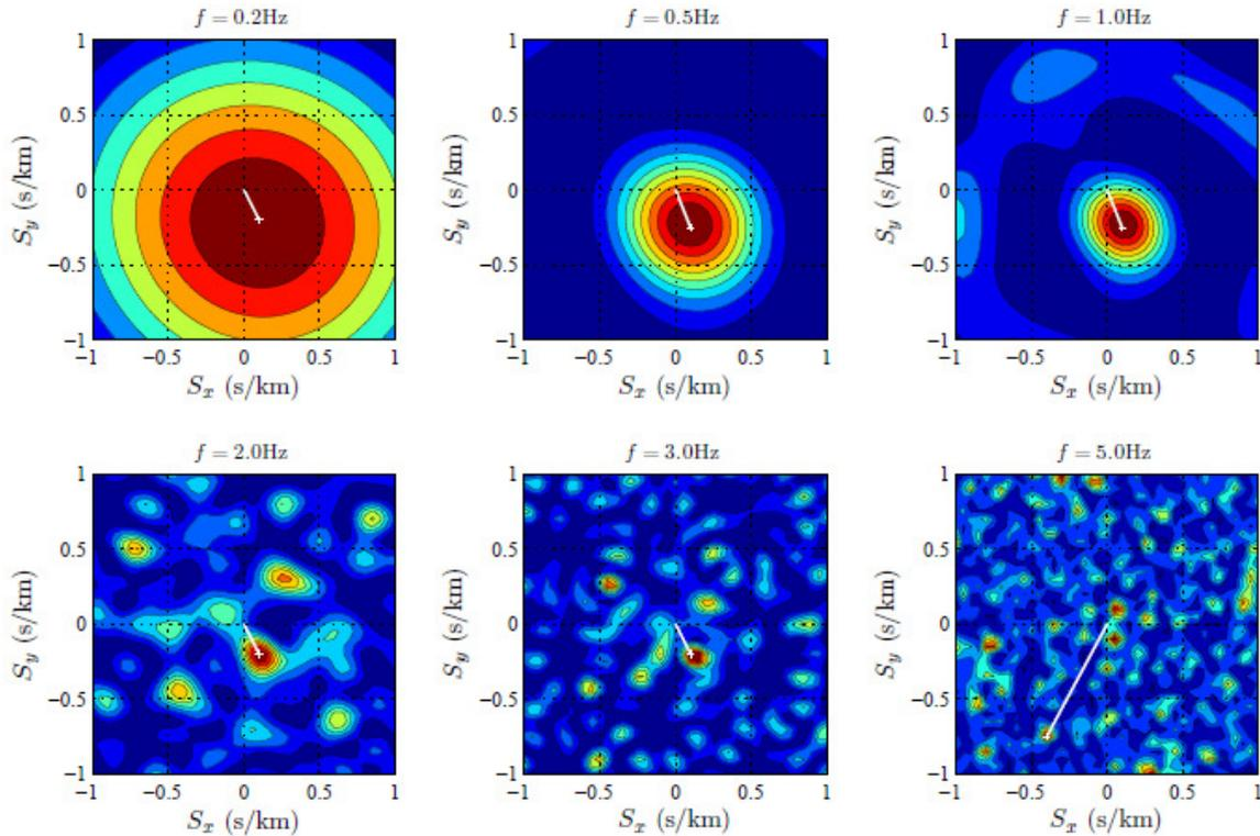
**Figure 2.** Slowness spectra computed from the NS component for 6 different frequencies as indicated in the title of the subplots.  $S_x$  and  $S_y$  indicate slowness in the EW and NS directions respectively. The spectral values from Eqn. 3.2 are normalized by the largest value. The location of peak is marked with a white cross, while the white line indicates the backazimuth direction.
