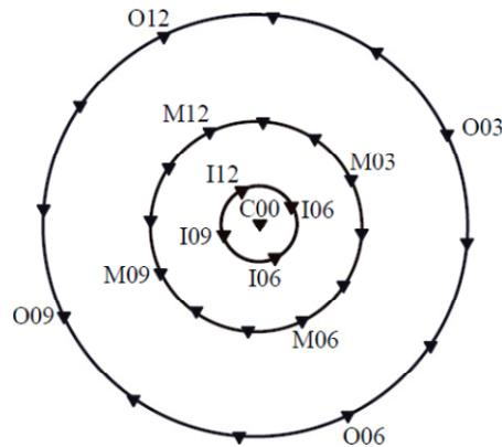
**Figure 1.** Configuration of the SMART 1 array showing the locations of the strong-motion stations (triangles). The central station is called C00; those at the inner ring, middle ring, and outer ring are numbered I01-I12, M01-M12, and O01-O12, respectively. The radii of the rings are 200m, 1km, and 2km.
