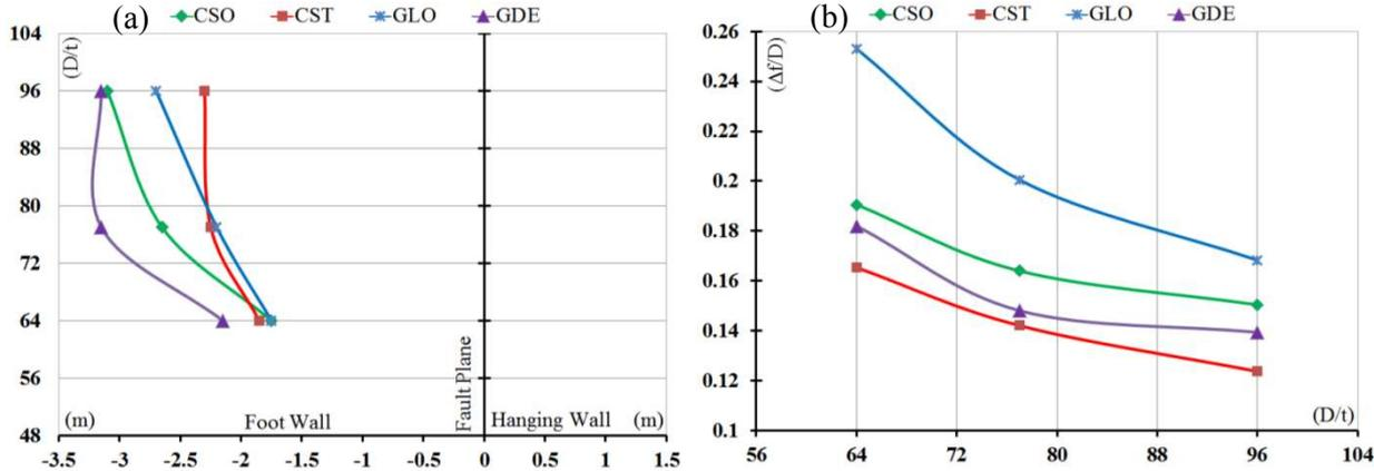
**Figure 2.3.** Influence of the Pipe Wall Thickness on (a) Failure Position of Elements Located at Crown Edge of Pipeline (b) Failure Fault Plane displacement to Diameter Ratio ( $\Delta f/D$ ) With Respect to  $D/t$ . ( $\alpha=45^\circ$ )
