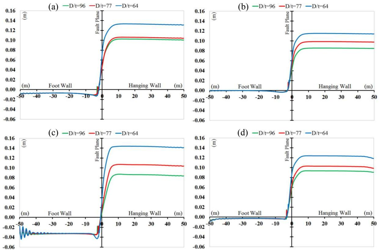
**Figure 2.1.** Influence of Pipe Wall Thickness on Failure Displacement of Pipelines in ( $y$ ) Direction, Buried in: (a) Soil CSO (b) Soil CST (c) Soil GLO (d) Soil GDE ( $\alpha=45^\circ$ , Crown Edge of Pipelines)
