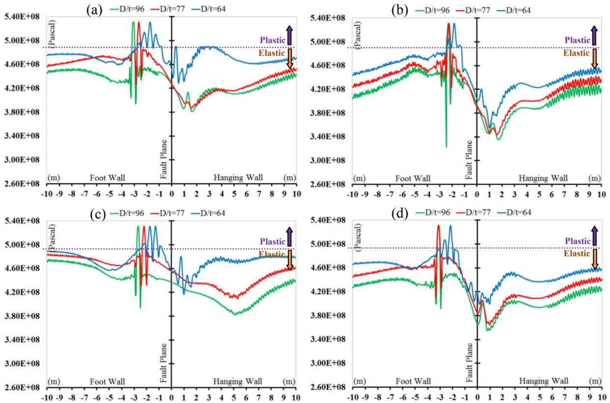
**Figure 2.2.** Influence of the Pipe Wall Thickness on Stress Response of Pipelines, Buried in: (a) Soil CSO (b) Soil CST (c) Soil GLO (d) Soil GDE ( $\alpha=45^\circ$ , Crown Edge of Pipelines)
