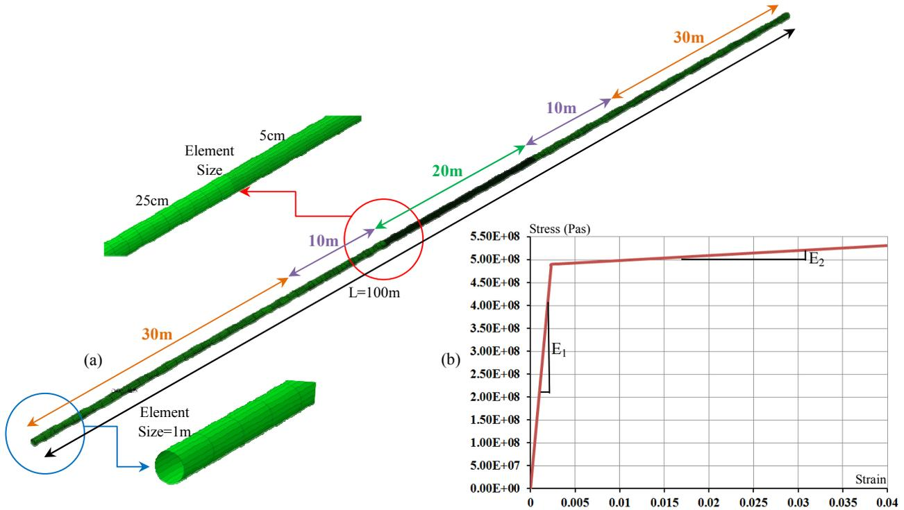
**Figure 1.1.** (a) 3D Finite Element Model of the Pipeline. (b) Material Properties of API-5L-X65 Steel.
